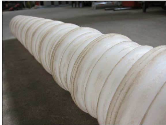
Figure 4-9: Sanded, Plastic Duct
