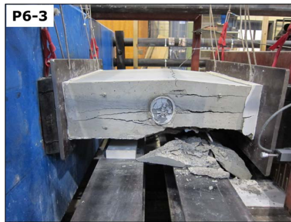
Figure 4-30: Failure of Reinforced Panel with Cracking at Level of Duct
