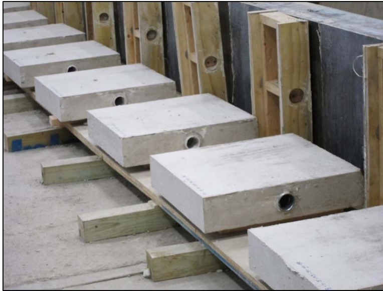
Figure 3-10: Completed Panel Set Cured and Removed from Forms
