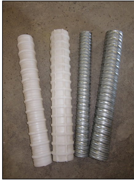
Figure 3-14: HDPE and Steel Ducts
