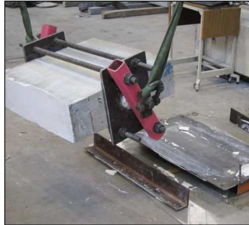
Figure 3-13: End-Capping Panels with Gypsum Hydrostone
