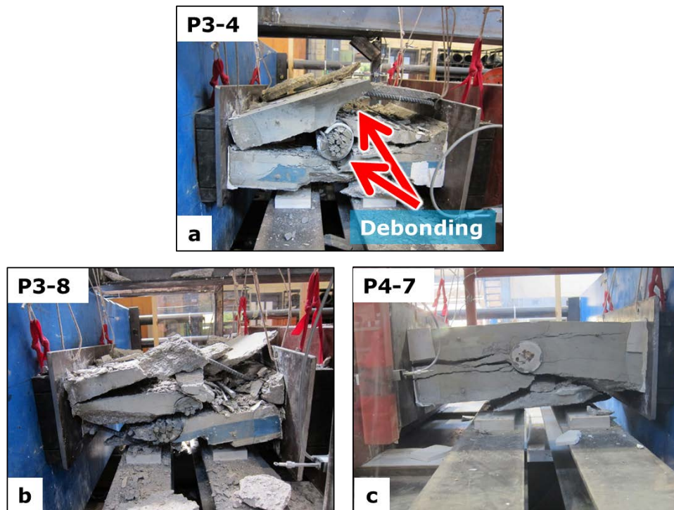
Figure 4-6: Common Failures of Plastic- or Steel-Ducted Panels
