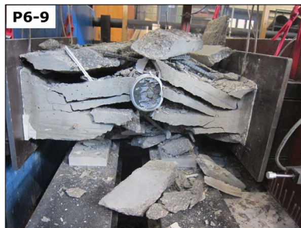
Figure 4-31: Failure of Panel with Reinforcement Near the Duct
