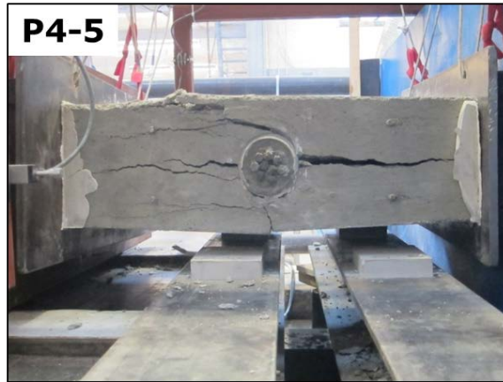
Figure 4-4: Tensile Splitting of Panels
