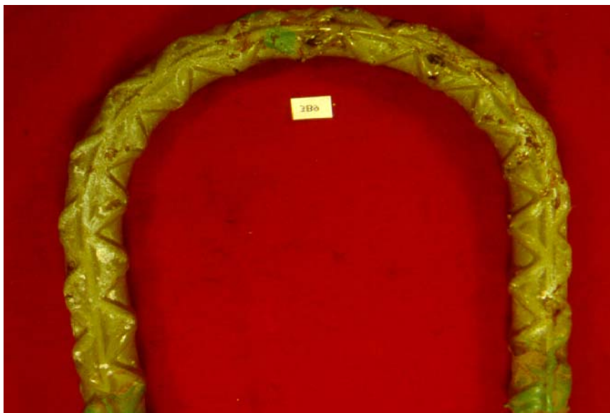
Figure 5.36. Pitting Damage on Epoxy Coated Bent Bar (3B9).
