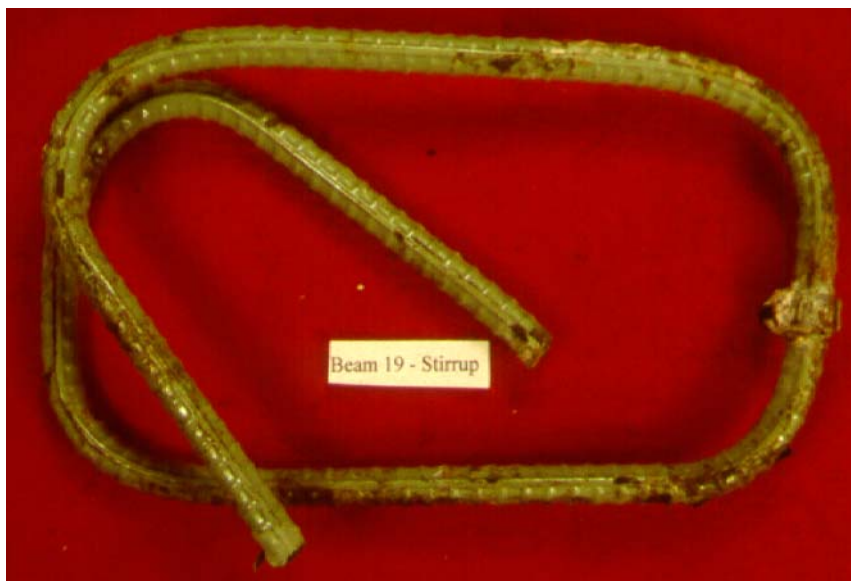
Figure 5.23. Corrosion Damage on Stirrup (Beam19).
