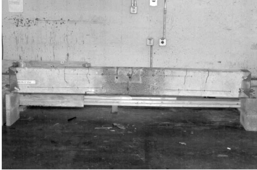
Figure 3.2. Beams Cleaned and Distribution Media Placed at Ends.
