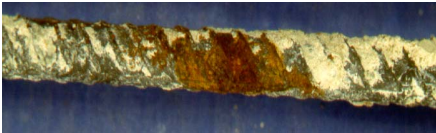
Figure 5.18. Corrosion Outside the Previous Exposed Region (Beam 12).
