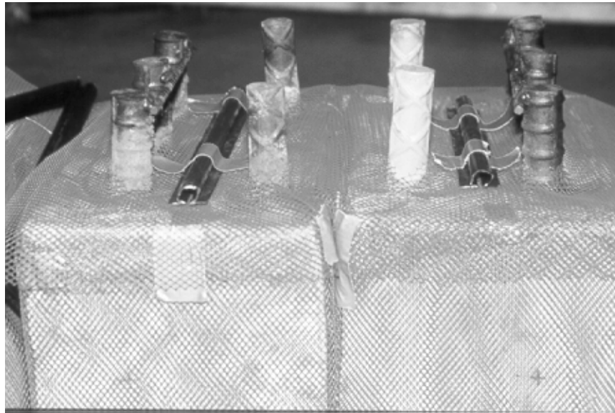
Figure 3.17. Application of Omega Channels as Injection Ports.
