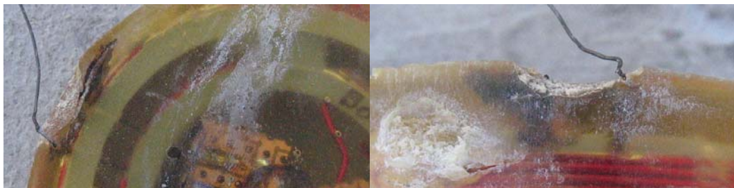
Figure 6-13 Black Corrosion in B04
