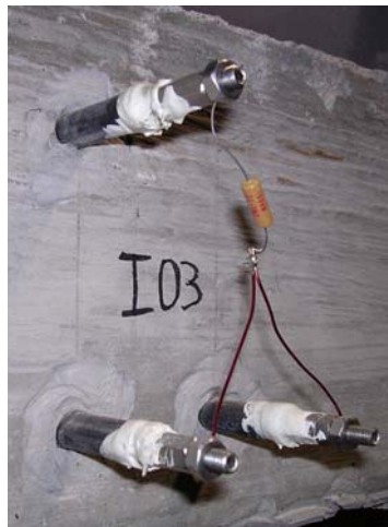
Figure 5-6 Resistor Connecting Top and Bottom Reinforcement
