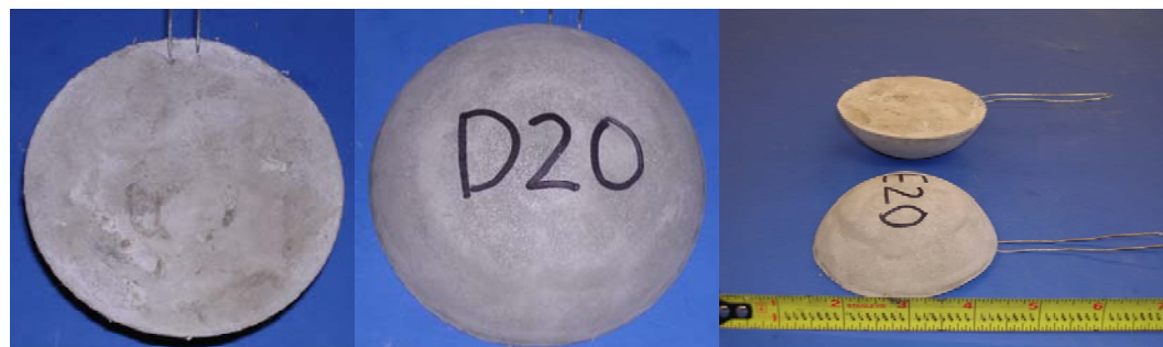
Figure 7-7 Sensor with Fiber-Reinforced Cement Paste Housing
