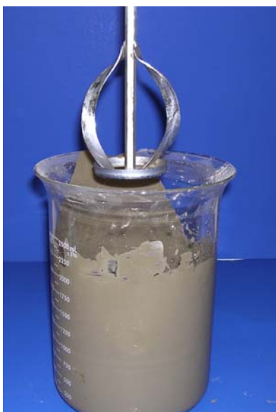
Figure E-2 Mortar Paddle Used to Stir the Mixture
