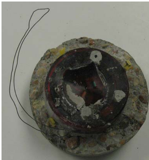
Figure 3-15 Discolorization of Sensor B19
