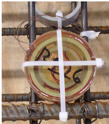
Figure 5-10 Sensing Wire Placed in the Expected Path of the Crack
