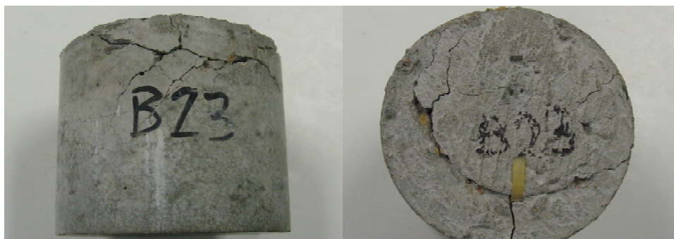
Figure 3-17 Cracks due to Differential Thermal Expansion
