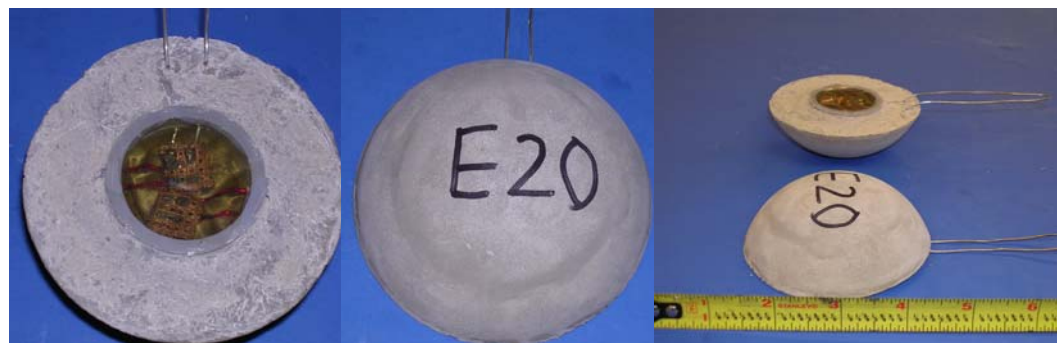
Figure 7-9 Sensor with Fiber-Reinforced Cement Paste Housing with Epoxy Core
