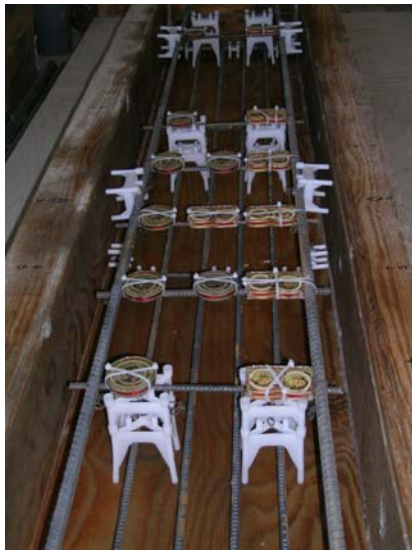
Figure 4-4 Layout of Sensors and Steel Reinforcement
