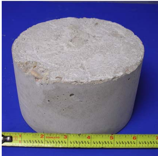
Figure E-11 Concrete Prism
