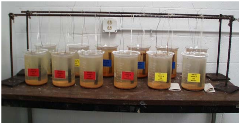
Figure 3-1. Accelerated corrosion test setup
