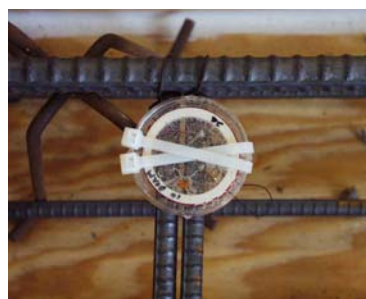
b) Positioning of sensor
