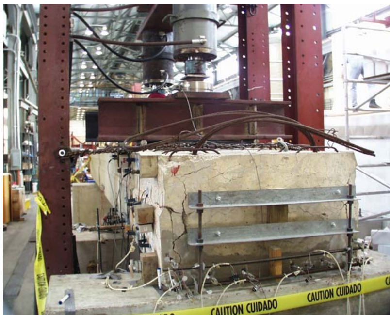
Figure 3.2 – Test Setup of Shear-Dominated Fatigue Test
