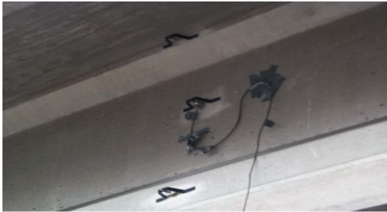
Figure 5.11 – Arrangement of Acoustic Emission Sensors
