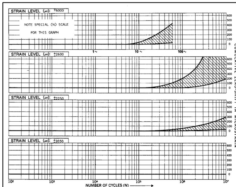
*Figure 5-18: Strain gage fatigue test results (Vishay, 2007)*
