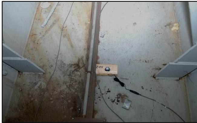
*Figure 3-22: Typical accelerometer installation at Bridge B*
