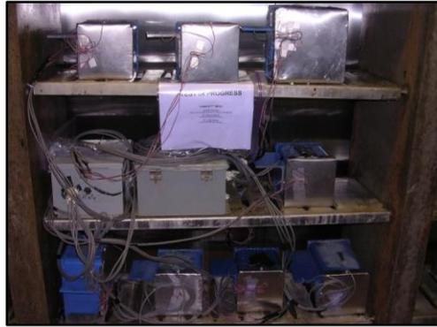
***Figure 5-14: Steel test-boxes inside humidity room***
