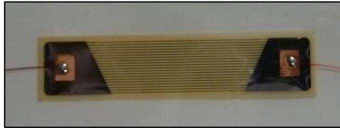
*Figure 5-20: Crack propagation gage*
