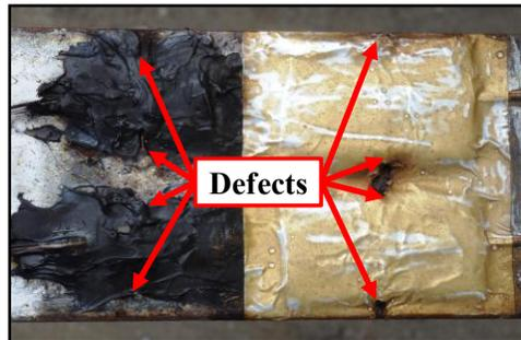
***Figure 6-15: Steel bar instrumented with bondable foil gages and defective protective coatings at the mid-length of the gage from both sides***
