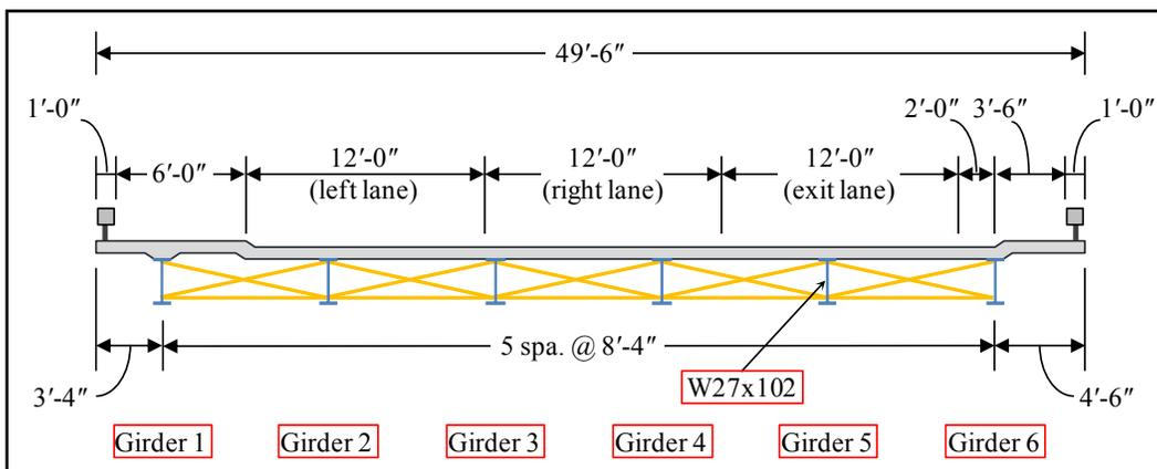
**Figure 3-28: Typical cross section of Bridge C**
