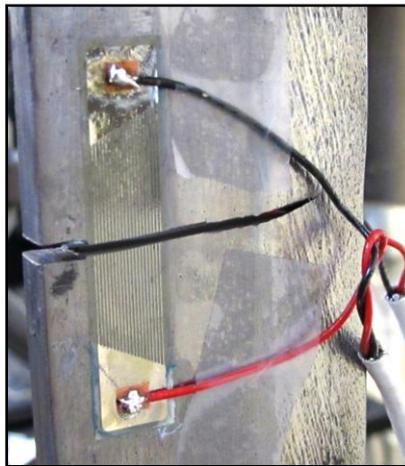
*Figure 6-39: Fatigue crack propagated through the width of the CP gage*
