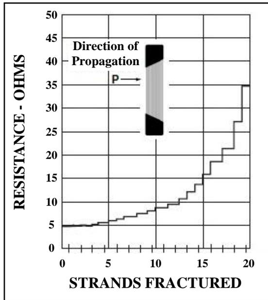
*Figure 2-13: Typical crack propagation gage output diagram (Vishay, 2012)*
