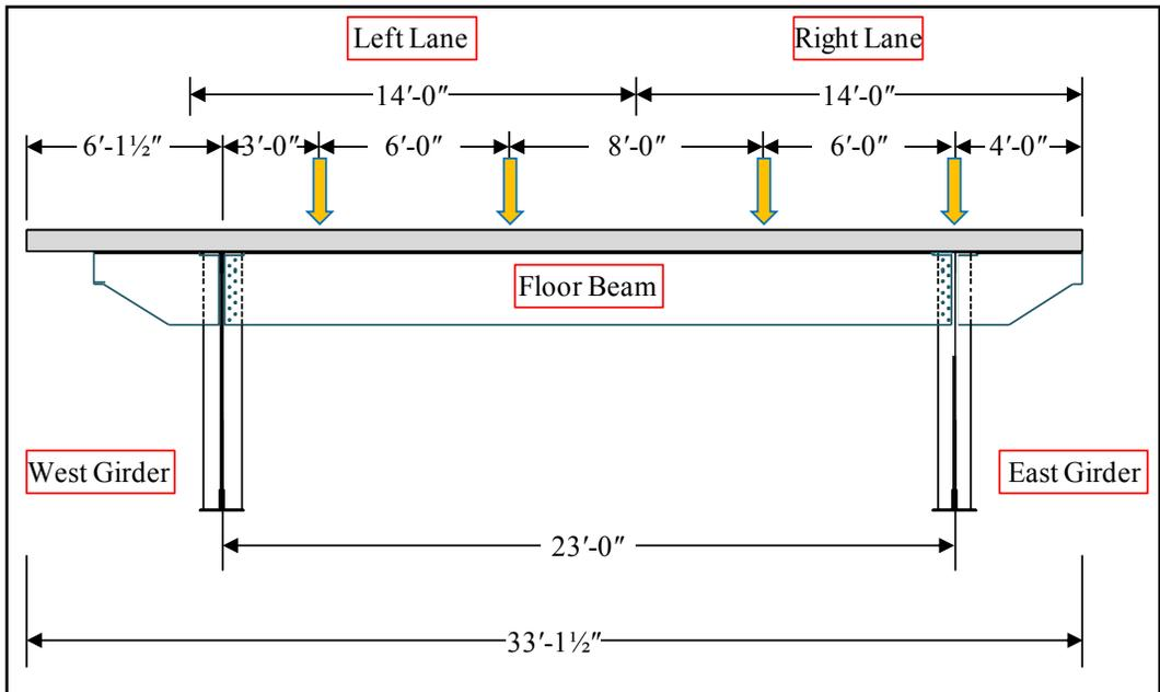
**Figure 3-7: Typical cross section of Bridge A**
