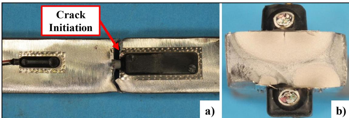
*Figure 6-29: Typical fatigue failure for weldable gages (LEA-L, LEA-R), a) plan view, b) cross-section*
