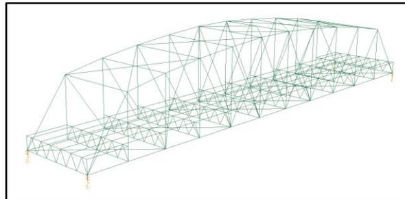
**Figure 4-11: Grillage model of Bridge E**
