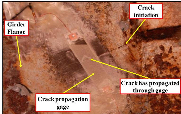
***Figure 6-43: Crack on (FB 34) propagated through the Gage 1***
