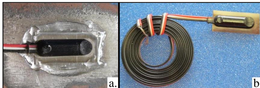
*Figure 2-11: Bondable shield strain gage with: a) stainless steel shim, b) polyimide shim*
