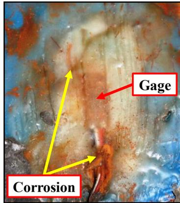
*Figure 6-26: Corrosion below protective coatings of bondable foil gage (CEA-C)*
