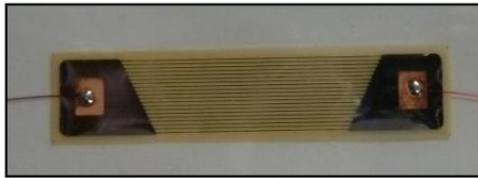
*Figure 1-6: Crack propagation gage*
