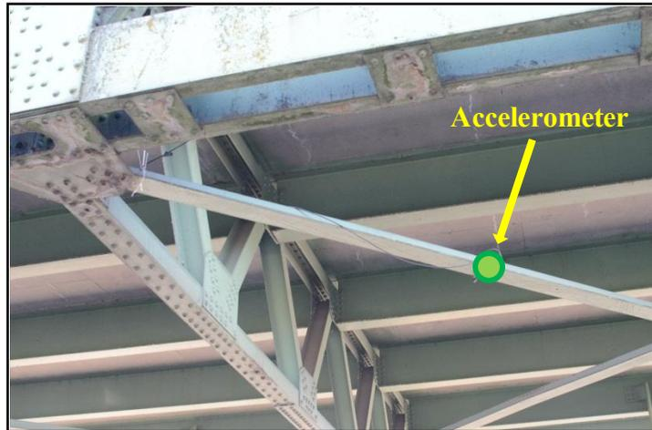
*Figure 3-39: Accelerometer placed to the midpoint of the bottom chord of Bridge E*
