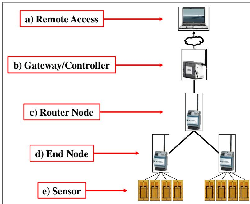
**Figure 1-3: Schematic of the wireless monitoring system components**
