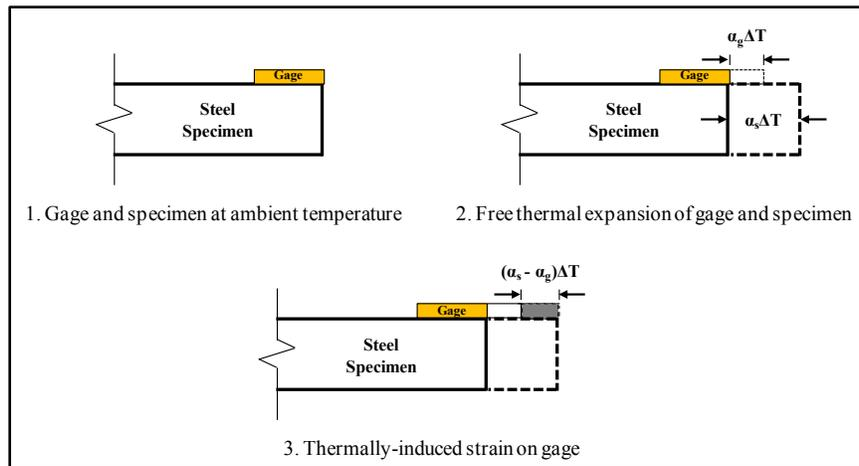
**Figure 5-1: Thermally-induced strain between specimen and strain gage**
