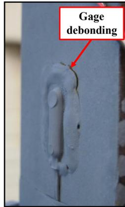
***Figure 6-10: Debonding of HBW-B gage***
