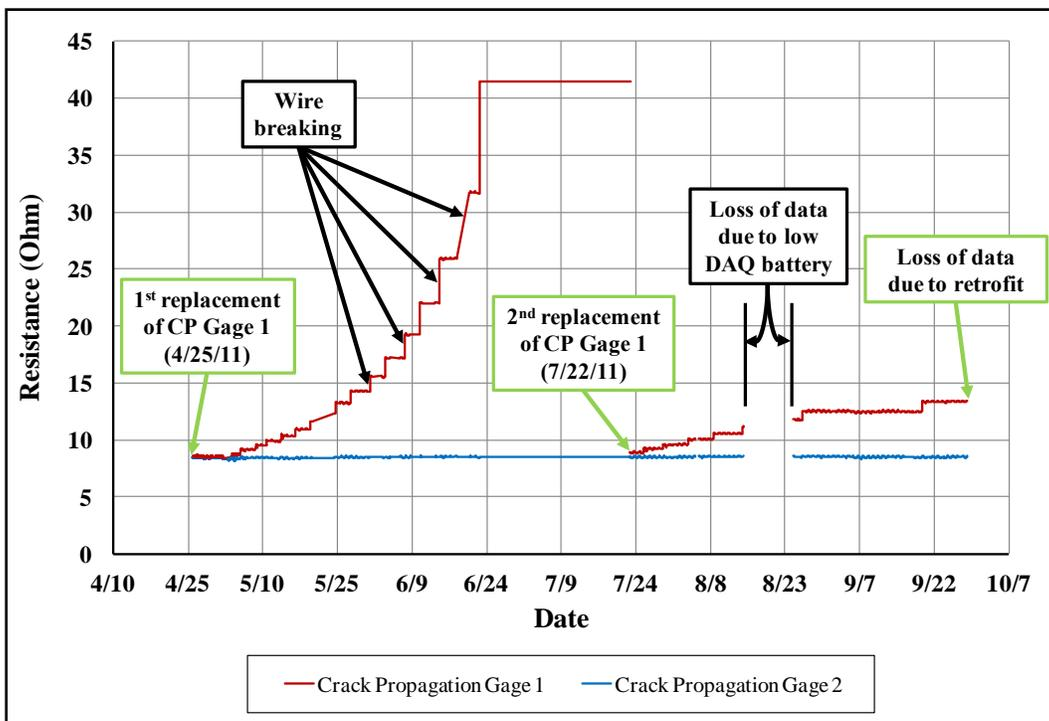
**Figure 6-44: Crack growth at floor beam 34 (Gage 1) and floor beam 38 (Gage 2) during 4/25-9/28/2011**
