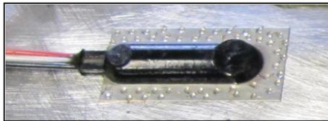
*Figure 2-10: Weldable strain gage*
