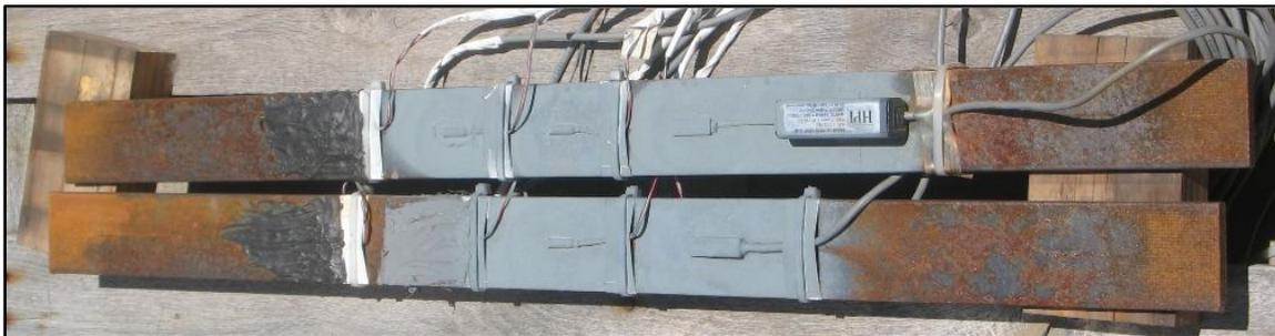
*Figure 5-5: Long steel bars instrumented with different types of gages*
