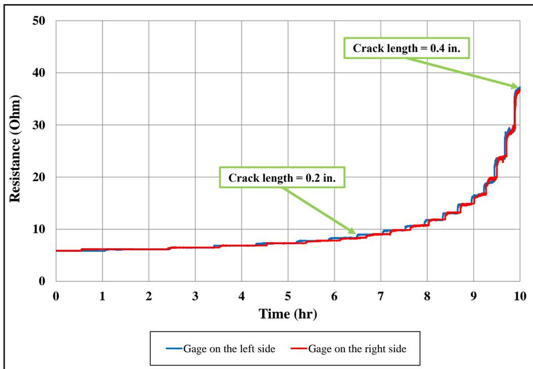
**Figure 6-40: Crack propagation gage output during fatigue test**
