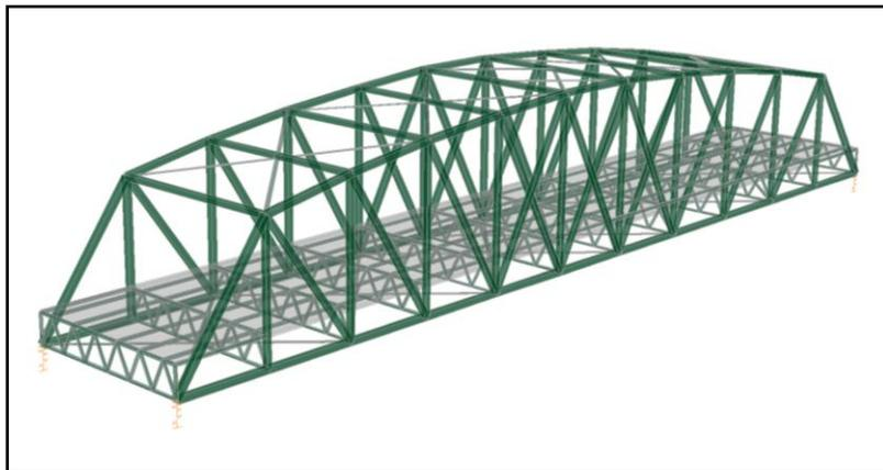
*Figure 4-6: 3D model of Bridge E in SAP 2000*
