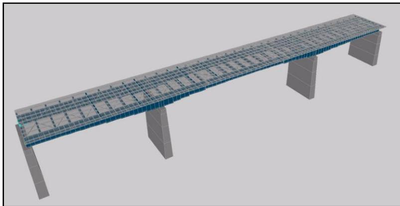
*Figure 4-3: 3D model of Bridge A in SAP 2000*
