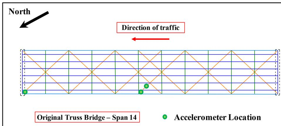
*Figure 3-37: Accelerometer locations at Span 14 of Bridge E*
