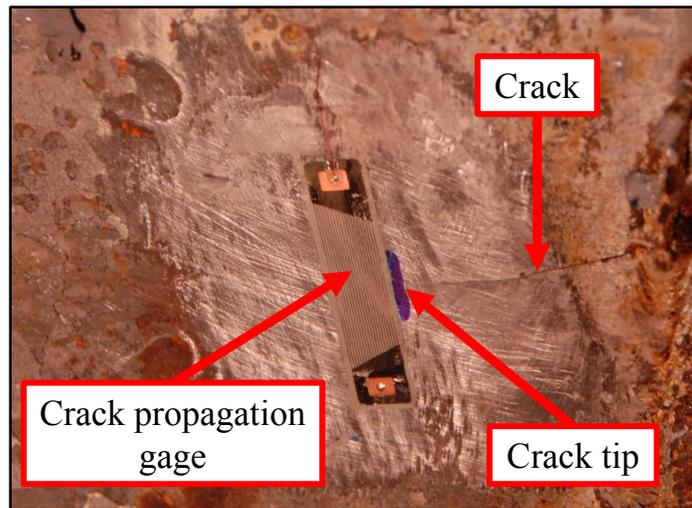
*Figure 5-22: Crack propagation gage installed on Bridge A*
