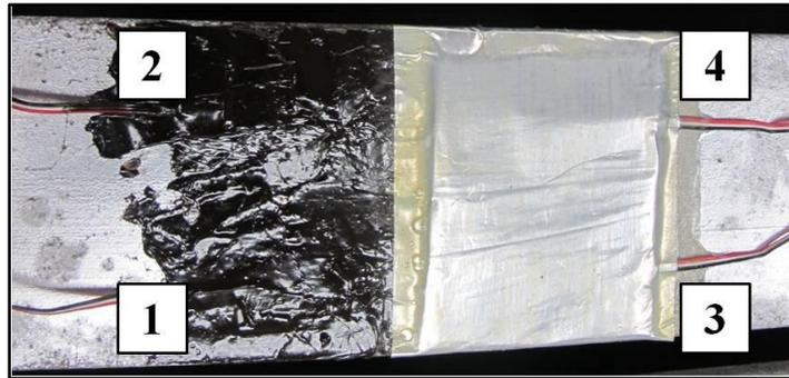
**Figure 5-10: Typical instrumentation of 14 steel bars**
