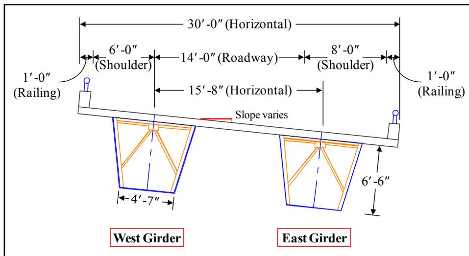
**Figure 3-21: Typical cross section of Bridge B**
