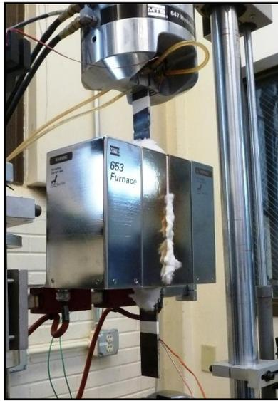
*Figure 6-18: Steel bar placed inside a MTS furnace*
