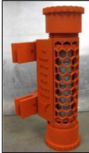
*Figure 2-1: UT Austin vibration energy harvester (Dierks, 2011)*
