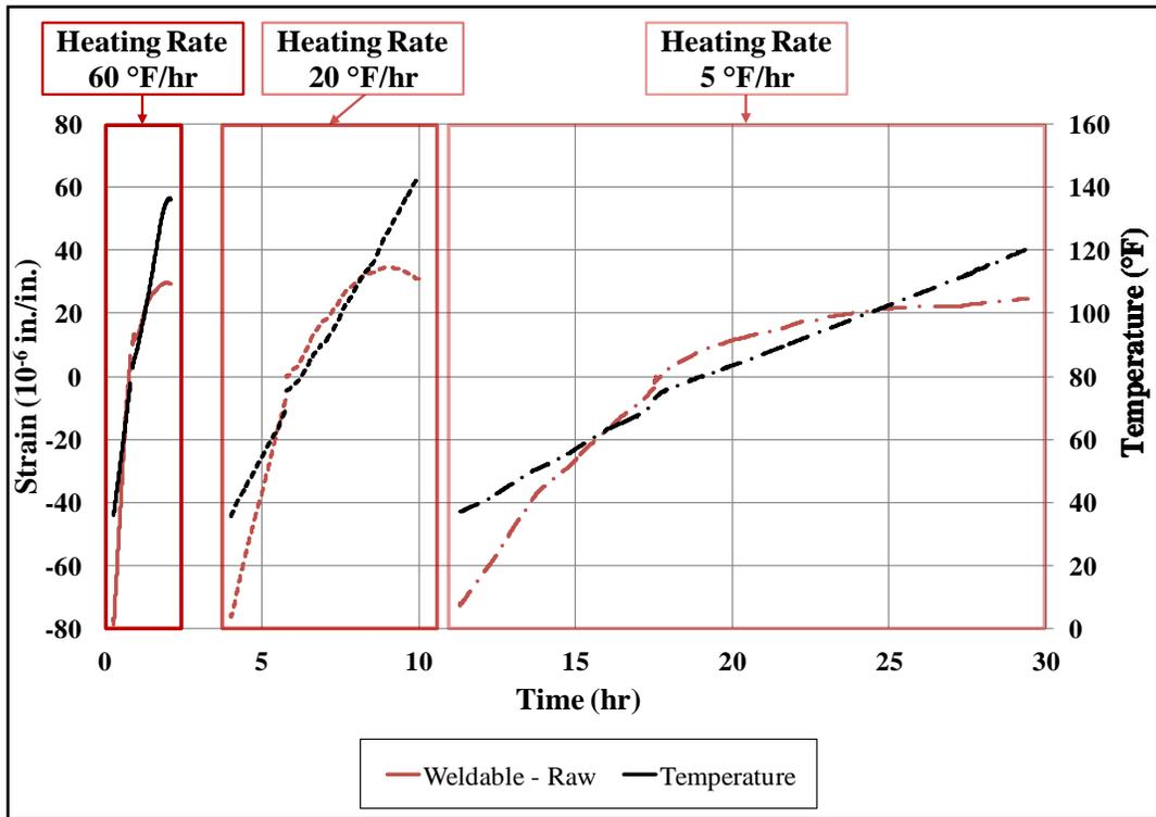
Figure 6-21: Weldable gage response at different heating rates
