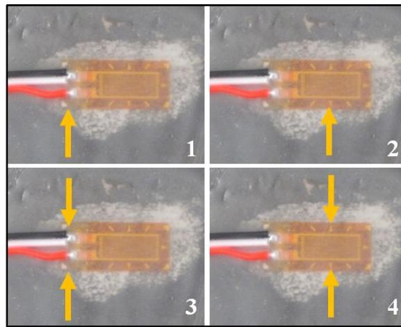
**Figure 5-11: Location of the different defect types**
