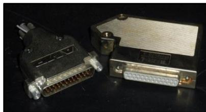
***Figure 5-15: Serial port connectors***
