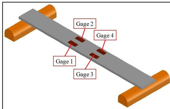
*Figure 5-8: Steel bar specimen instrumented with strain gages*
