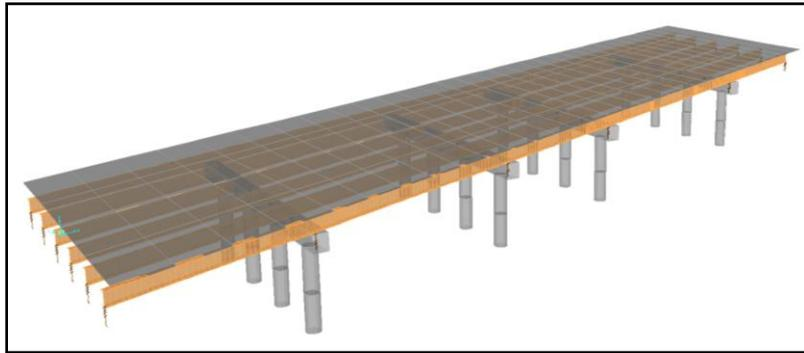
*Figure 4-5: 3D model of Bridge C in SAP 2000*
