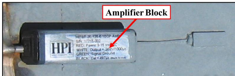
*Figure 6-6: Amplifier block of amplified weldable gage*
