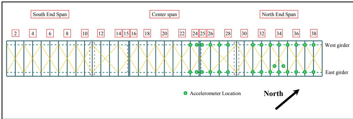
**Figure 3-14: Locations of the accelerometers at Bridge A**
