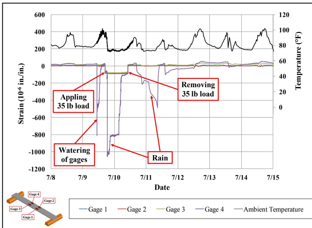
**Figure 6-16: Strain history during moisture validation test**
