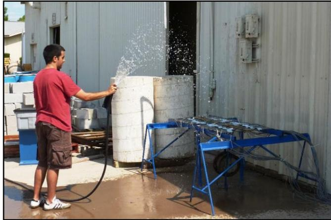
***Figure 6-14: Watering steel bars located outside FSEL***
