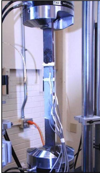
*Figure 5-6: Testing of long steel bar*
