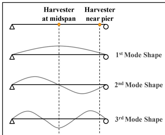
**Figure 4-15: Modes of vibration of a simply-supported beam**
