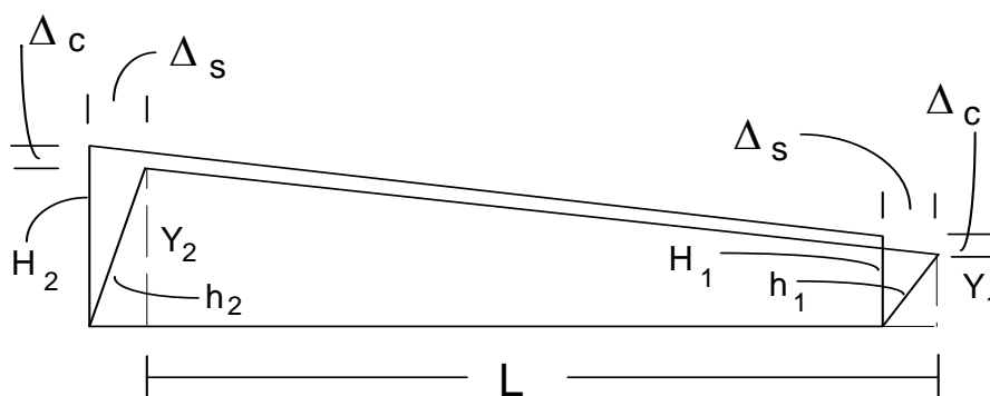
Figure 3.7 Geometry of Displaced Bearing
