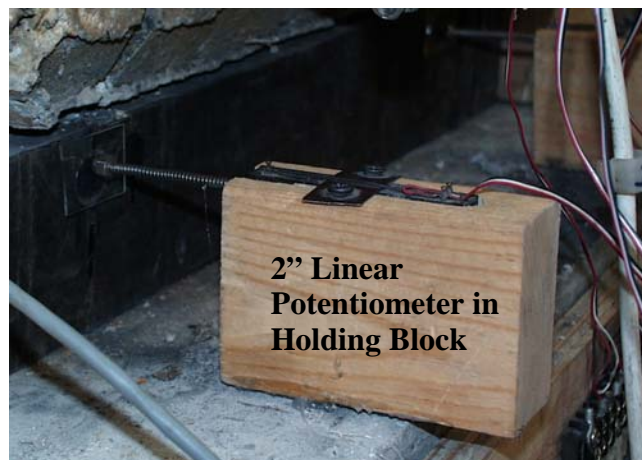
Figure 5.8: Horizontal Displacement Measurement of Bearing Pad
