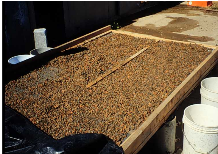
Figure 3.20 Drying of Aggregate on Screened Bed
