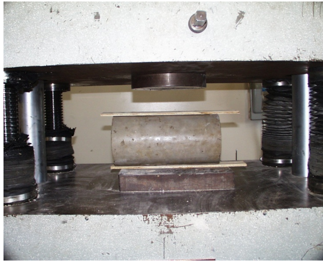
Figure 3.10 Test Setup for Splitting Tensile Test
