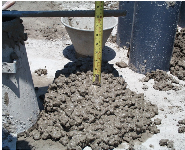
Figure 5.9 Slump for Third Batch of 8000 psi Concrete
