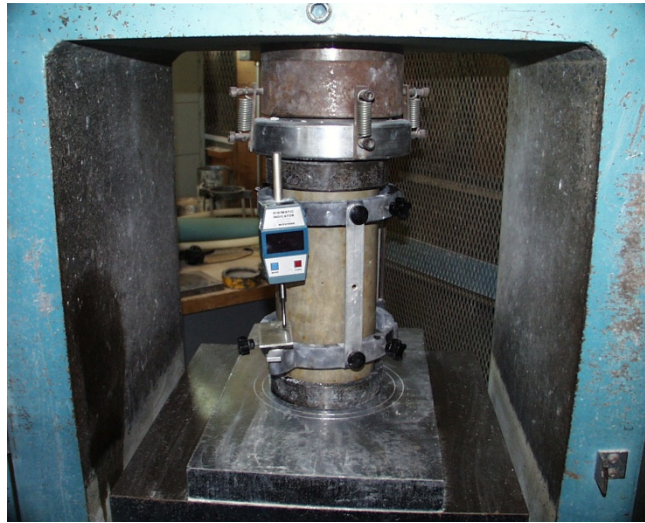
Figure 3.7 Test Setup for Modulus of Elasticity
