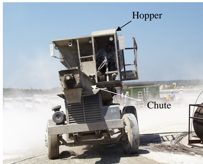
Figure 4.1 Sidewinder at Heldenfels Precast Plant
