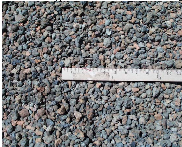
Figure 3.14 Appearance and Maximum Size of Clodine Aggregate
