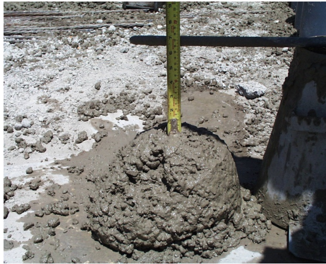
Figure 4.9 Slump of Second Batch of 6000 psi Concrete
