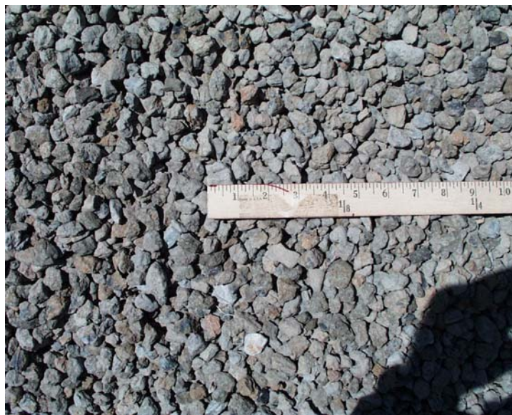
Figure 3.18 Appearance and Maximum Size of Western Aggregate
