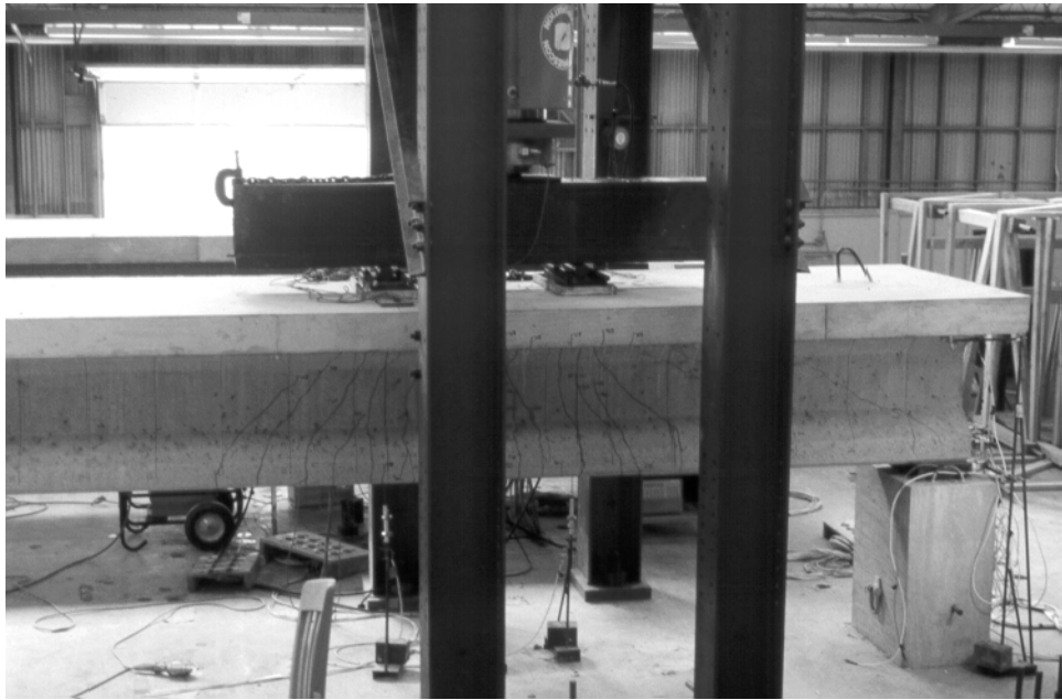
Figure 7.2: Load Application Components— Test H0R-D-66
