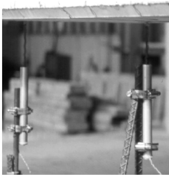
Figure 7.6: Linear Potentiometers Used to Measure Beam Deflection
