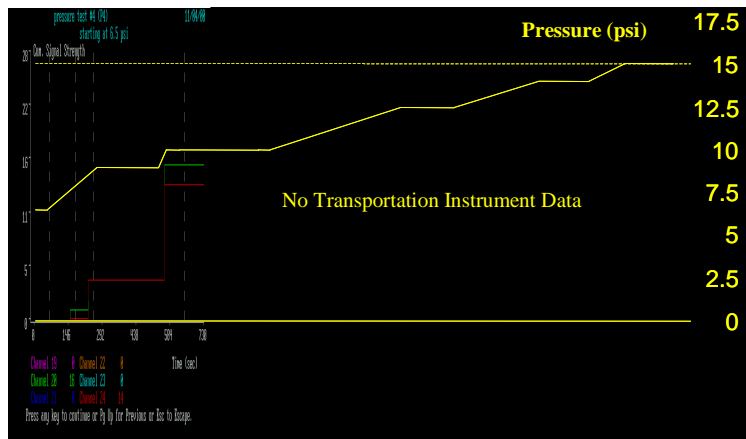
Figure 10.35 – Fourth pressure test – original vessel (Channels 19-24) Transportation Instrument
