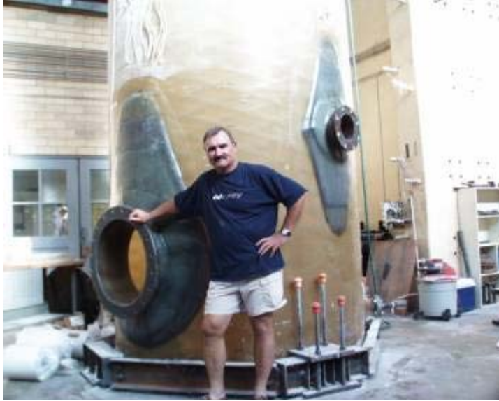
Figure 8.4 – Photograph of new manway and new 8”nozzle (exterior of vessel)
