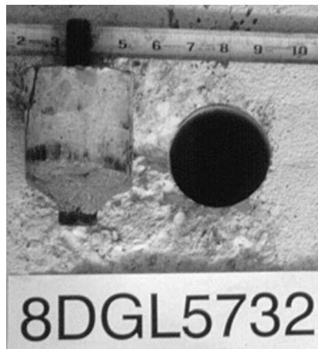
Figure 5.5 Typical Breakout Body in Dynamic Tests of Grouted Anchors
