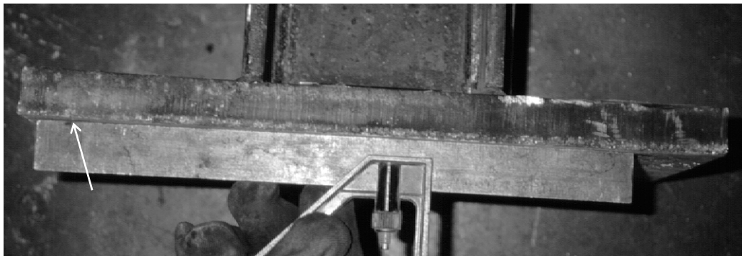
Figure 5.16 Deformation of Flexible Baseplate after Testing
