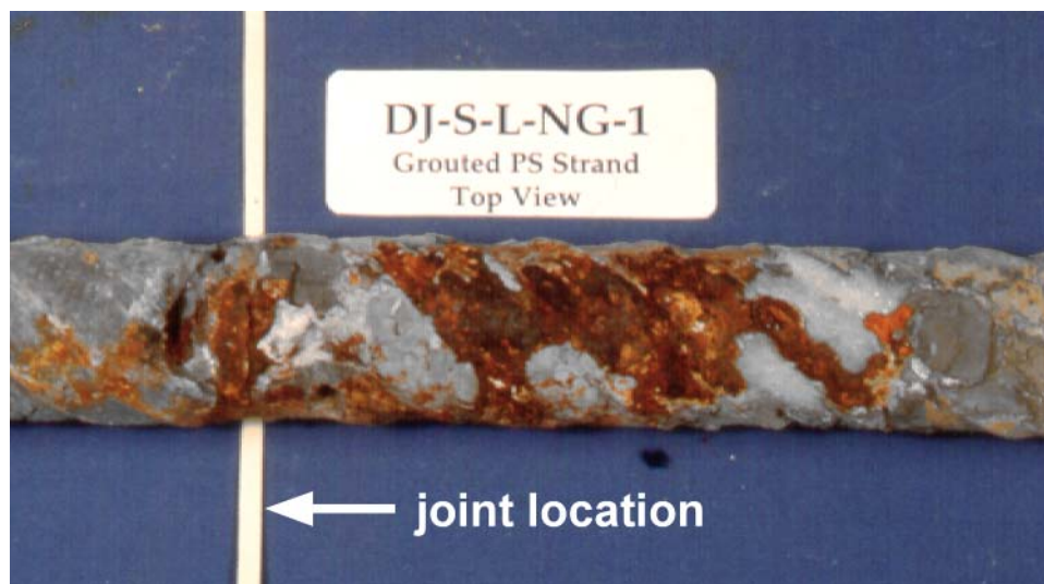
Figure 5.27 - Heavy Rust Staining on Grout Surface
