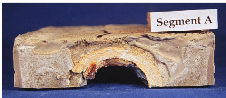
Figure 5.33 - Incomplete Epoxy Coverage In Epoxy/Gasket Joint (EG-S-M-NG-2)
