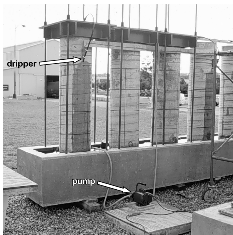
Figure 4.11 - Trickled Saltwater Exposure for Columns
