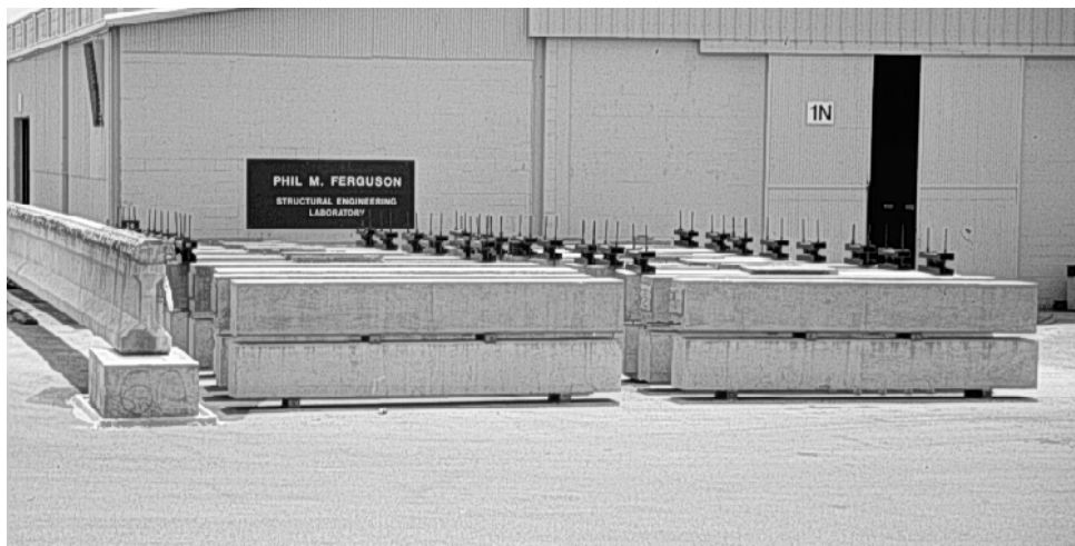
Figure 3.22 - Beam Test Setup at North End of Ferguson Laboratory
