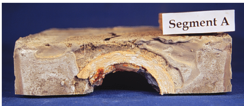
Figure 5.33 - Incomplete Epoxy Coverage In Epoxy/Gasket Joint (EG-S-M-NG-2)
