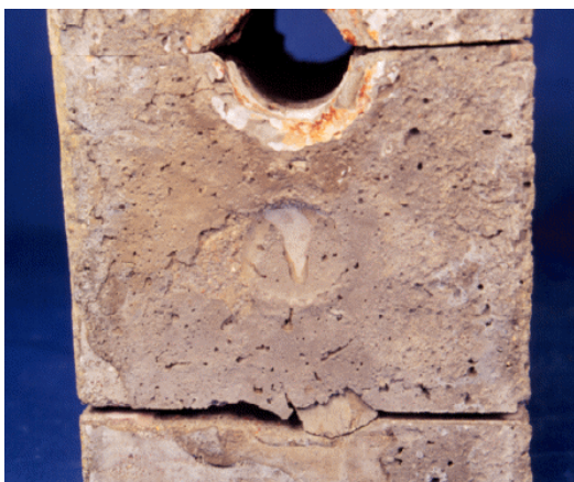
Figure 5.30 - Grout Infiltration Into Joint: Specimen DJ-S-L-CI-1
