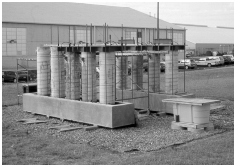
Figure 4.10 - Long Term Column Corrosion Test Setup
