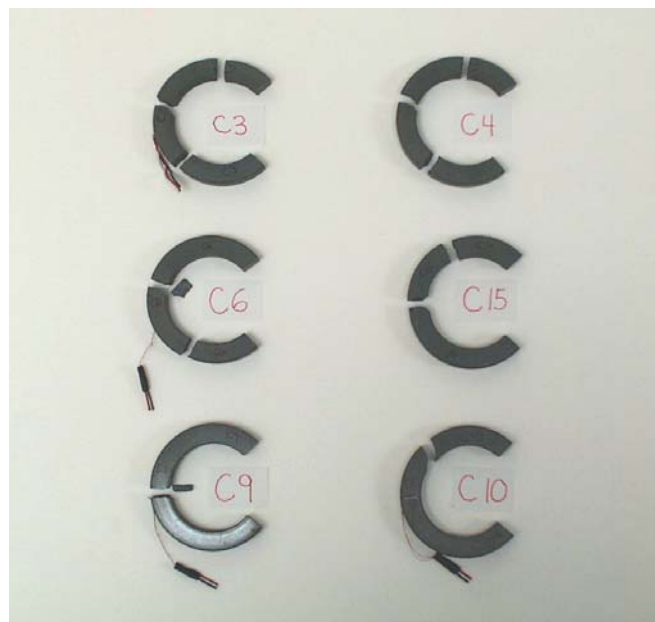
Figure 4.9 Pictures of the failed specimens
