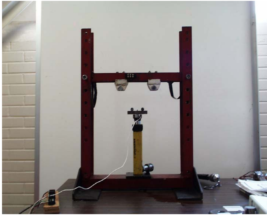
Figure 3.2 The loading frame used for the flexural testing of the bar specimens
