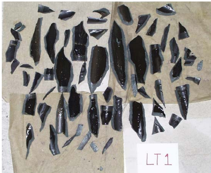
Figure 5.33 Fractured sections from LT1
