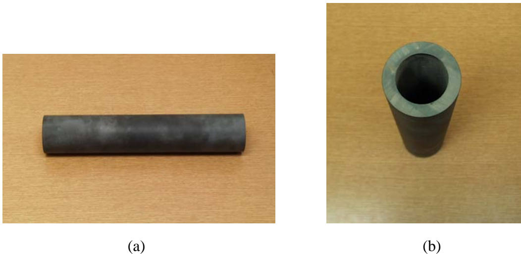
Figure 1.1 An example of a silicon carbide tube (a) side view (b) looking at the cross-section
