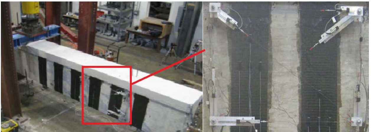
Figure 2-26 LVDTs configuration for shear strain
