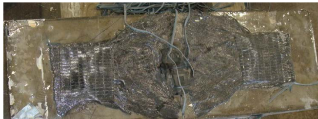
Figure 5-39 Anchored strip attached on the tensile surface of specimens (Huaco, 2009)
