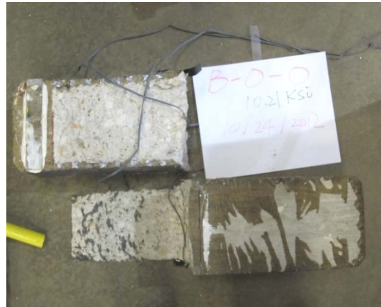
Figure 3-8 Debonding observed between CFRP strip and concrete substrate
