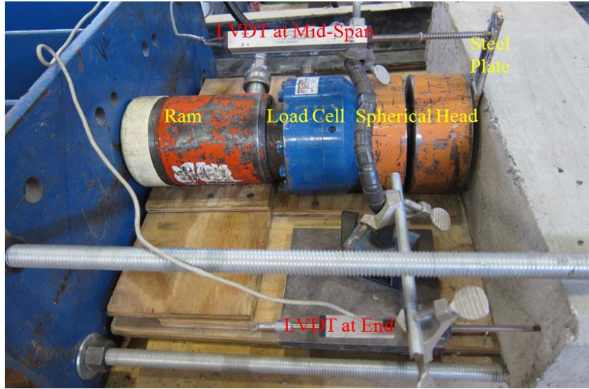
Figure 3-28 Measurements for load and displacement
