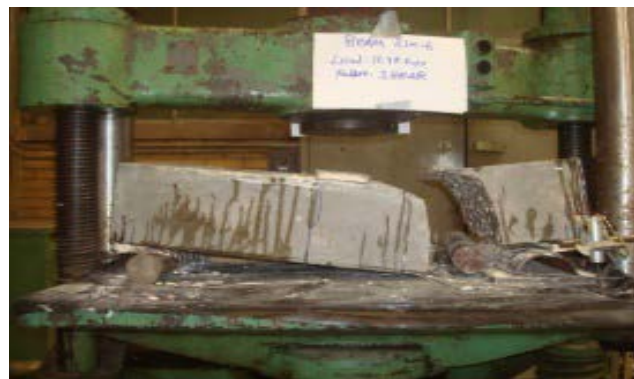
a) Shear concrete failure (Huaco, 2010)
