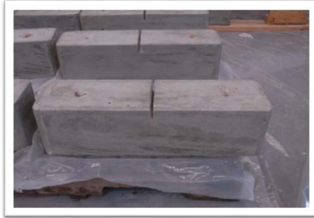
Figure 3-1 Standard specimen before CFRP installation
