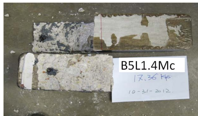
Figure 4-15 CFRP anchor rupture
