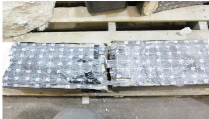
Figure 4-14 CFRP strip fracture
