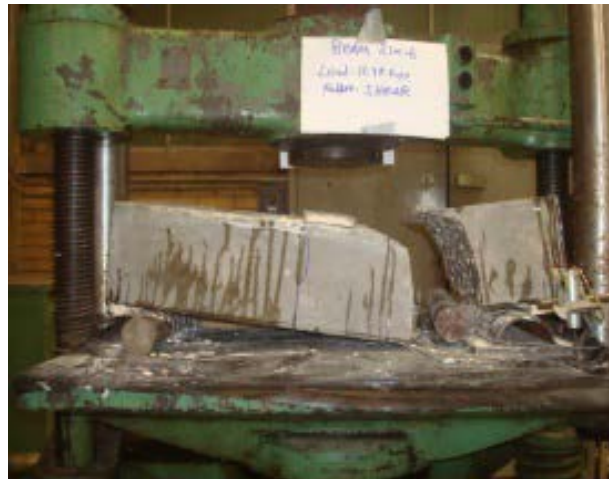
Figure 3-2 Pure concrete specimen failed in shear (Huaco, 2010)
