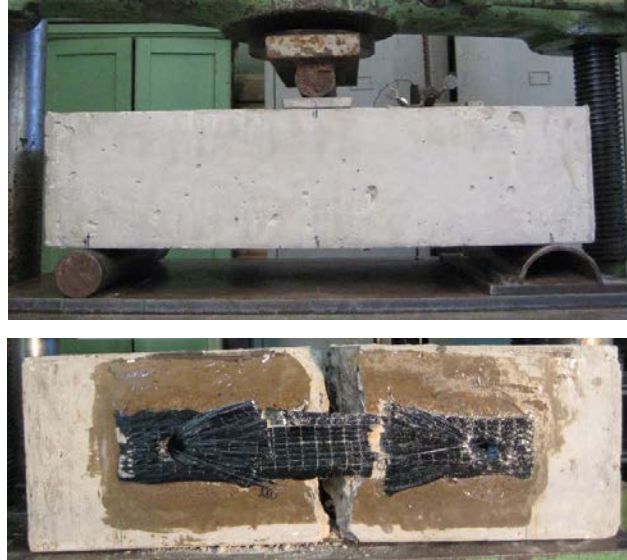
Figure 2-13 A simple test setup for quality control of CFRP anchors (Pham, 2009)
