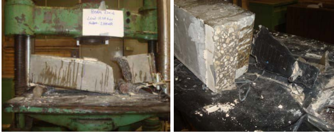
Figure 4-16 Concrete beam shear failure (Huaco, 2010)
