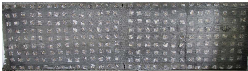
Figure 3-32 Targets affixed on tension surface of a beam specimen
