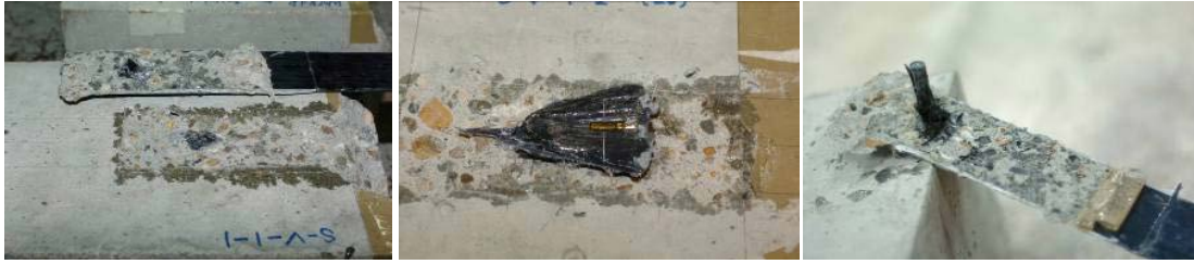
(a) Anchor shear failure (b) Anchor fan failure (c) Anchor pullout failure
