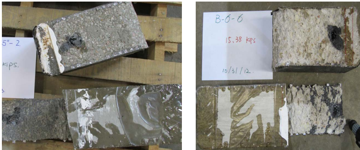
(a) High strength concrete (b) Normal strength concrete Figure 4-22 Concrete and CFRP surfaces after debonding
