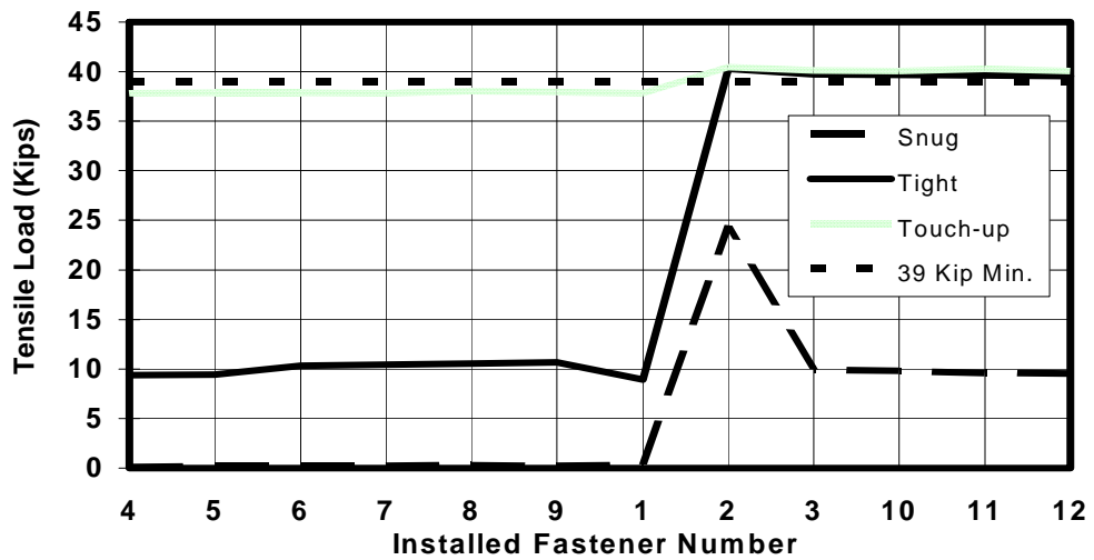
Figure B.60: Tensile Load History for Fastener #2 - Test CD3CW254.MTO
