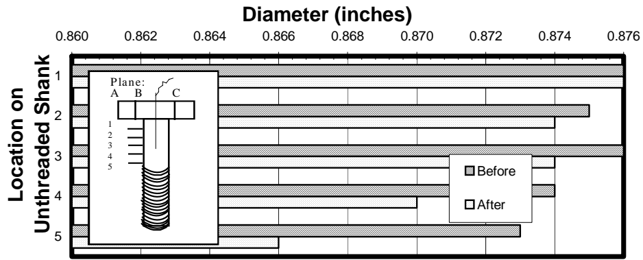
Figure 3.26: Before/After Diameters in Plane A, Unlubricated Nut, Flat
