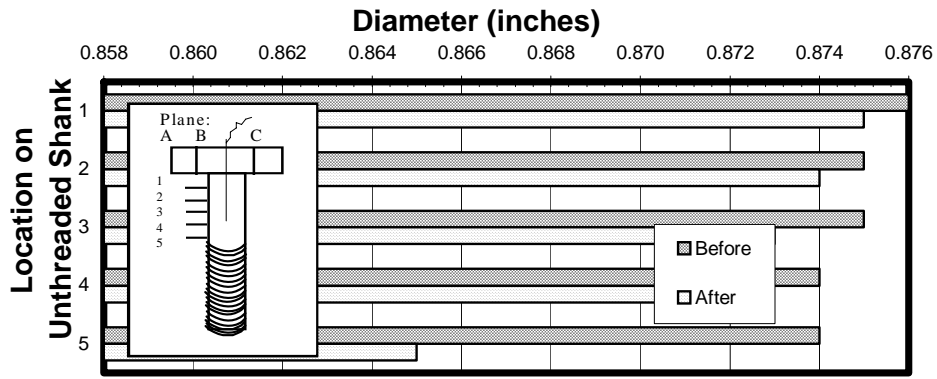
Figure 3.31: Before/After Diameters in Plane A, Unlubricated Nut, Beveled
