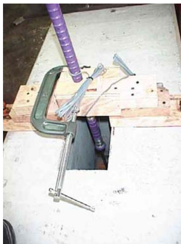
Figure 4.16: Bar Ready for Grouting in SLGP
