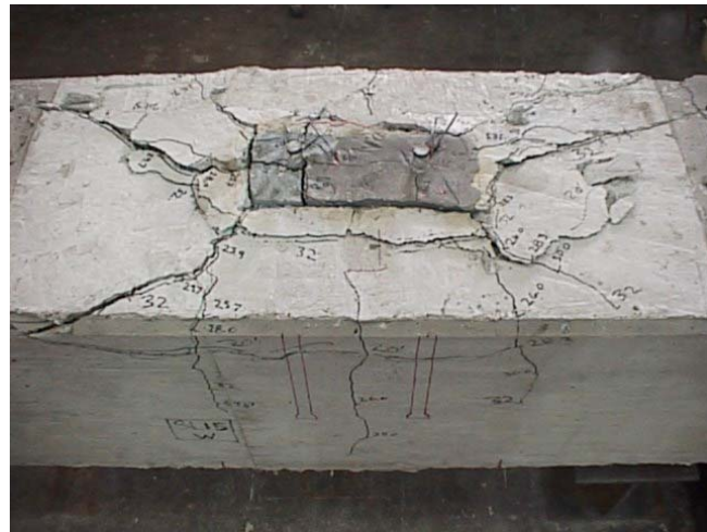
Figure 5.16: SL15 Breakout Surface Cracks
