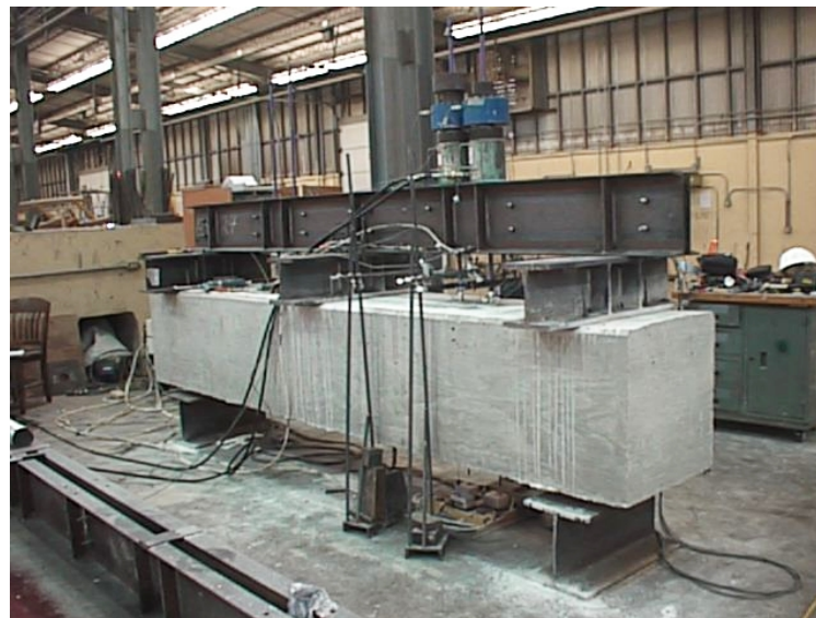
Figure 4.5: Typical Completed Test Setup
