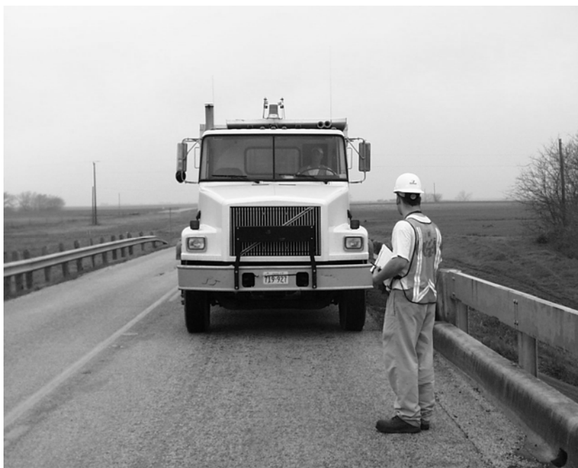
Figure 3.19 Photograph of the Single-Truck Loading Configuration
