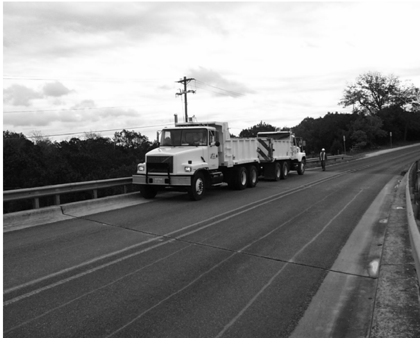
Figure 3.15 Photograph of the Back-to-Back Loading Configuration
