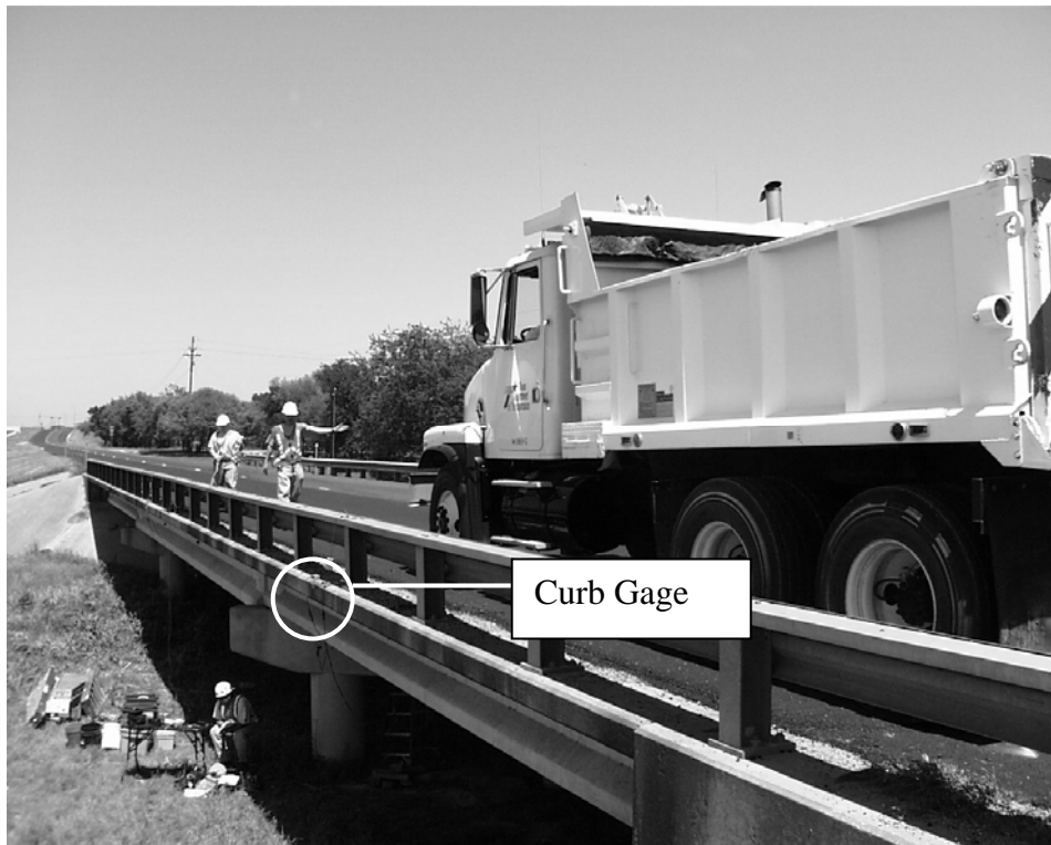
Figure B.9 Curb Gages – Chandler Creek Bridge
