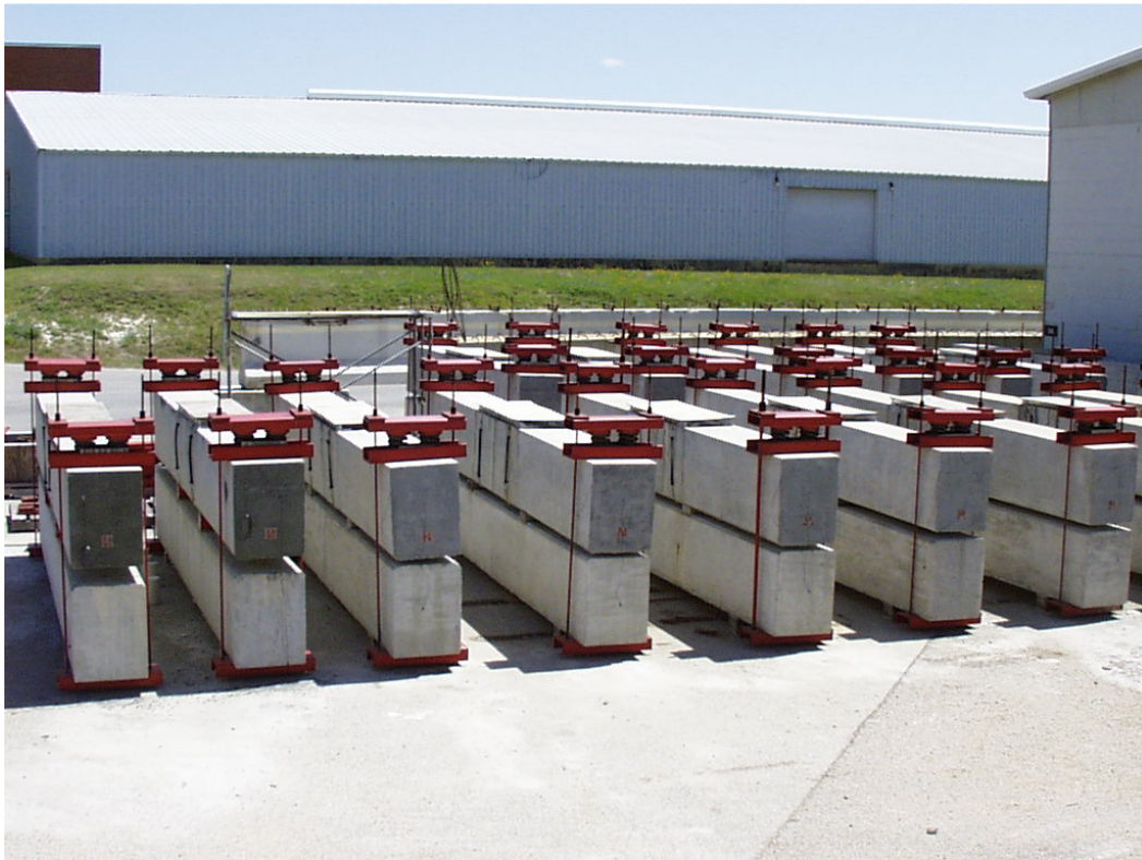
Figure 6.2 The saltwater ponding beams (from an ongoing project at Ferguson Structural Engineering Laboratory) used for corrosion rate testing.
