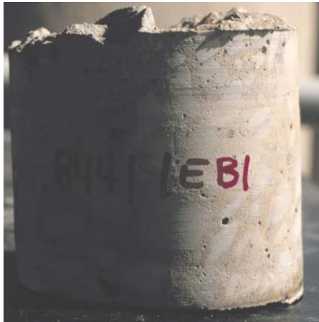
Figure 5.7 Permeability core taken from Structure #10.
