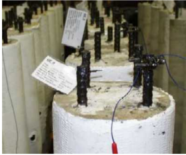
Figure G.2 The exposure environment for the circular specimens.
