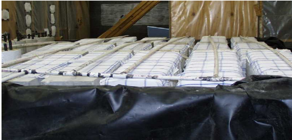
Figure G.3 The exposure environment for the rectangular specimens.
