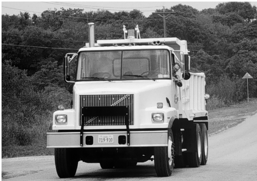
Figure 3.16 TxDOT Loading Vehicle
