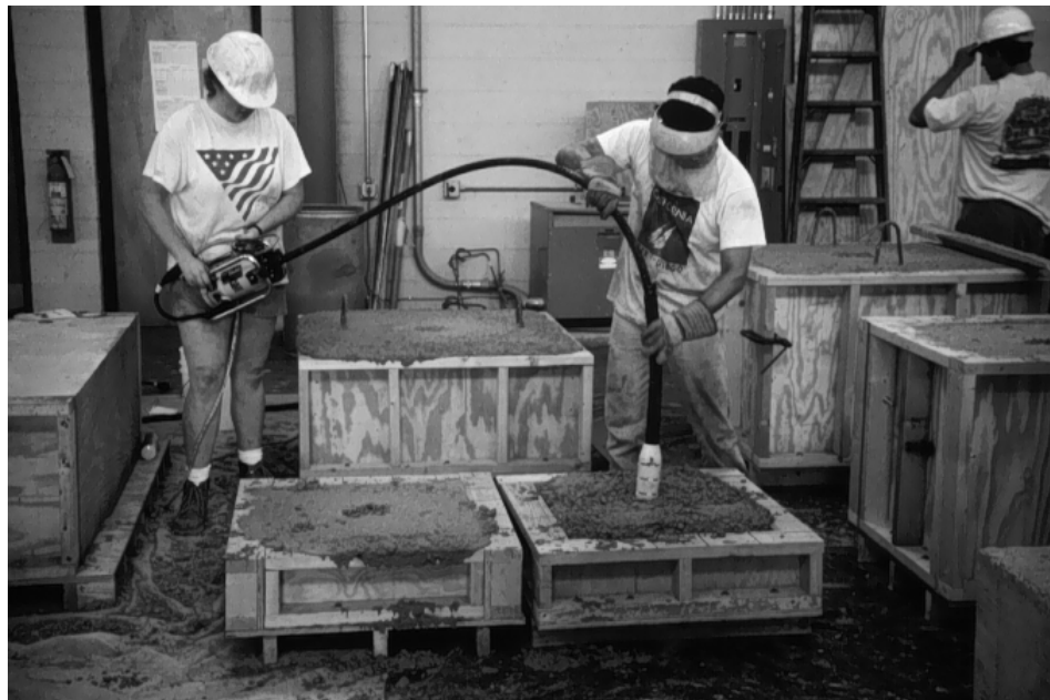
Fig. 7.10: Consolidation of specimen 20.5 cm (8 in) high.
