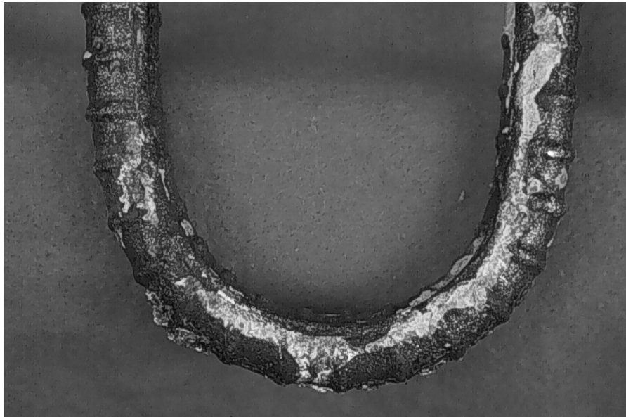
Fig. 8.35: Whitish products alongside longitudinal lug at bottom side of bar 1A.5.
