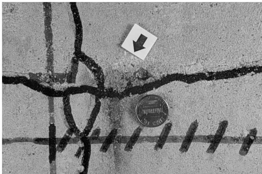
Figure 9.50: Horizontal cracking on front surface of beam B32.
