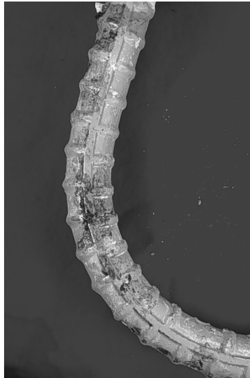
(a) Rust staining and blistering on epoxy-coated bar.
