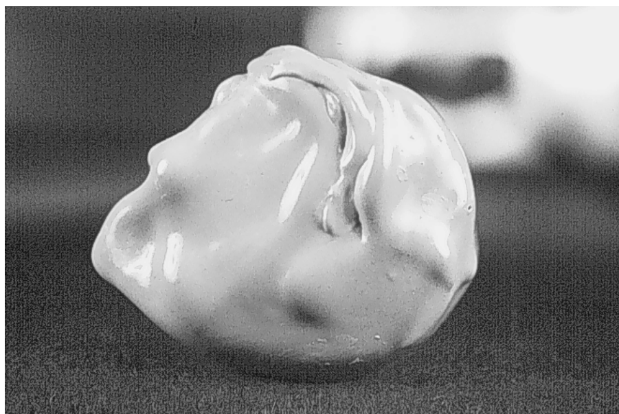
Figure C.4: Repaired bar end. Epoxy material was spread with a small wooden stick.
