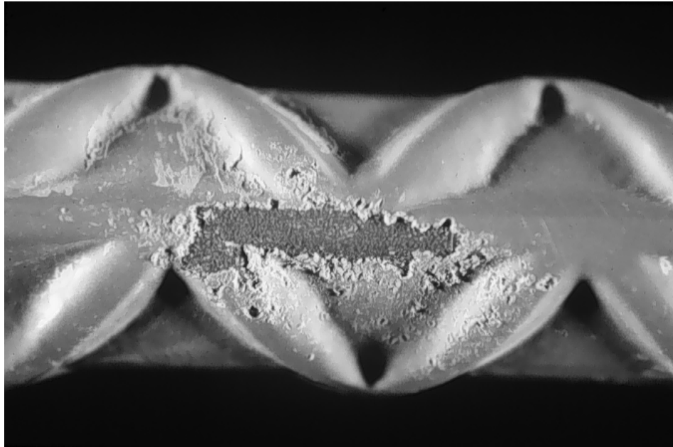
Fig. 7.6: Damage to coating caused by metal head vibrator on test bar from Phase 1 study.
