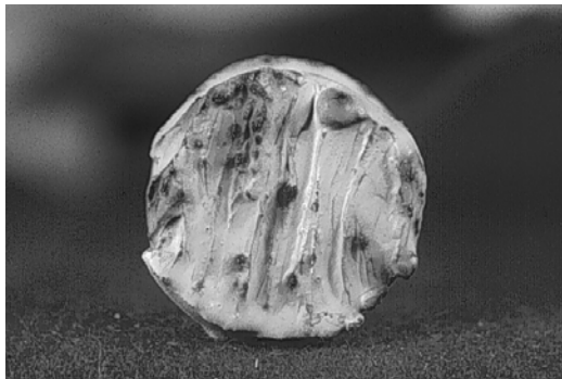
(a): Appearance after 53 days of immersion in 3.5% salt solution.
