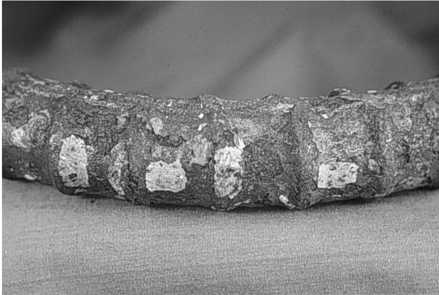
(a) Patched bar 3B.2, outside bend.
