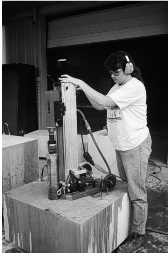
Fig. 7.11: Coring reinforced concrete test specimen.
