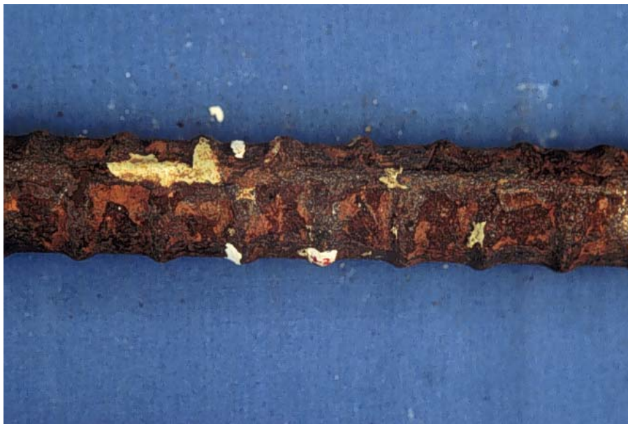
(a) Zone around crack location near the edge of wetted region.
