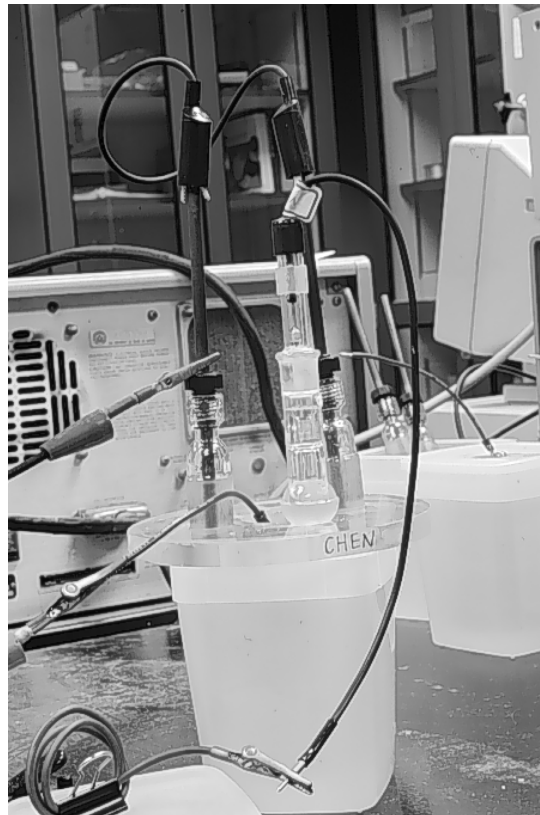
Figure 6.31: Test setup for EIS and polarization resistance tests.
