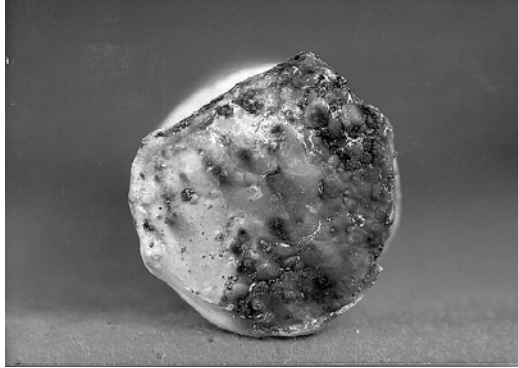
(a): Corrosion of patched end (shear-cut).
