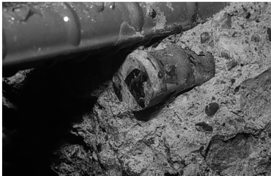
(b) Lower splice bar, appearance of bar end at time of autopsy.
