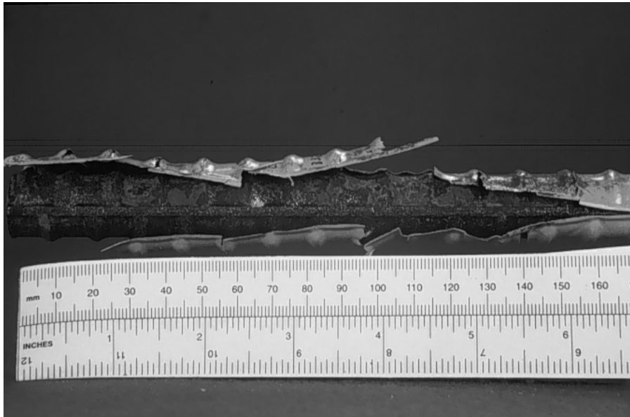
Fig. 9.67: Coating debonding of splice bar within the wetted region (beam B32).
