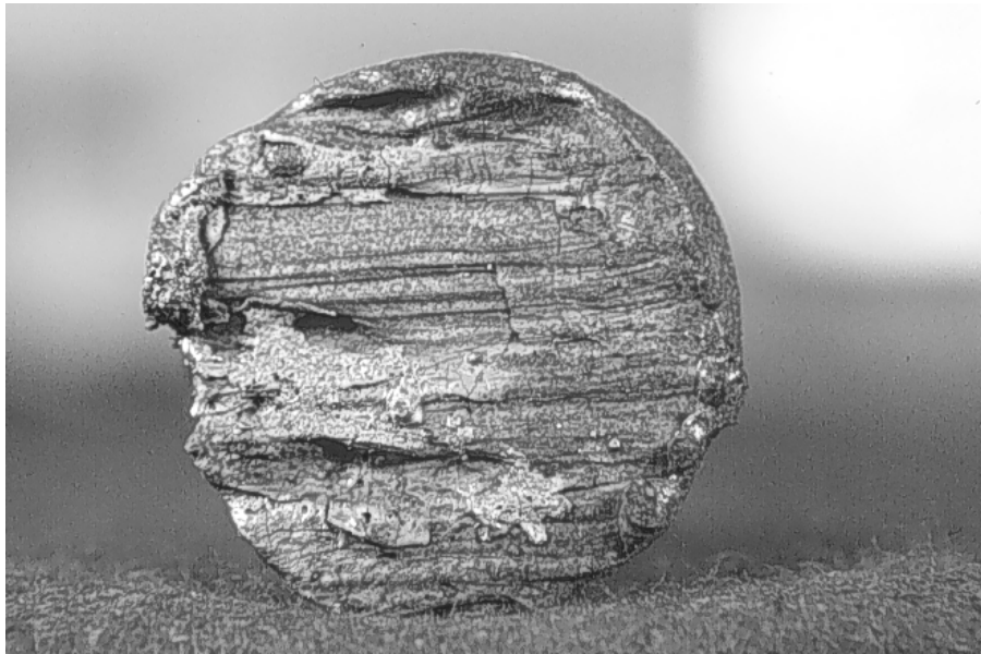
(a): Torch-cut bar end after 2 weeks of exterior exposure
