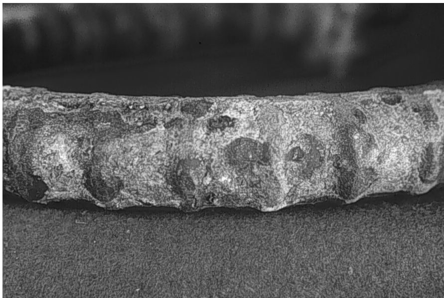
Fig. 8.36: Various rust products above uniformly black corroded surface under the coating.
