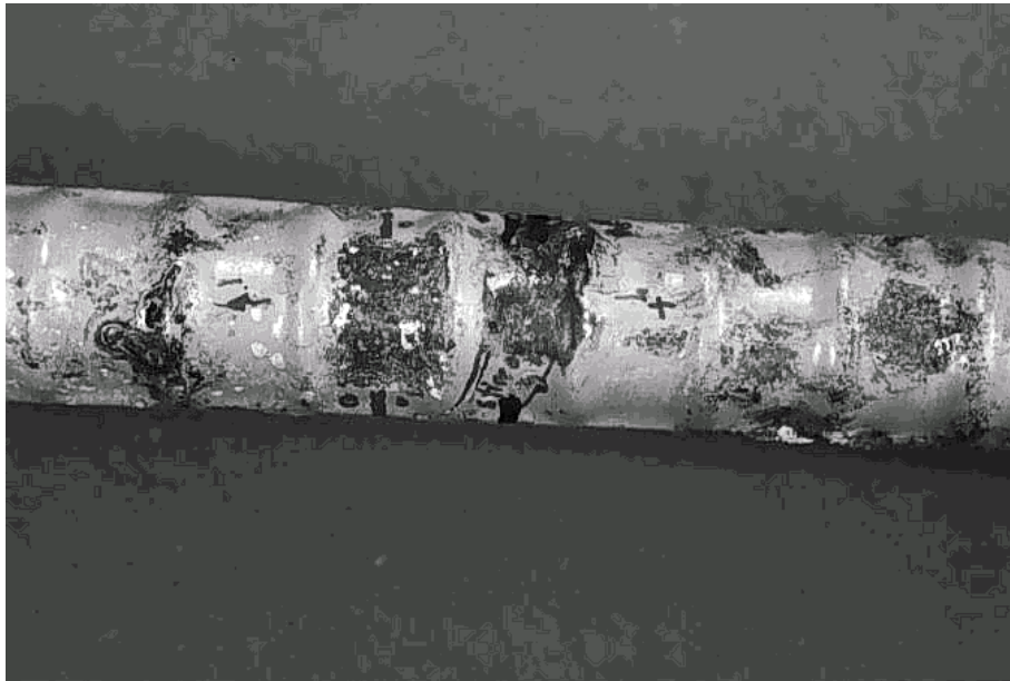
(b) Bar of beam B10, portion at midspan (wetted zone).
