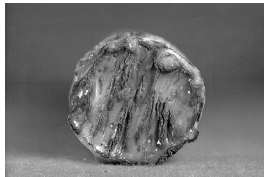
(b): Appearance after 200 days of immersion.
