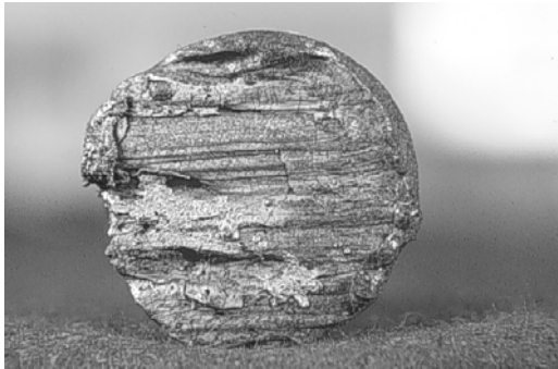
(e): Appearance of torch-cut end after two weeks of exterior exposure.
