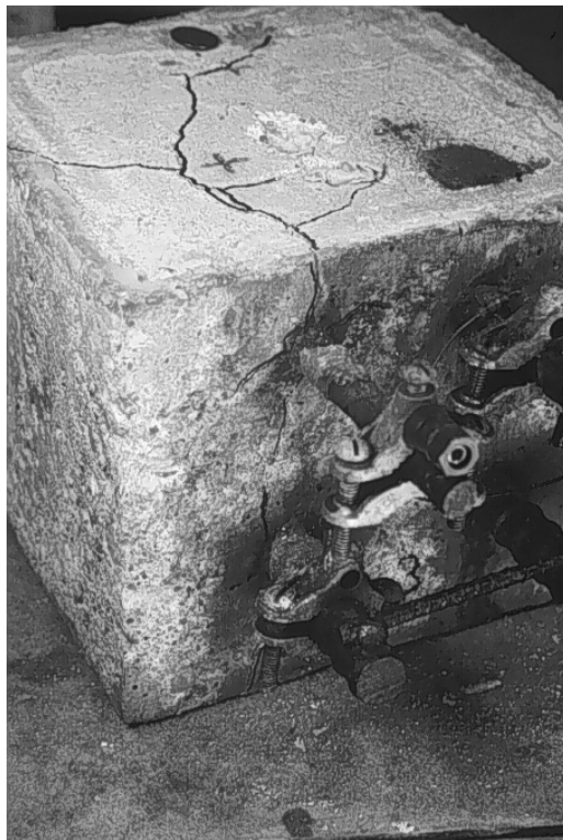
Fig. 8.13: Specimen surface condition of specimen with uncoated bar.
