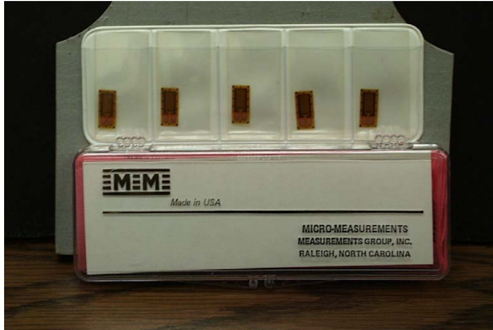
Figure 3.2. Strain Gages Used on Plastic Surfaces.
