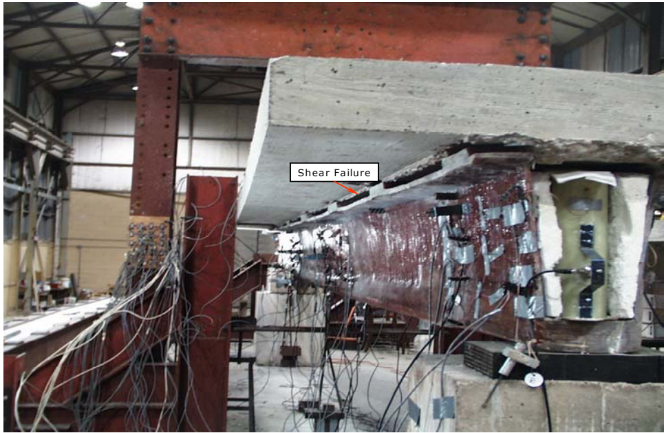
Figure 8.16. Shear Failure at Deck-Girder Interface at South End.
