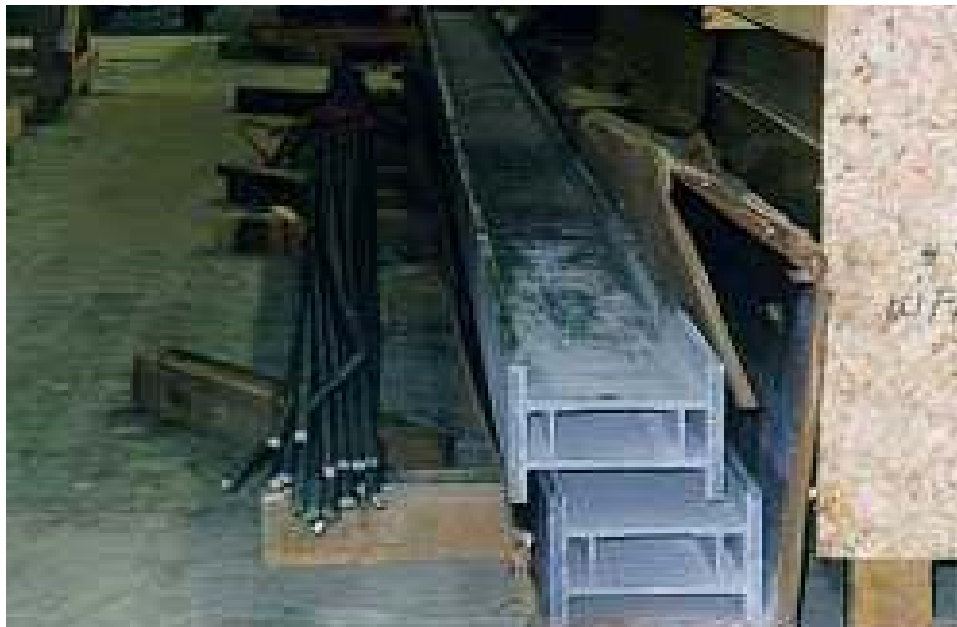
Figure 7.1. FRP Hybrid Girders Laid Sideways.
