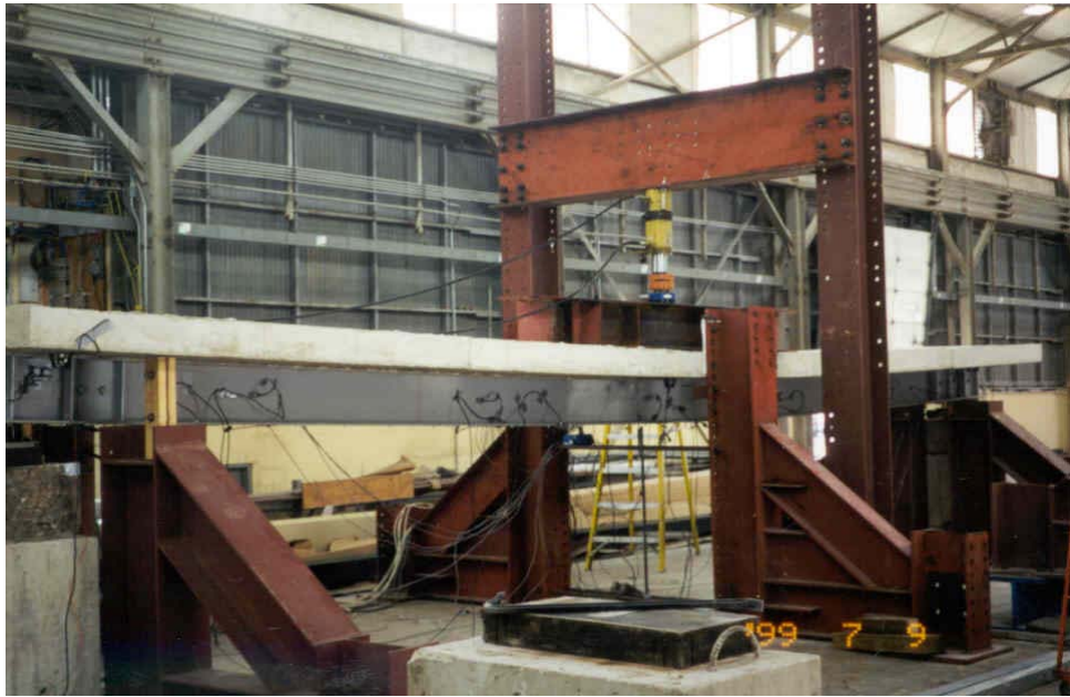
Figure 5.17. Specimen Without Tubes, Excessive Deflections.
