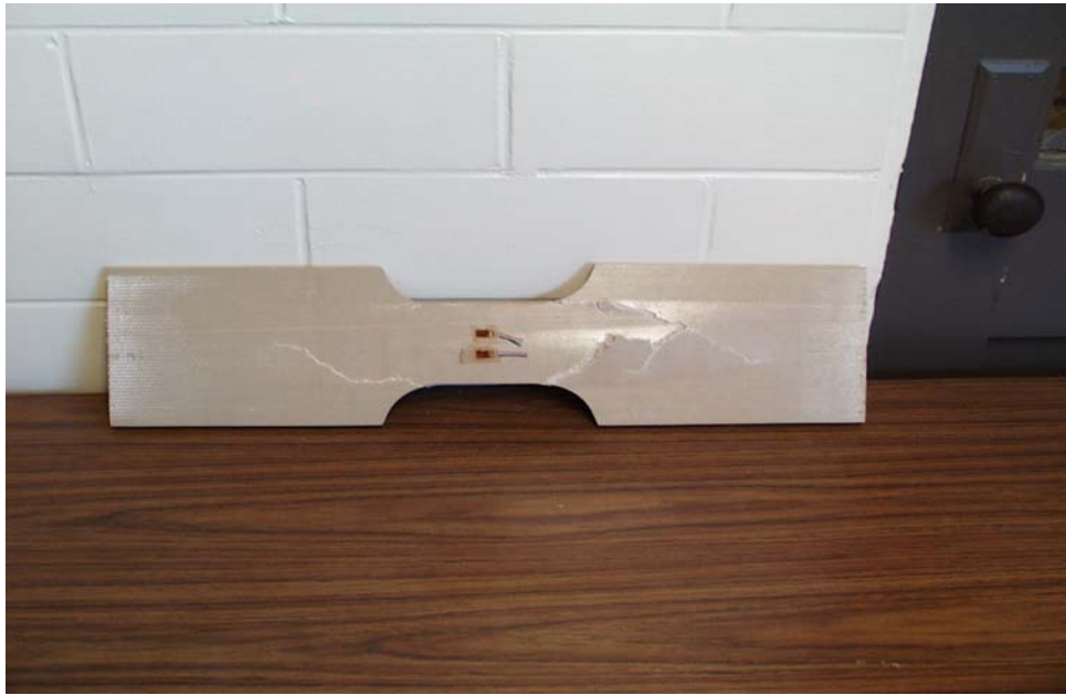
Figure 6.21. Tensile Test Coupon, Longitudinal Direction.
