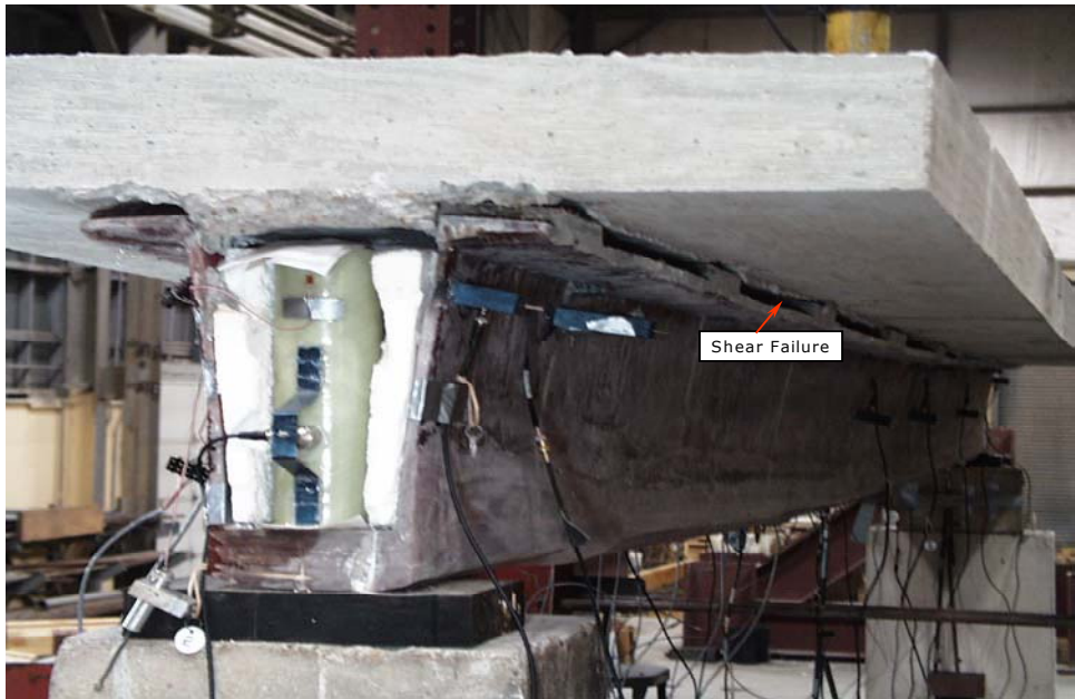
Figure 8.17. Shear Failure at Deck-Girder Interface at South End.
