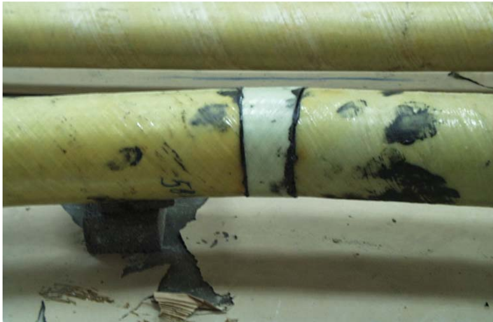
Figure 9.6. Assembled Connection Type 1 Prior to Final Wrap.
