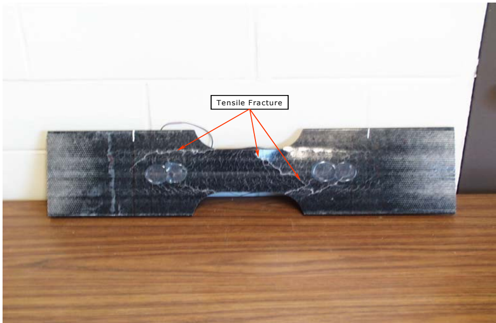
Figure 7.25. Specimen SW2 Tensile Coupon After Test.
