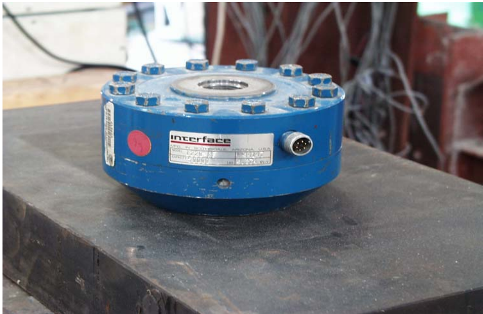
Figure 3.5. Load Cell, Capacity 50 kips.
