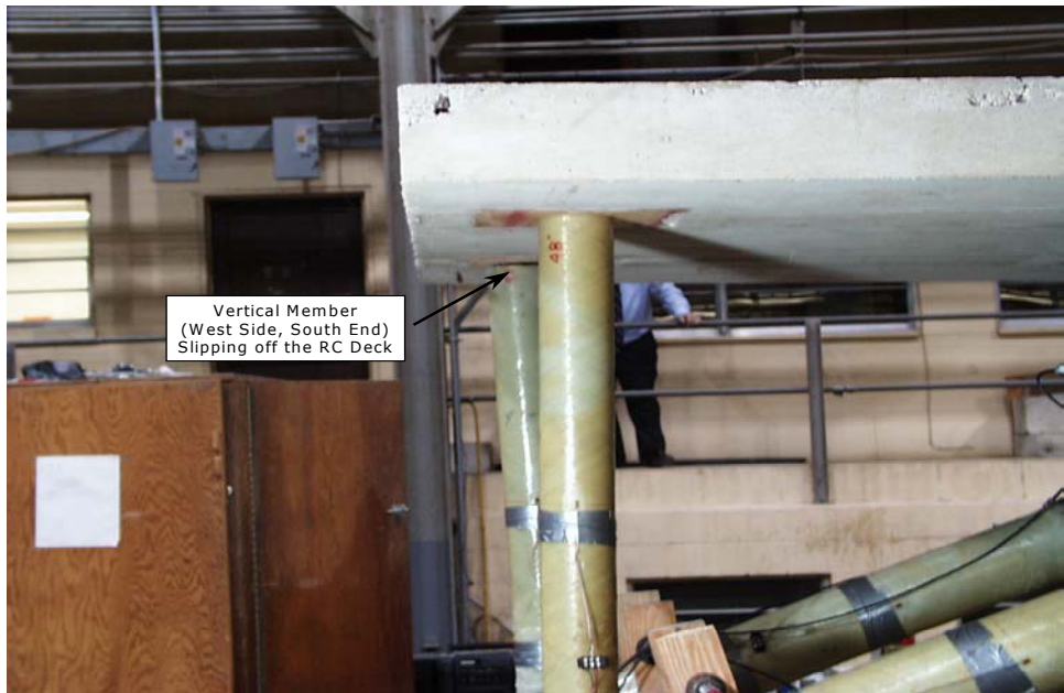
Figure 9.33. Slippage of Vertical Member at South End of East Arch.
