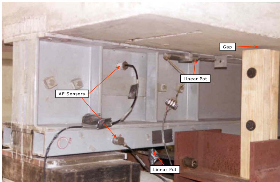
Figure 4.28. Instrumentation, Linear Potentiometer, AE Sensors.
