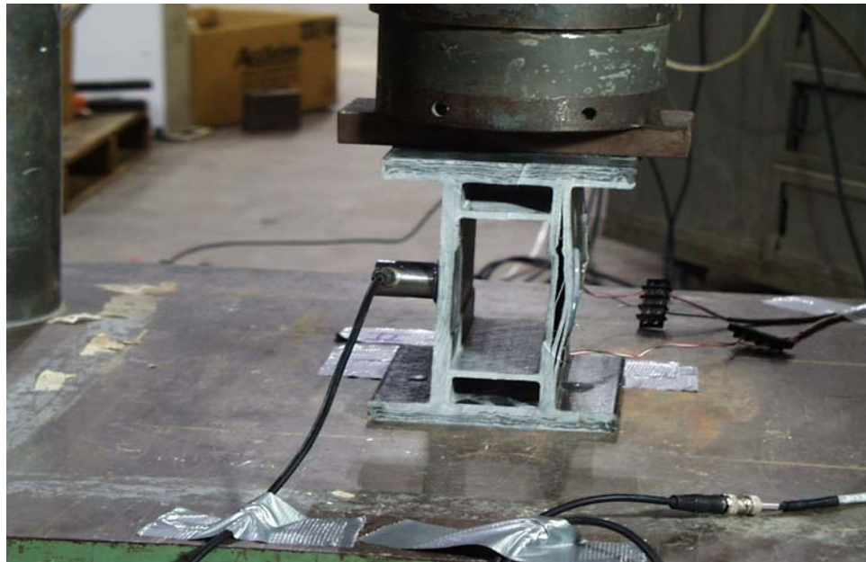
Figure 7.20. Specimen SW2 Web Buckling Test Failure.
