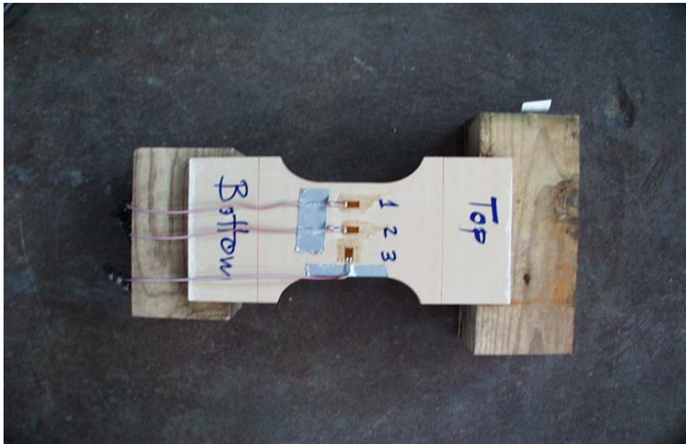
Figure 6.22. Tensile Test Coupon, Transverse Direction.
