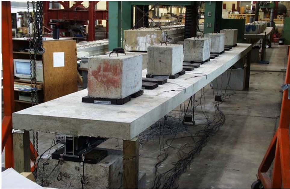
Figure 7.31. Specimen SW1 - First Level of Loading.
