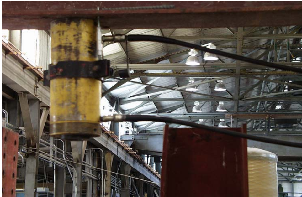
Figure 3.6. Hydraulic Jack and Hose System.
