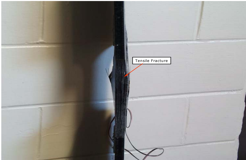
Figure 7.26. Specimen SW2 Tensile Coupon After Test (Side View).
