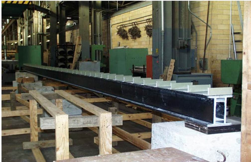
Figure 7.3. FRP Hybrid Girder and Shear Connectors.
