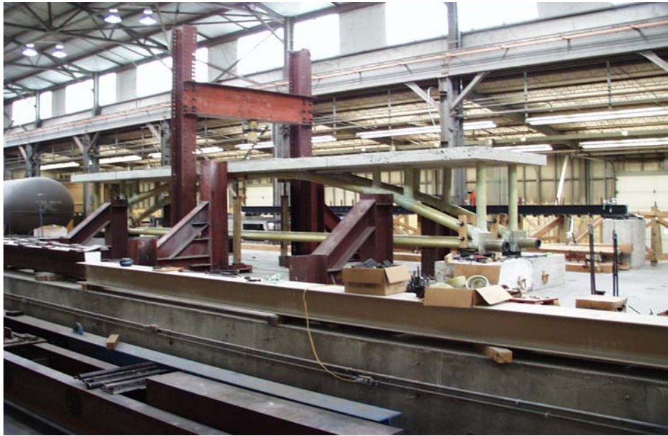
Figure 9.20. Specimen After Formwork Removal.
