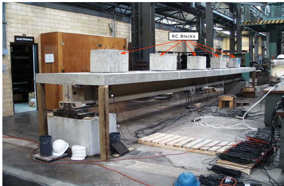
Figure 6.27. Specimen IKG1 - First Level of Loading.
