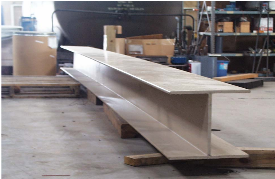
Figure 6.1. Original FRP Girder.
