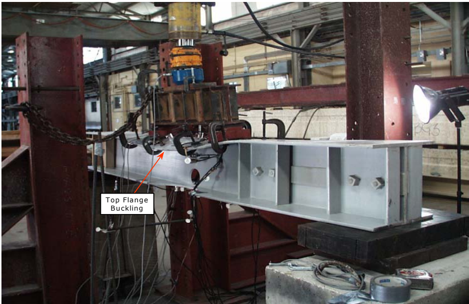
Figure 4.20. Buckling of Top Flange.
