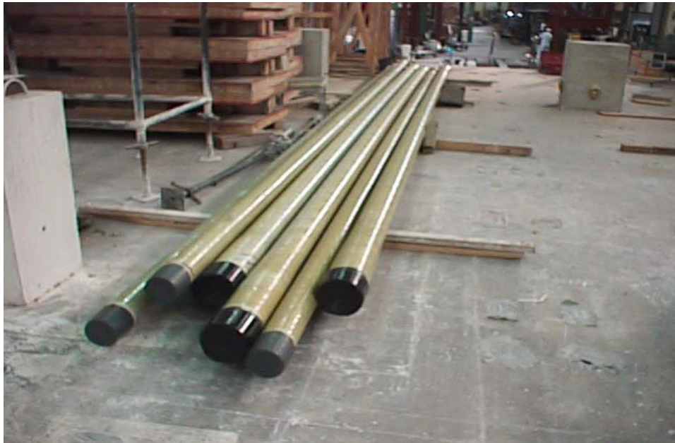
Figure 9.1. FRP Pipes (Downhole and Line types).
