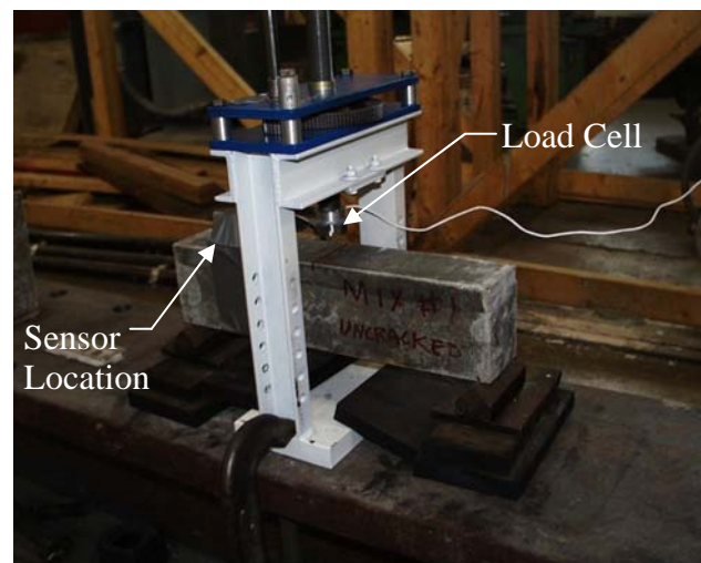
Figure 4.6- Experimental Setup Used for Plain Concrete Tests
