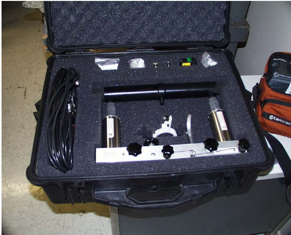
Figure 6.9 - Photo of DOCTOR Impact-Echo Equipment
