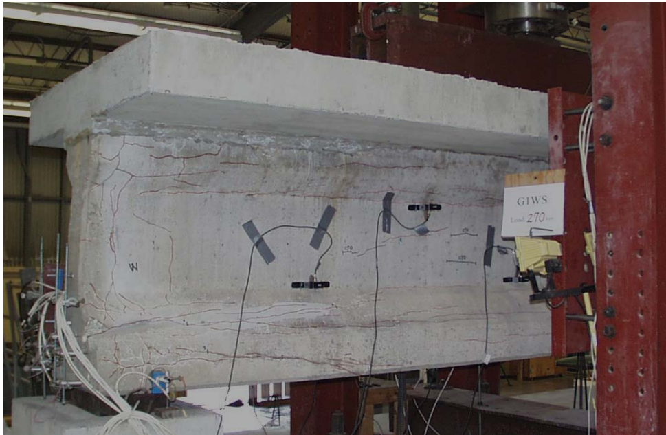
Figure 4.48 - G1WS under test at 270 kips
