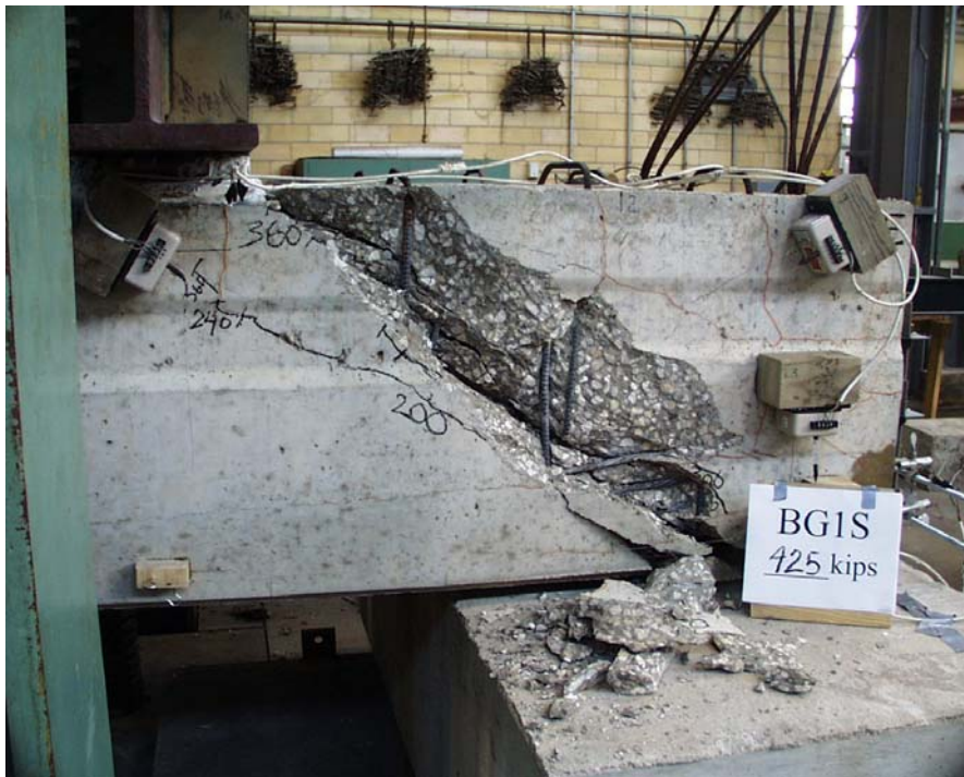
Figure 4.33 - Compression Strut Failure of BG1S
