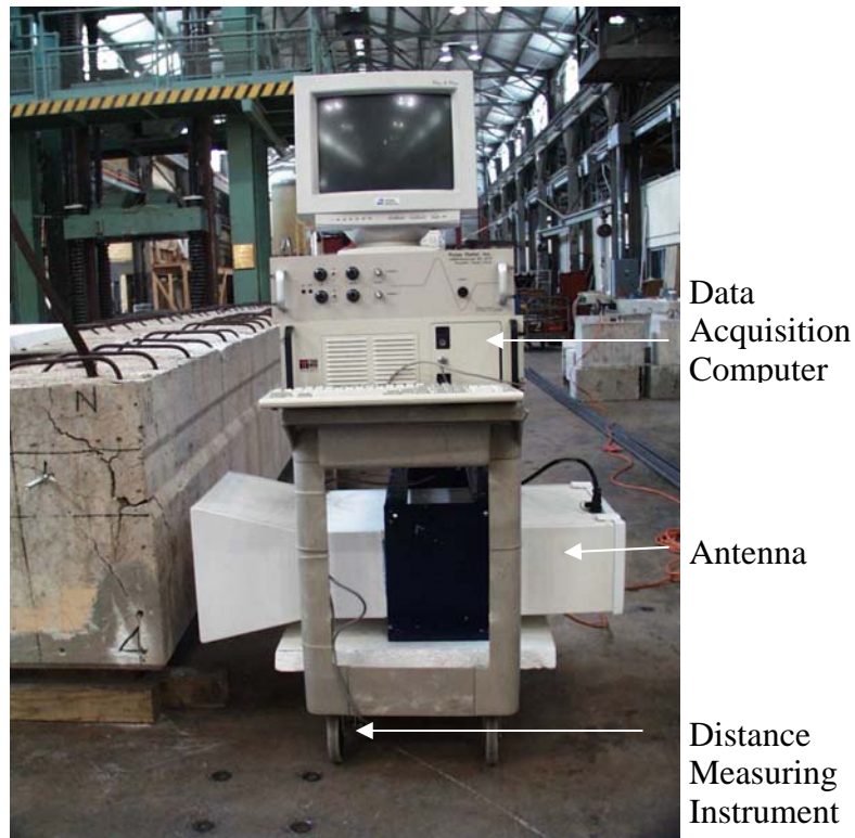
Figure 5.3 - Short Pulse Radar Equipment
