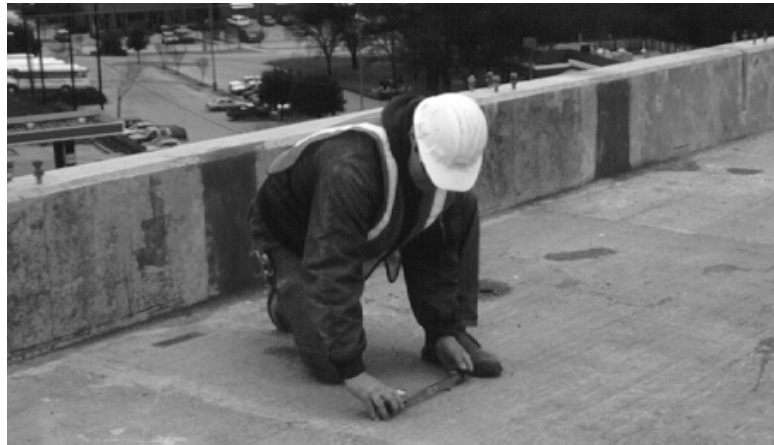
Figure 3.19 - A researcher takes measurements from Demec points installed on the deck of RampP
