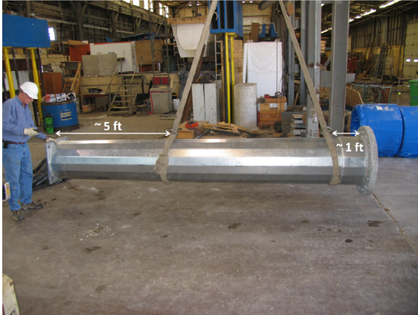
Figure A2 Lifting High Mast Specimen
