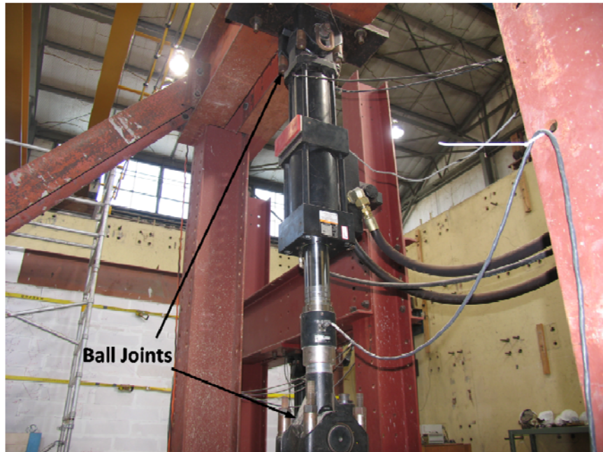
Figure 2.4 MTS 55 kip Hydraulic Actuator
