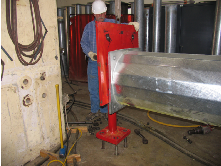
Figure A5 Replacing Pinned-End Support
