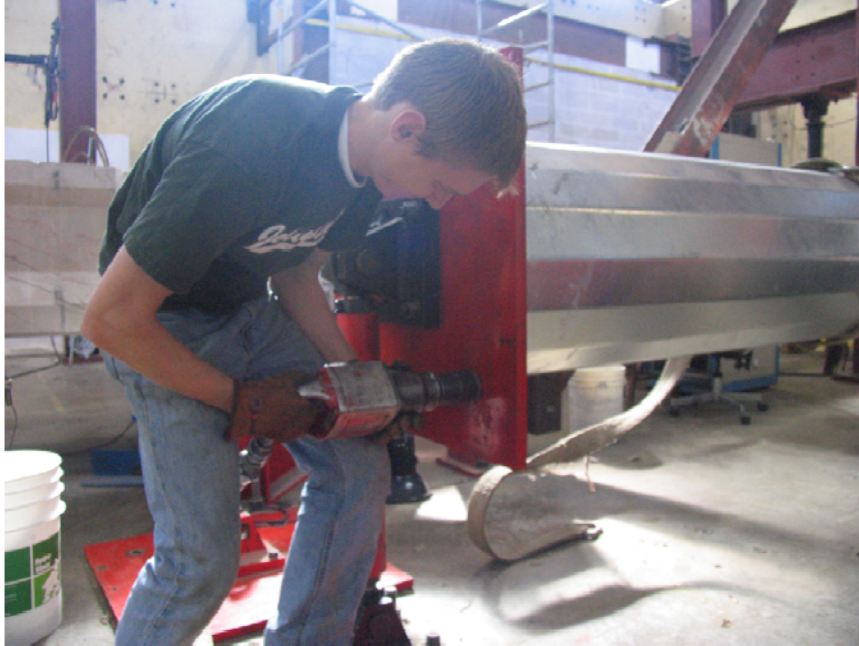
Figure A6 Tightening with Pneumatic Impact Wrench
