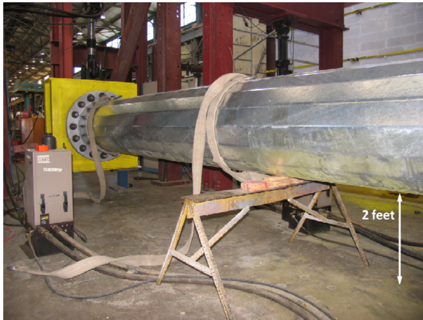
Figure A4 Temporary Saw Horse Support
