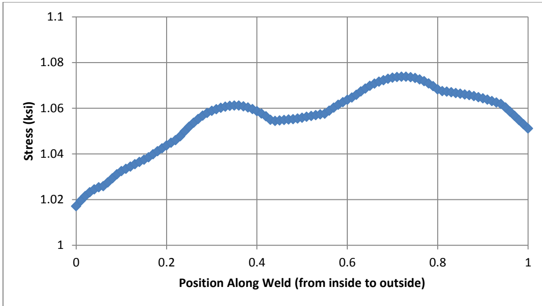
Figure 5-7: The stress along the weld of a plate stiffener that has been skewed 10 degrees (values taken \frac{1}{2} flange thickness from weld)
