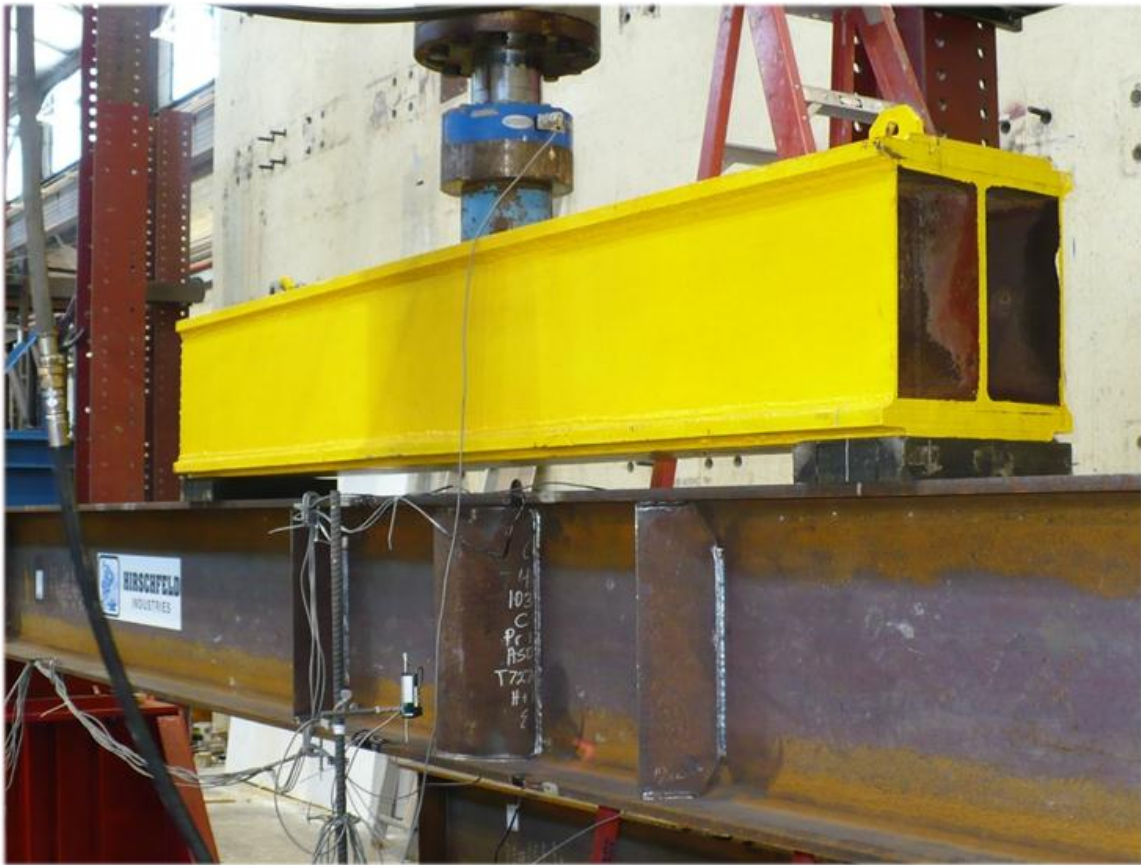
Figure 2-12: Application of Load to Specimen
