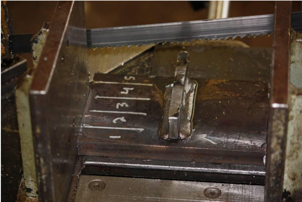
Figure 3-2: A piece of the beam that is to be tested for fatigue cracks is cut into five, narrow sections using a band-saw (this is the perpendicular stiffener from beam 30A)
