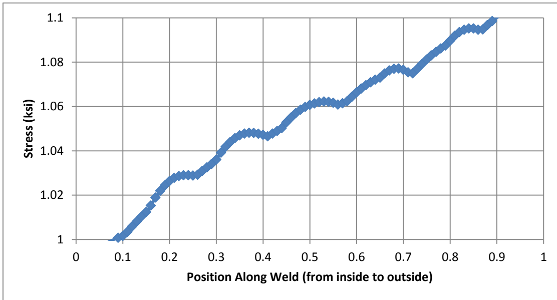
Figure 5-8: The stress along the weld of a plate stiffener that has been skewed 25 degrees (values taken \frac{1}{2} flange thickness from weld)
