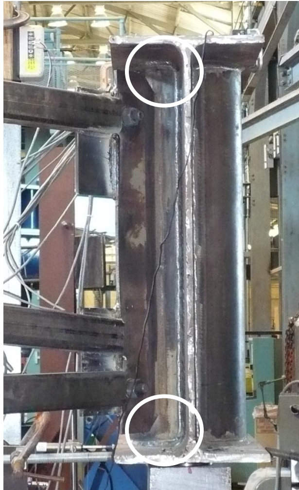
Figure 6-1: Connection of Cross-Frame to Half-Pipe Stiffener
