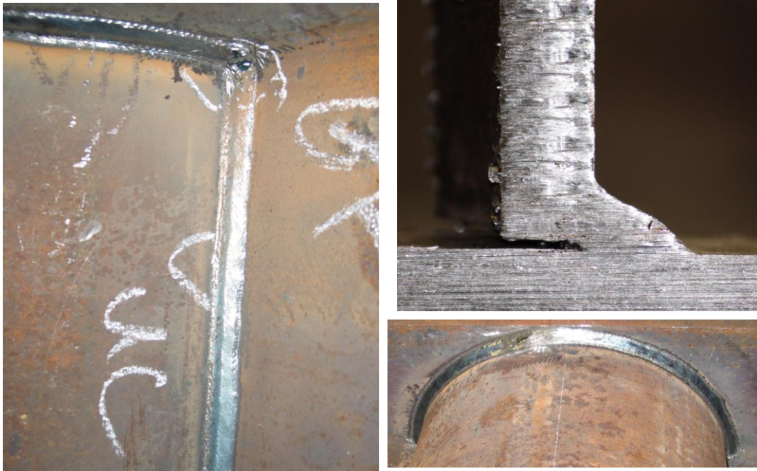
Figure 2-7: Welded Details for Half-Pipe
