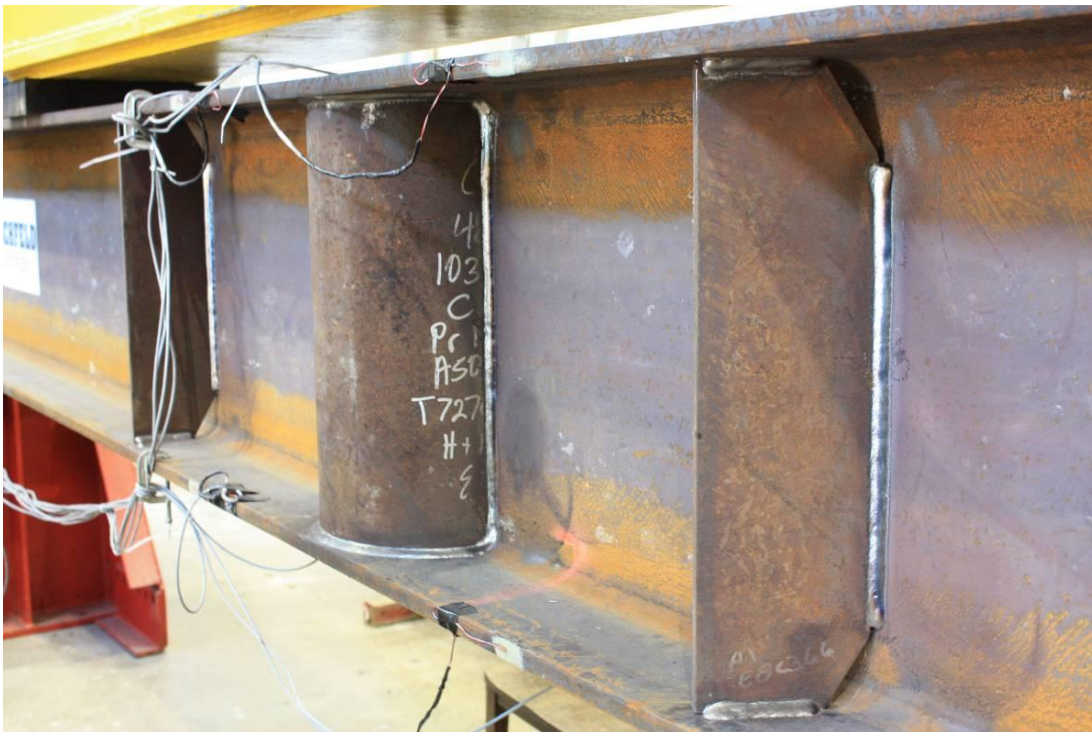
Figure 3-6: Beam 30A with two 30 degree stiffeners, two pipe stiffeners and two perpendicular stiffeners (only one side shown here, the reverse side is mirrored)
