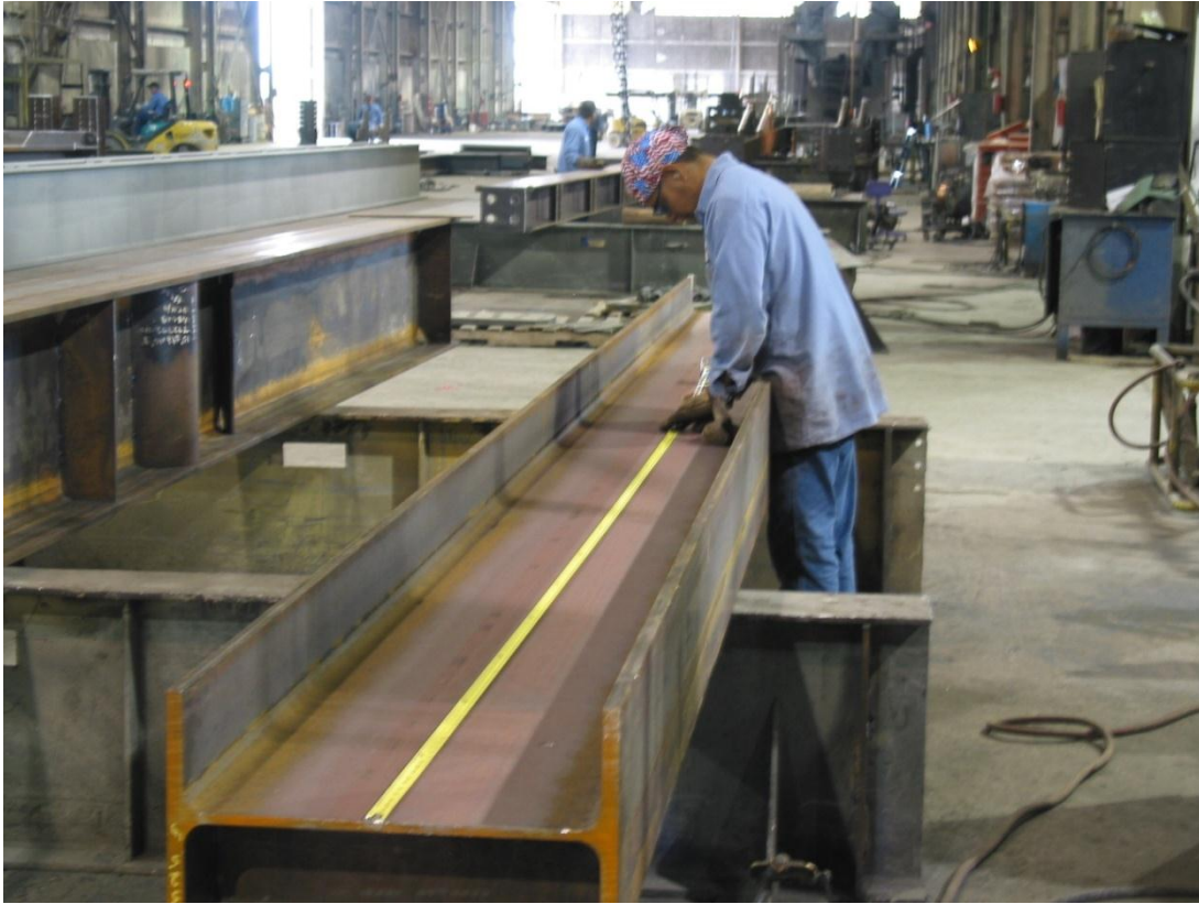
Figure 2-3: A Specimen Being Measured During Fabrication
