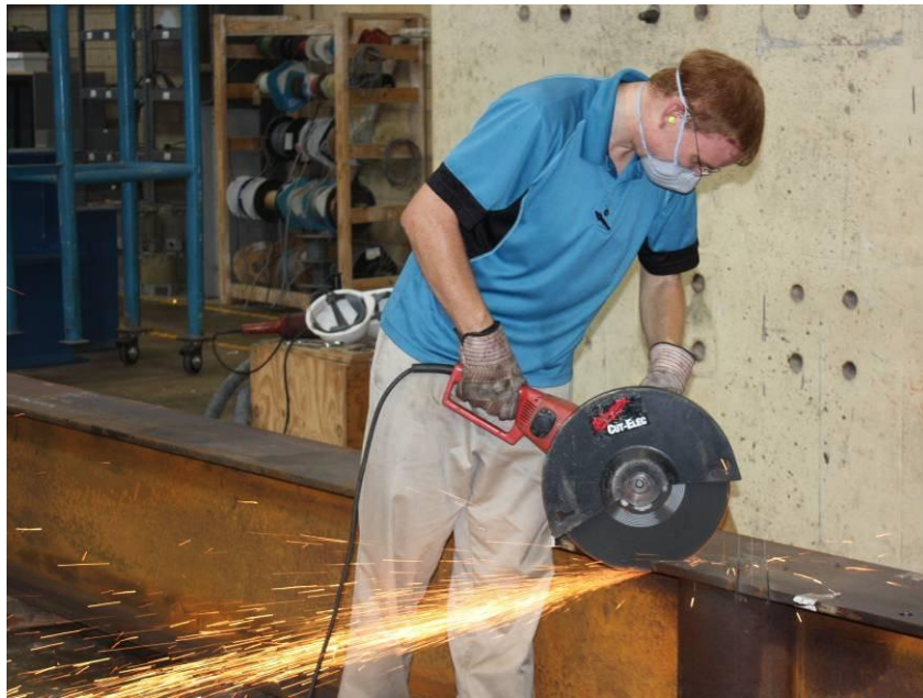
Figure 3-1: Using an abrasive saw to cut out sections of interest for destructive testing
