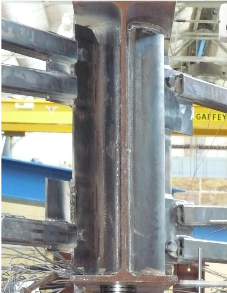
Figure 1-3: Half-Pipe Connection in Laboratory Tests at The University of Texas, Austin (Quadrato 2010)
