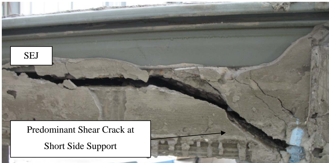
(a) Southeast Corner of Specimen P45P3 Viewed from Side
