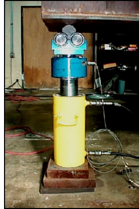
Figure 3.5 Load Ram, Load Cell, and Roller/Bearing Assembly
