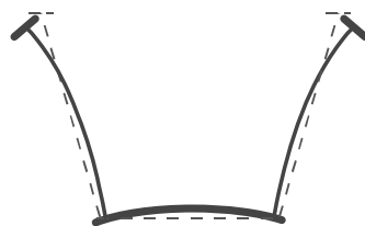
Figure 2.8 Cross-Section Distortion (Gilchrist, 1997)
