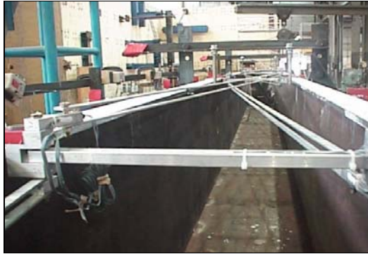
Figure 4.13 Bracing Taught Before Loading
