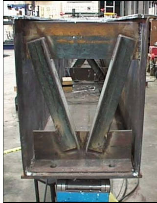
Figure 3.7 K-Brace at Location of Concentrated Load
