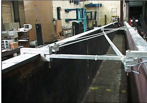
Figure 3.15 Original Brace, Coupler, and Flange Mount Connection
