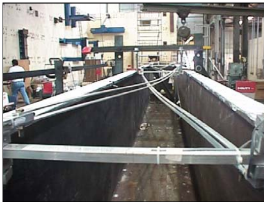
Figure 4.14 Bracing Slack During Initial Loading
