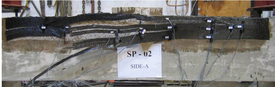
Figure 4.10 Failure mode of Specimen No.2, Side-A
