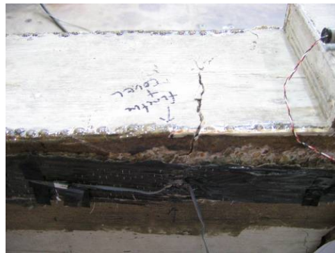
Figure 4.63 Failure Mode of Specimen No.7, Side-B, Concrete failure around CFRP Anchor
