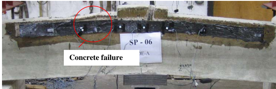
Figure 4.46 Failure Mode of Specimen No.6
