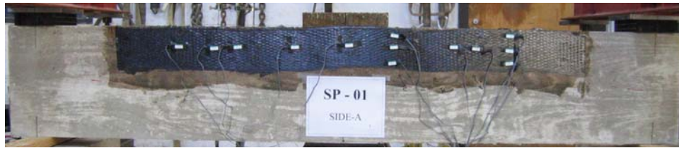
Figure 3.4 One Layer of CFRP sheet, 5.5 in. wide
