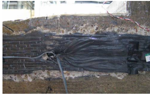
Figure 4.62 Failure Mode of Specimen No.7, Side-B, Fracture of CFRP Sheet
