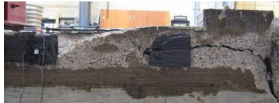
Figure 4.47 Failure Mode of Specimen No.6, After Cutting CFRP Sheet
