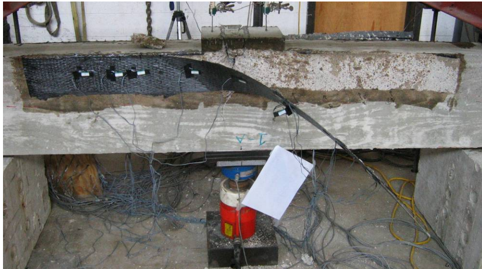
Figure 4.2 Failure mode of Specimen No.1, Delamination of CFRP Sheet
