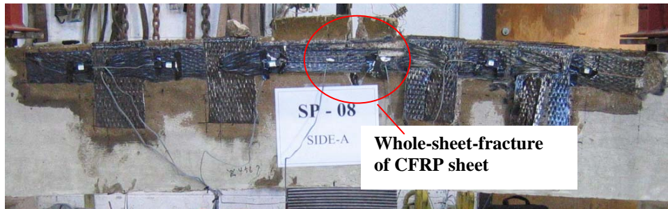
Figure 4.72 Failure Mode of Specimen No.8
