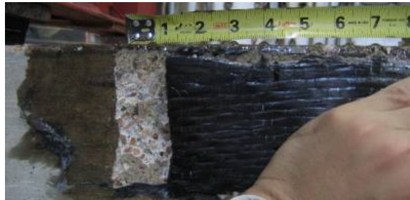
Figure 4.50 Slip of CFRP Sheet
