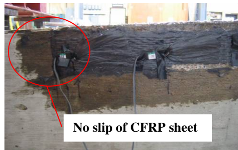
Figure 4.64 Slip Condition of CFRP Sheet
