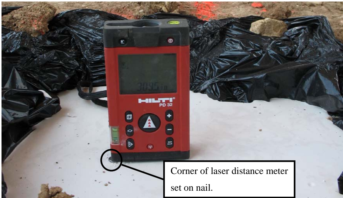
Figure 3-8 Deflection Laser Measurement from Isolated Base
