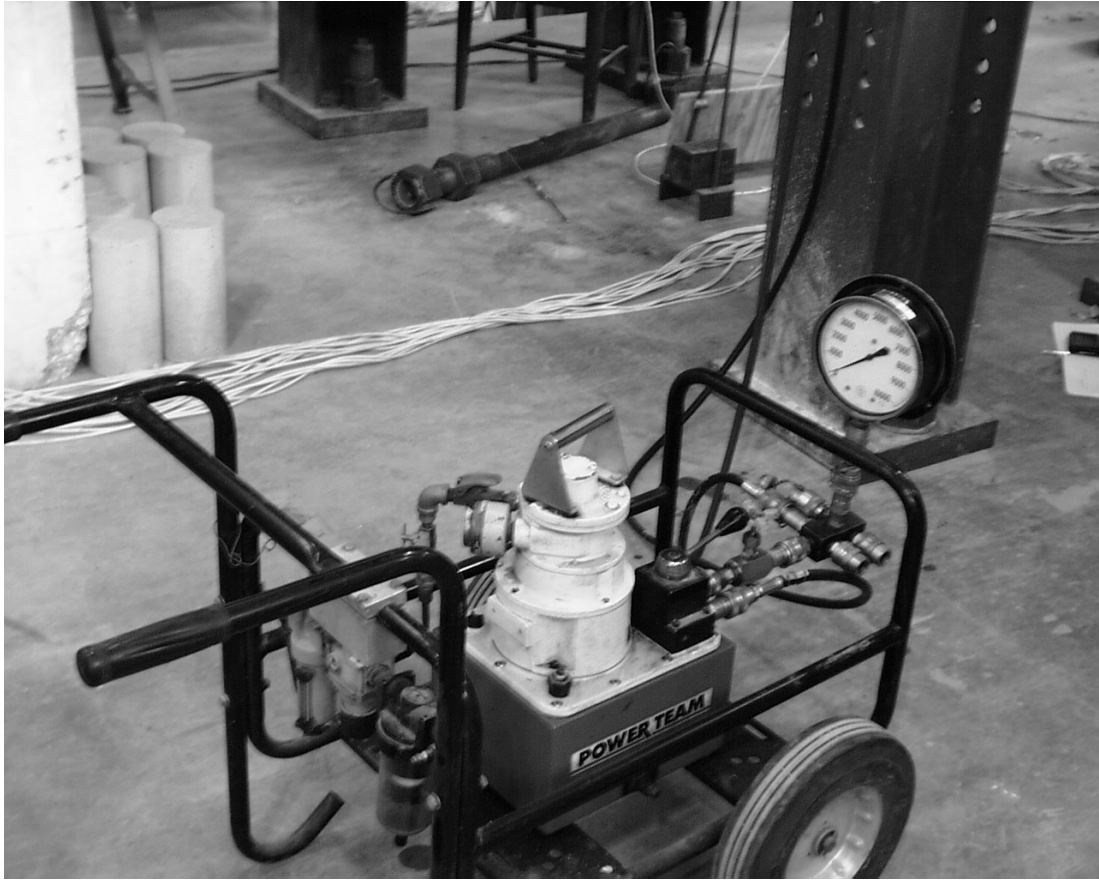
Figure 2.13 Hydraulic Pump and Pressure Gauge
