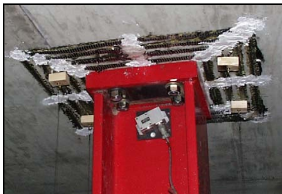
Figure 3.16 Upgrade B4 Slab-Column Connection
