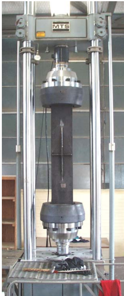
Figure 3-2: MTS Uniaxial Testing Machine with Specimen
