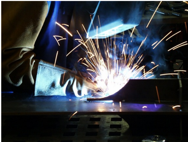
Figure 2-13: Welding the Web to the Flange
