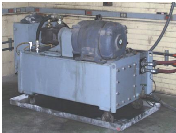
Figure 3-5: MTS Hydraulic Supply Unit
