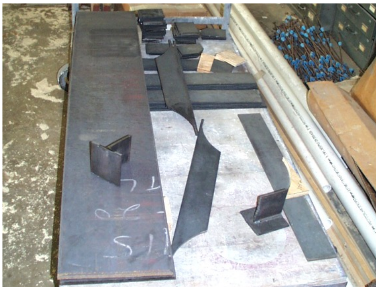
Figure 2-14: Steel Parts Prior to Welding
