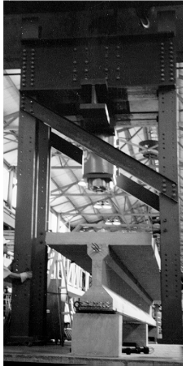
Figure 3.3 Movement of test frame by over head crane
