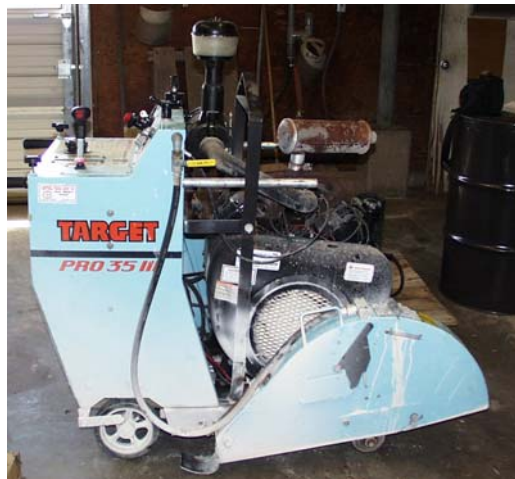
Figure 4.63 Concrete Saw Used in Autopsy
