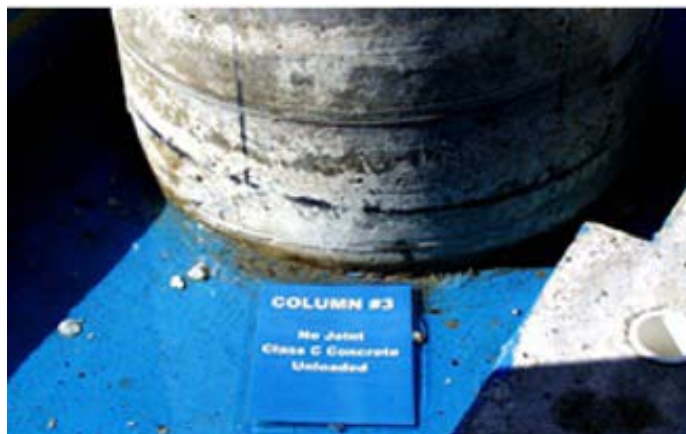
Figure 5.52 Condition of Specimen NJ-TC-N at the End of Testing
