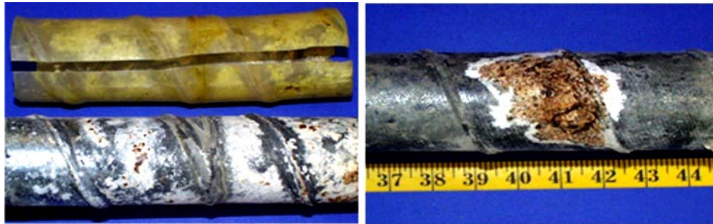
Figure 4.111 Specimen 2.6 – Duct Splices
