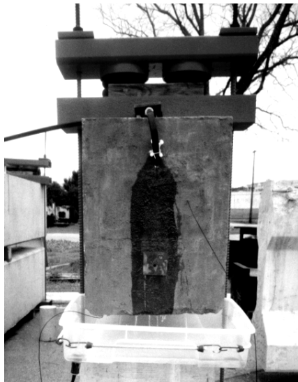
Figure 4.18 Beam End Dripper System 4.3
