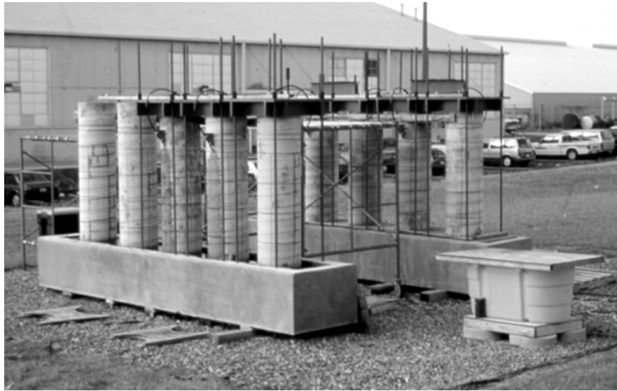
Figure 5.11 Column Corrosion Test Setup. 5.1
