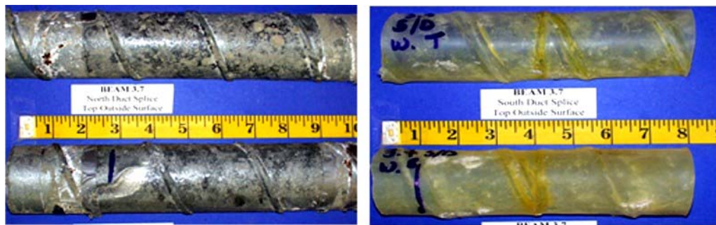
Figure 4.119 Specimen 3.7 – Duct Splices
