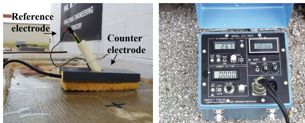
Figure 4.22 3LP Equipment and Setup
