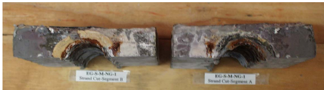
Figure 3.47 Incomplete Epoxy Coverage in Epoxy/Gasket Joint (EG-S-M-NG-1)
