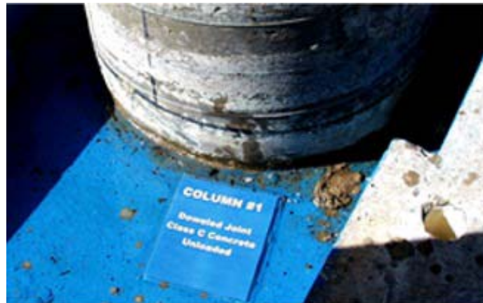
Figure 5.54 Condition of Specimen DJ-TC-N at the End of Testing
