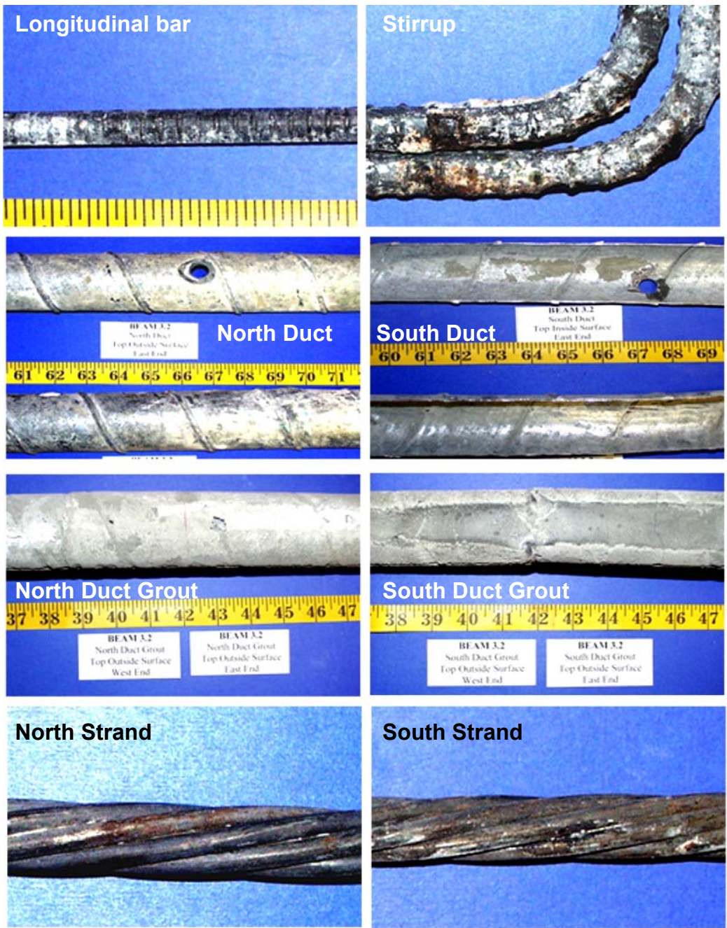
Figure 4.90 Specimen 3.2 – Reinforcing Elements
