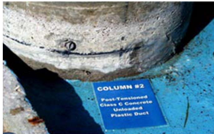
Figure 5.62 Condition of Specimen PT-TC-N-PD at the End of Testing
