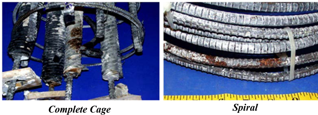
Figure 5.62 Condition of Specimen PT-TC-N-PD at the End of Testing
