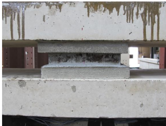
Figure 3-35 Grouted loading point
