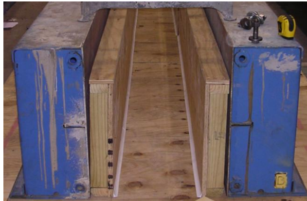
Figure 3-8 Side view of wooden panel inserts
