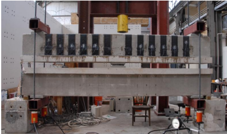
Figure 3-38 Initial loading test setup
