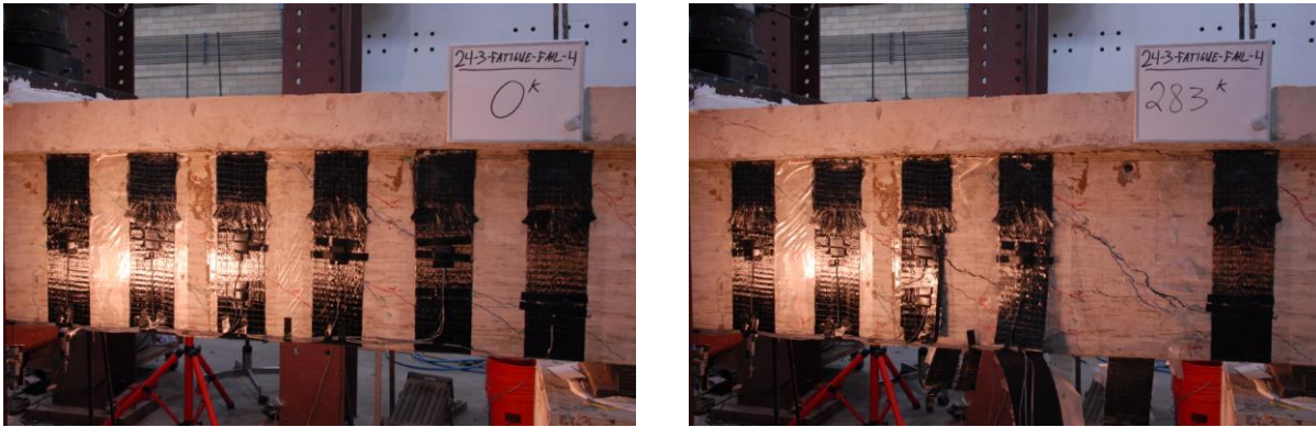
Figure 4-32 24-3-Fatigue-Fail-4 before (left) and after (right) loading
