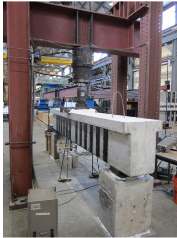
Figure 3-28 As-built fatigue load test setup
