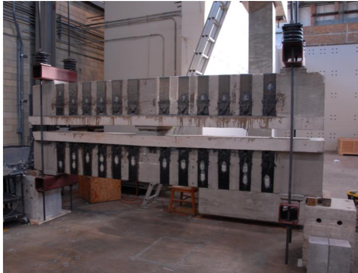
Figure 3-34 Sustained load test setup
