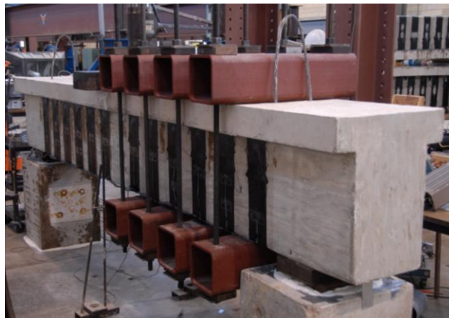
Figure 3-32 Prestressed external clamps
