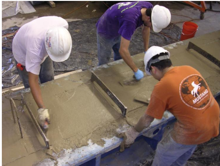
Figure 3-20 Hand screeding of specimen
