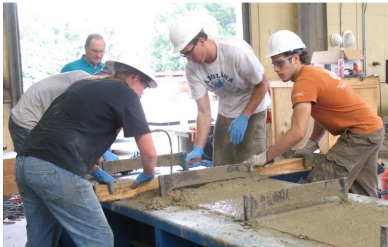
Figure 3-19 Screeding the top surface of the specimen
