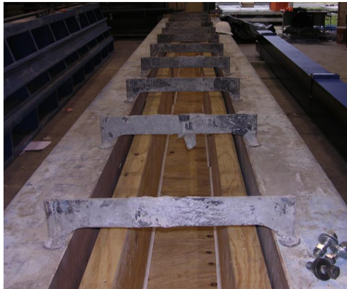
Figure 3-10 Steel cross ties
