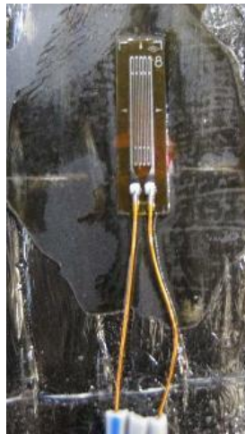
Figure 3-45 CFRP strain gauge (Pham, 2009)
