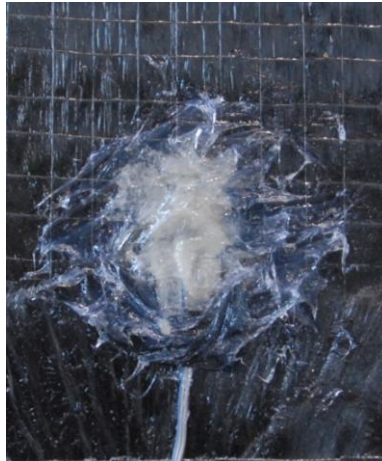
Figure 3-47 Long-term load gauge protection covering
