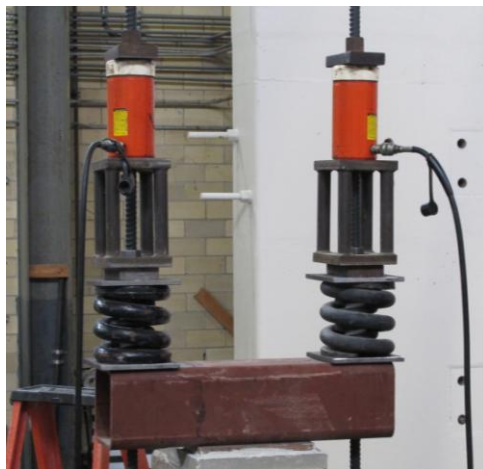
Figure 3-40 Hydraulic loading system for final loading
