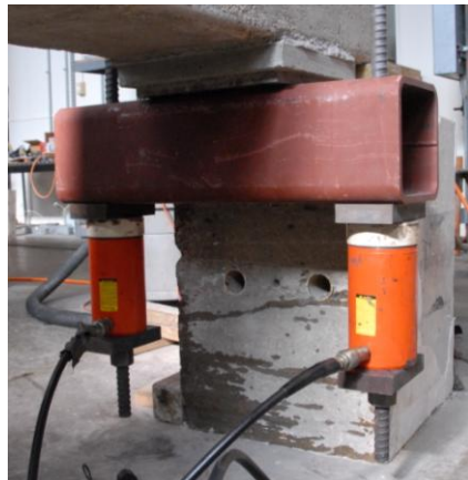
Figure 3-39 Hydraulic loading system for initial loading
