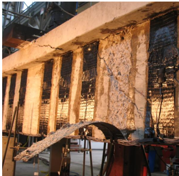
Figure 4-26 First CFRP anchor failure observed during 24-3-Fatigue-Fail-3
