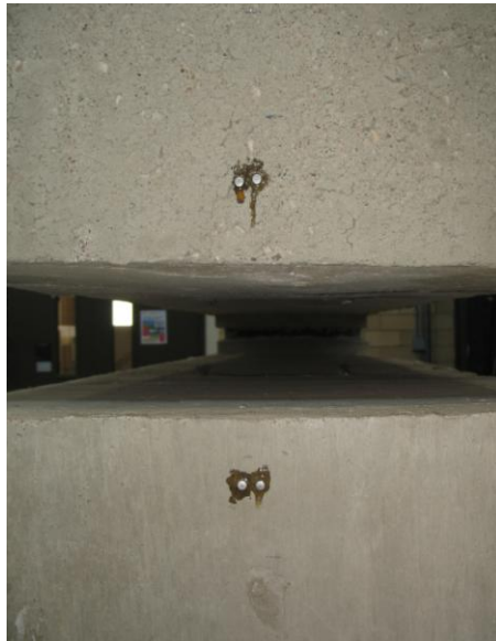
Figure 5-9 End displacement DEMEC points
