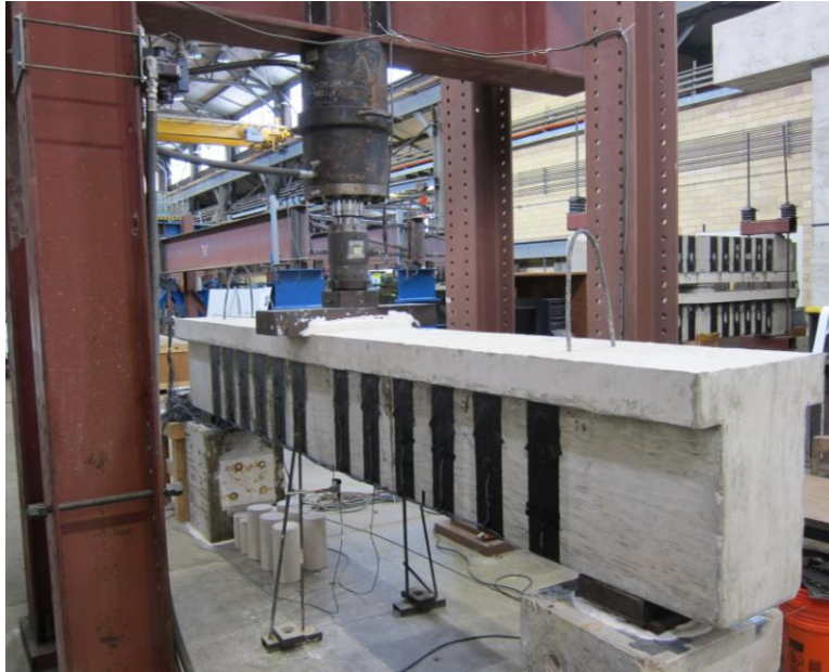
Figure 3-2 Fatigue load test setup
