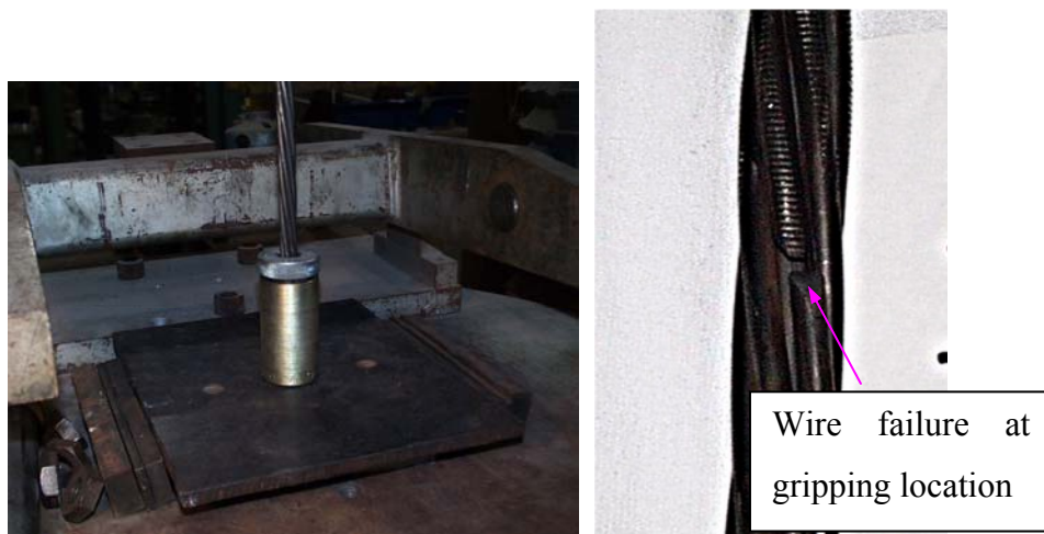
Figure 3.22 Photo of Barrel and Wedge Anchoring System (Chucks) (left); Photo of Failed Strand with Smooth Wires (right)
