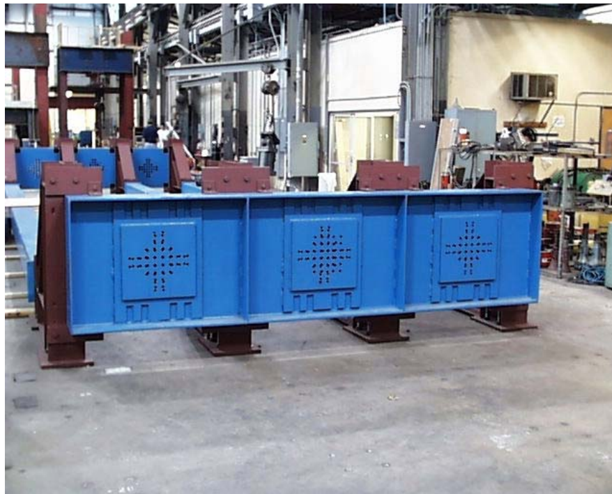
Figure 3.6 Steel Bulkheads for Strand Anchors
