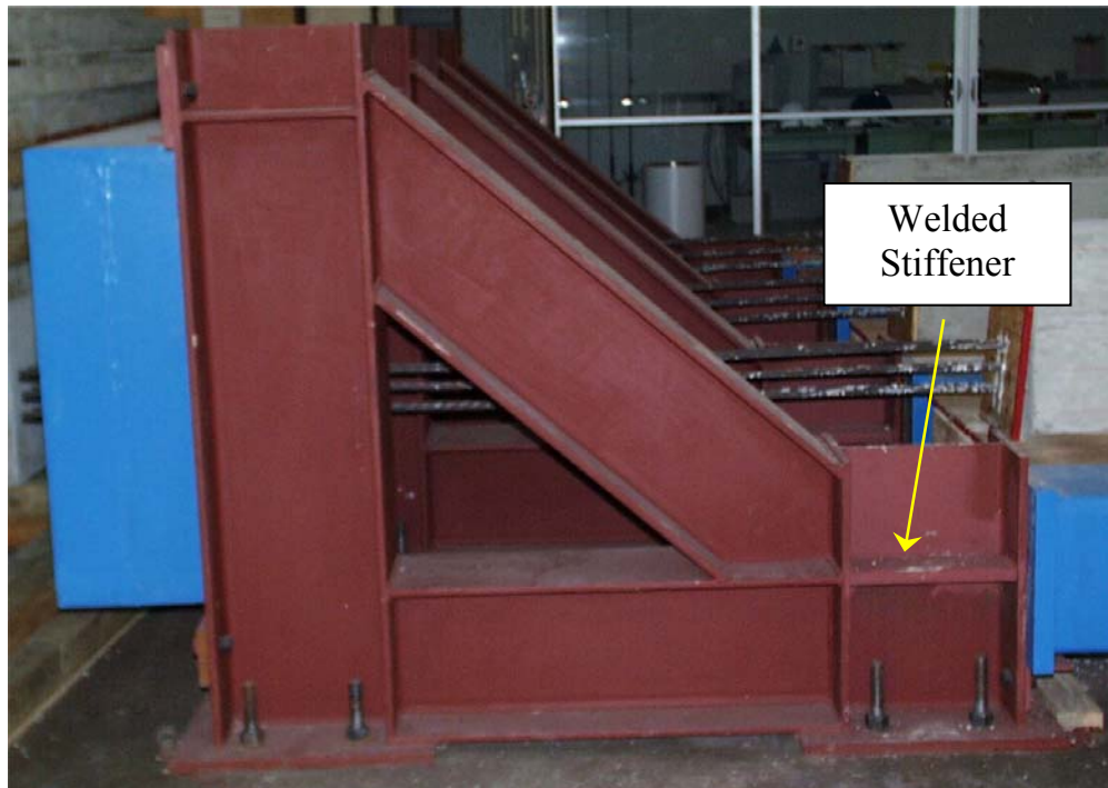
Figure 3.5 Photo of Modified Buttresses
