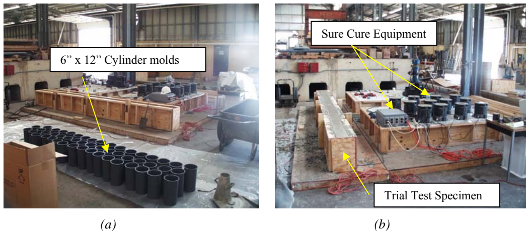
Figure 3.25 Compression Test Cylinder Molds (a); Trial Test specimen with Sure Cure Equipment (b)
