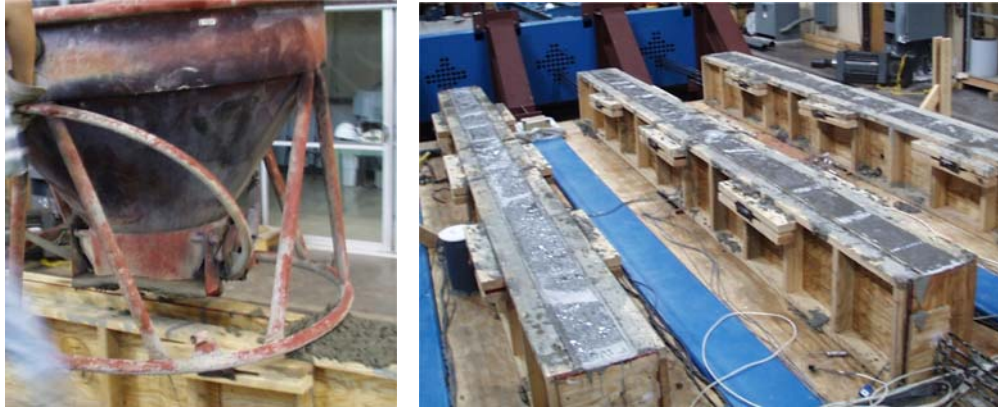
Figure 4.3 Casting of Test Specimens
