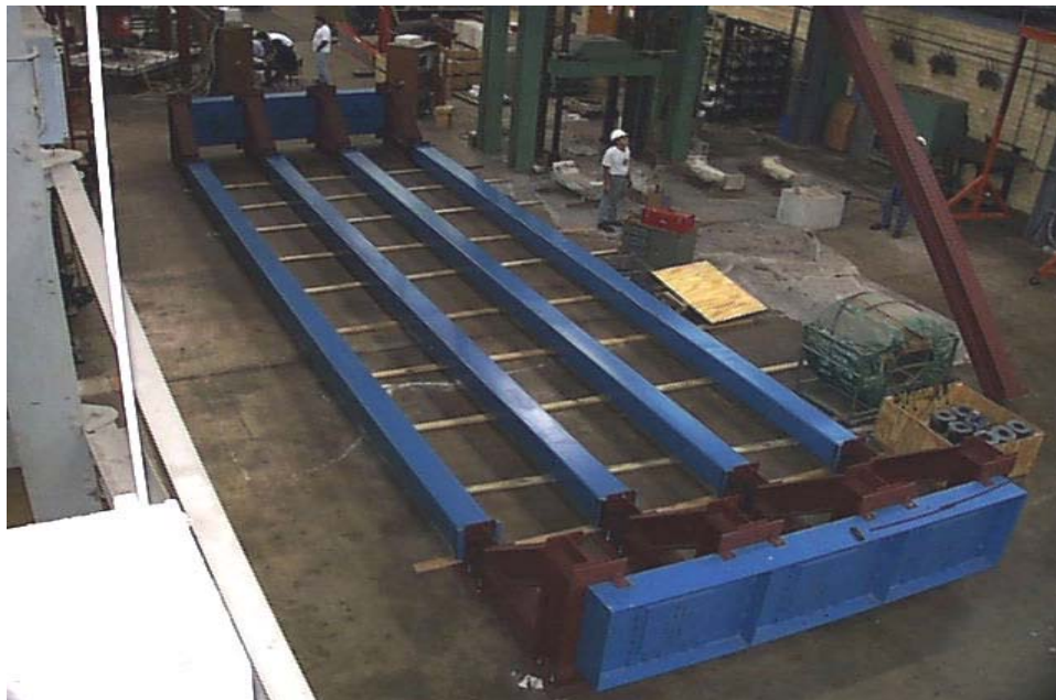
Figure 3.4 Photo of Modified Reaction Frame
