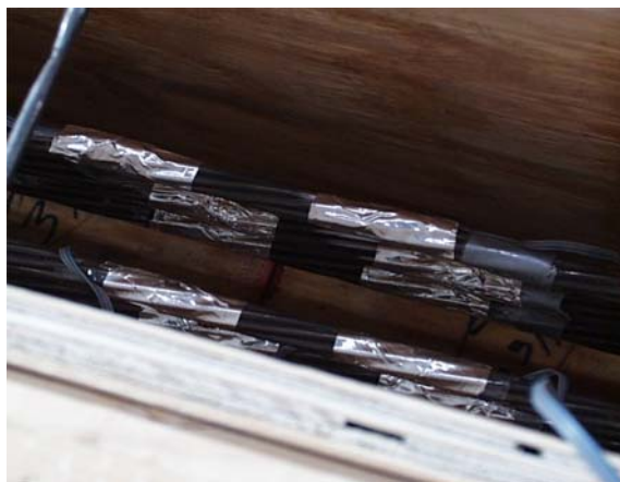
Figure 4.1 Instrumented Prestressing Strand for Test Specimen
