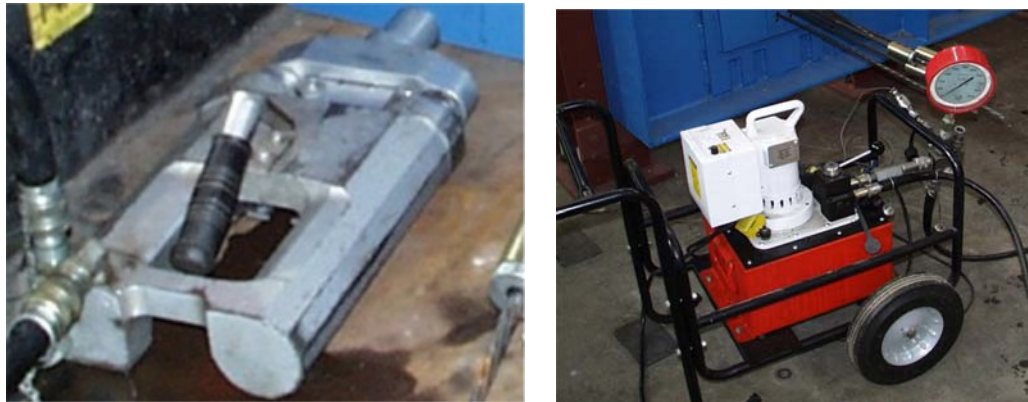
Figure 4.2 Single-Strand Prestressing Ram (left); Hydraulic Pump (right)
