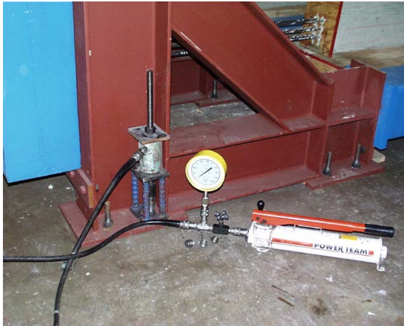
Figure 3.12 Post-Tensioning of Tie-Down Rods
