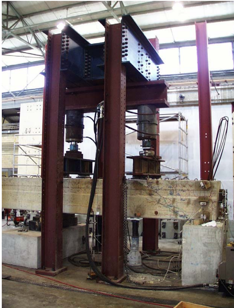
Figure 3.3 Loading setup for shear-dominated fatigue specimens
