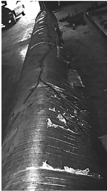
Figure 5.1 External Pressure Specimen after Testing
