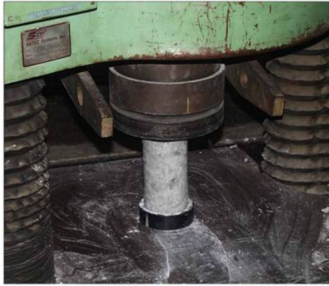
Figure 3.6 ASTM C39 Standard test method for determining the compressive strength of concrete.
