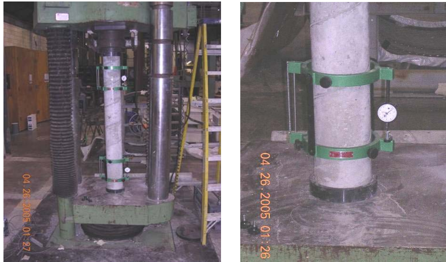
Figure 3.9 6x54-inch cylinder. Modulus of Elasticity measured at top and bottom in accordance with ASTM C469
