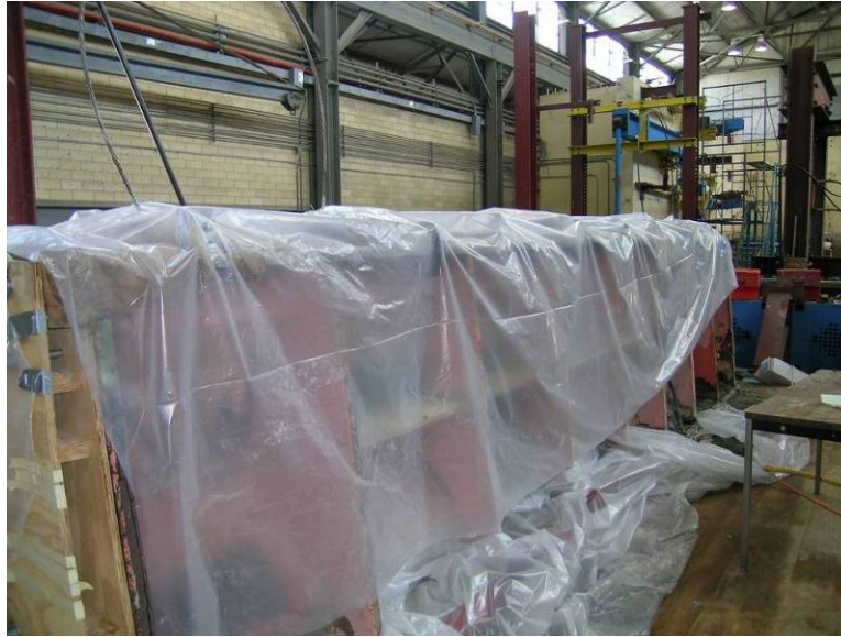
Figure 3.30 Beam specimens were cured by covering with wet burlap and plastic.
