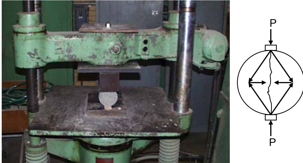
Figure 3.7 ASTM C496 Standard test method for determining the splitting tensile strength of concrete.
