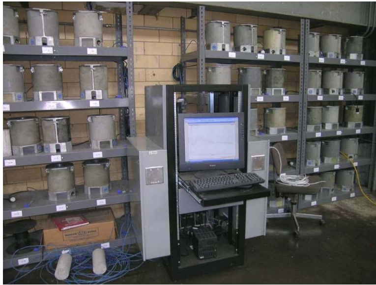
Figure 3.11 Electronic match-curing controller and insulated cylinder molds.
