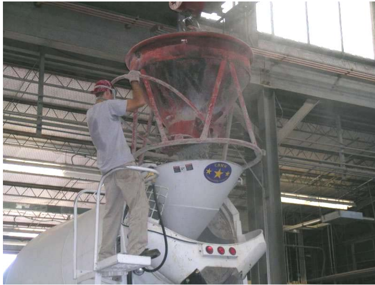
Figure 3.27 Type III cement being added to a ready mix truck.
