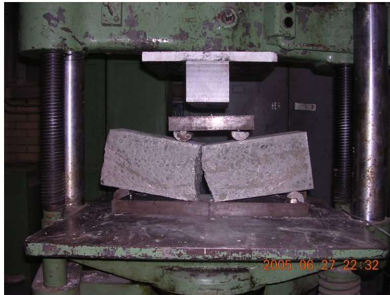
Figure 3.8 ASTM C78 Standard test method for determining the flexural strength of concrete.
