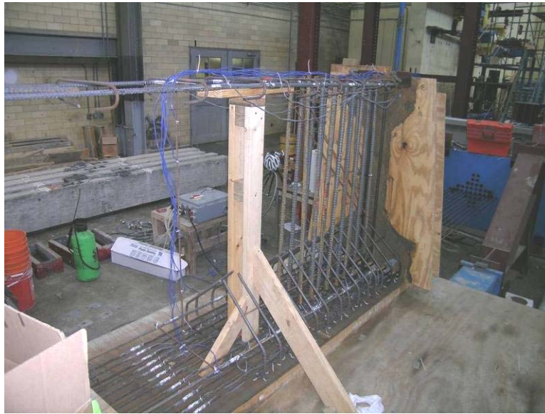
Figure 3.24 End of specimen illustrating gauge locations.
