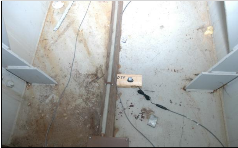
Figure 3.26 Typical accelerometer setup at the US-290E Direct Connector Bridge.
