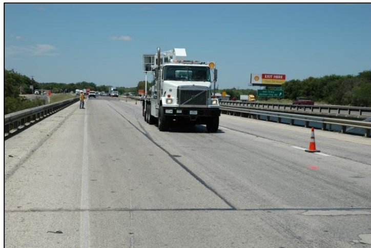
Figure 6.1 Snooper truck live load test (63 mph) conducted in July 2011.
