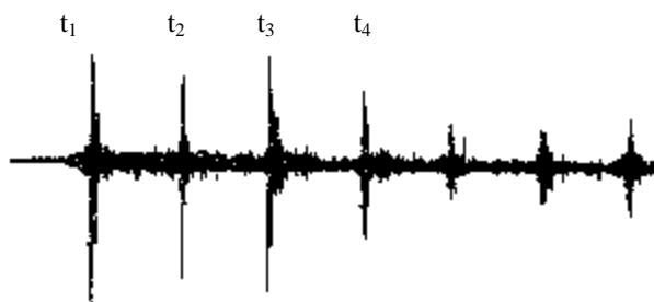
Figure 2.30 – Waveform of Multiple Arrivals Due to Different Propagation Paths [Yoon et al., 1990]
