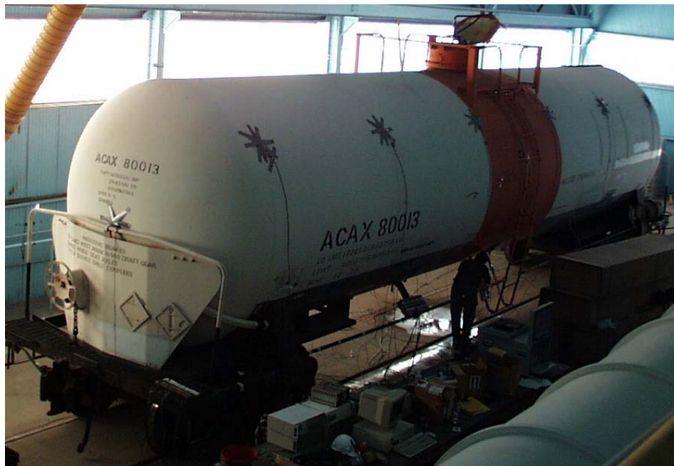
Figure 3.40 – Hydrogen Fluoride Tank Car
