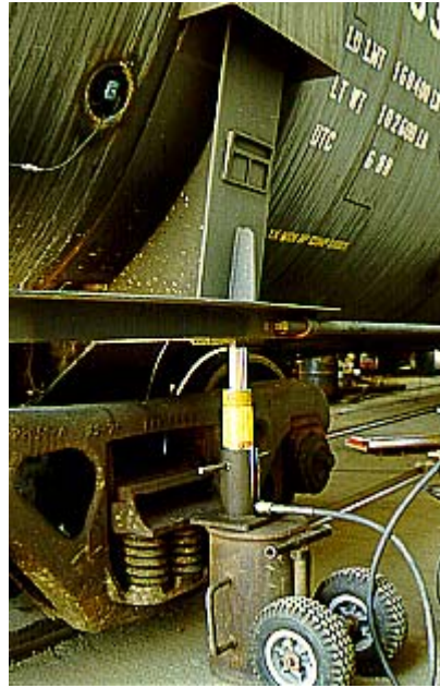
Figure 4.11 – Jacking Test Setup
