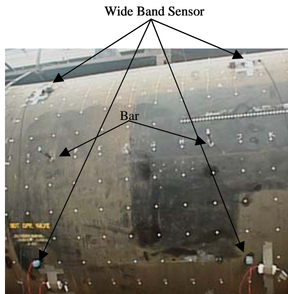
Figure 3.34 - Test Setup for Multiple Sources Study
