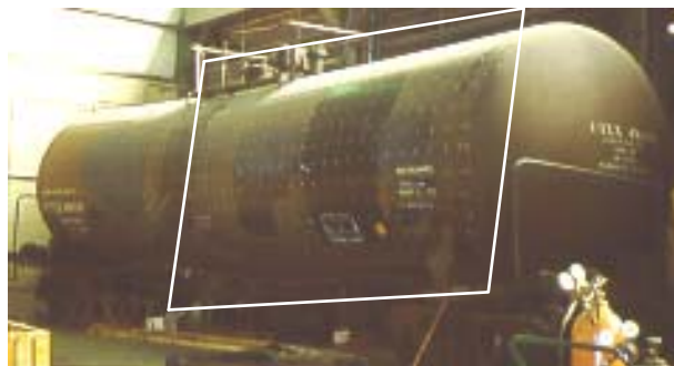
Figure 3.7 – Area of Tank Car Used for Source Location Studies
