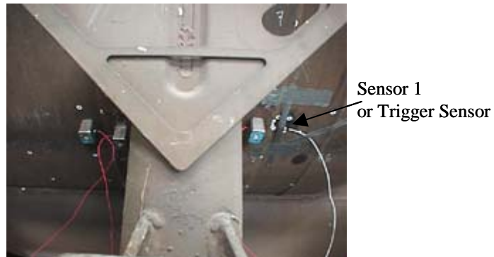
Figure 3.27 – Test Setup for a Wave Propagation Study around the Bolster
