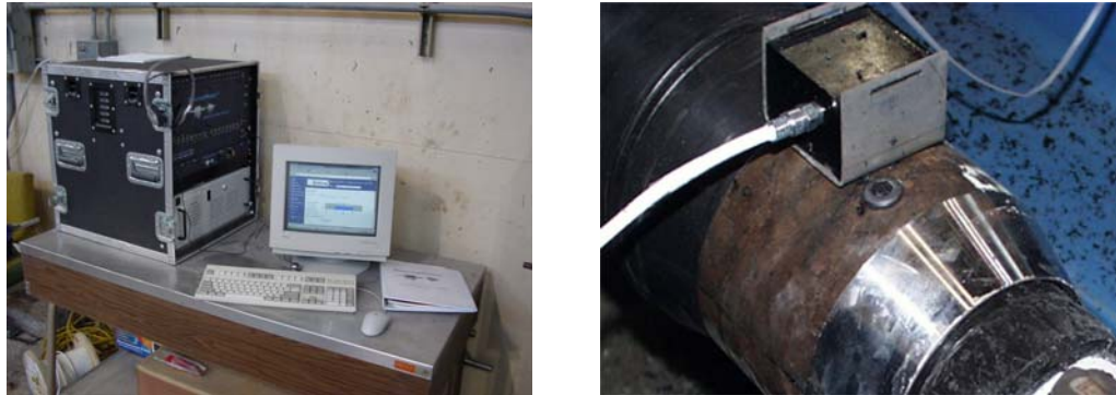
Figure 3-33: Soundprint Instrumentation and Acoustic Sensor
