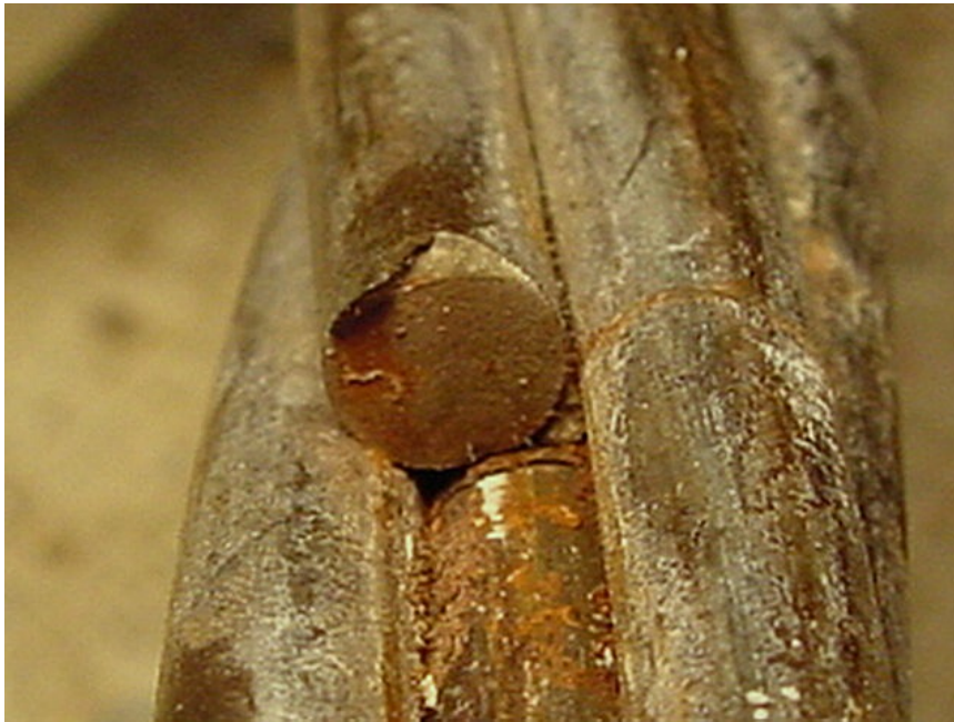
Figure 4-34: Fracture Surface – Specimen #2
