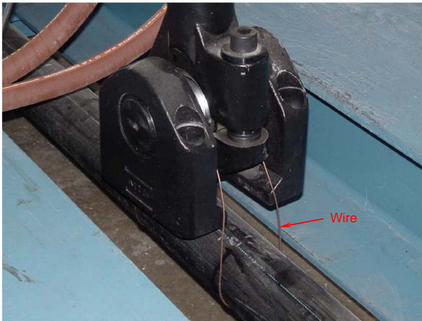
Figure 4-42: General Setup for a Pluck Test
