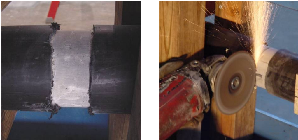
Figure 4-1: Cutting of the Specimen
