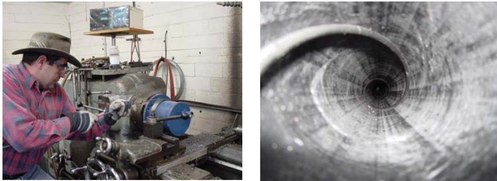
Figure 3-17: Helical Spacer Wire – Manufacturing and Inside the PE Pipe
