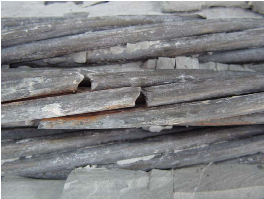
Figure 4-23: Wire Breaks – Strand #1 – Loading Point – Specimen #1
