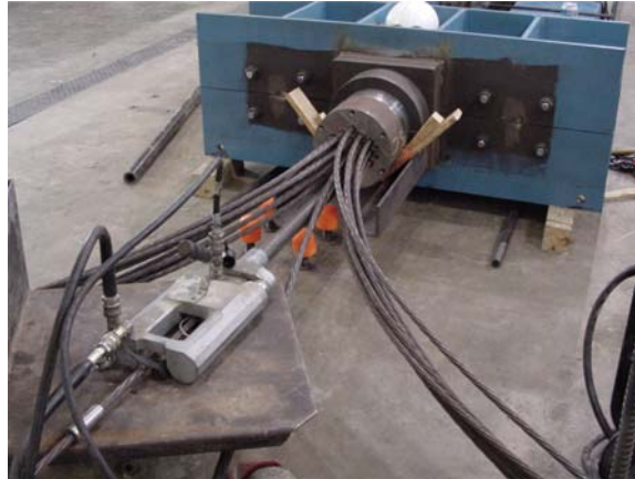
Figure 3-22: Mono-Strand Ram Stressing
