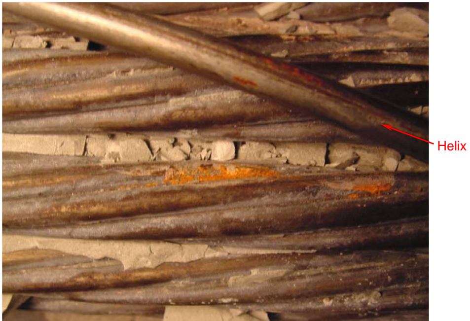
Figure 4-12: Localized Corrosion on Strand and Helix – Specimen #2
