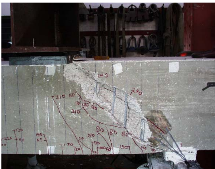
Figure 3.4 Failure of test specimen 4
