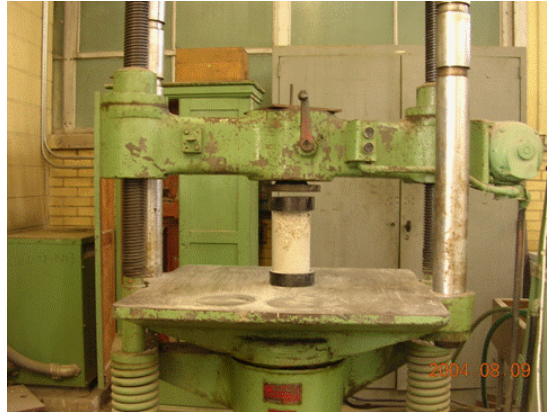
Figure 2.9 Testing of compressive strength of concrete
