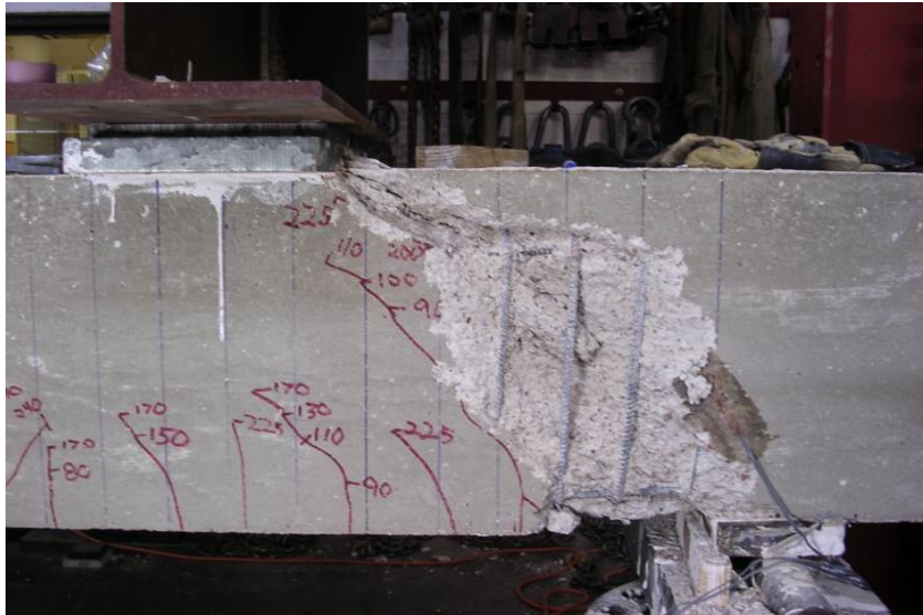
Figure 3.5 Failure of test specimen 5
