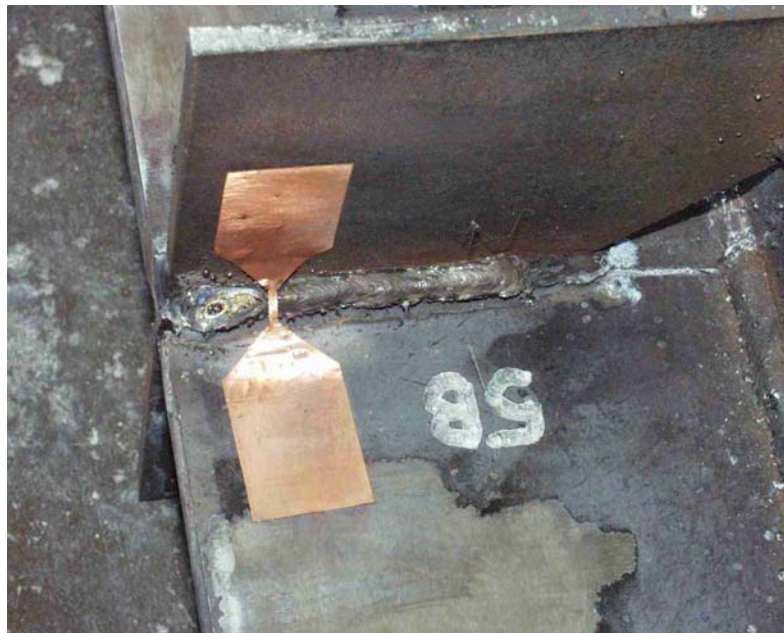
Figure 4.5 1/16-in. Wide Copper Shape over Crack, Top View
