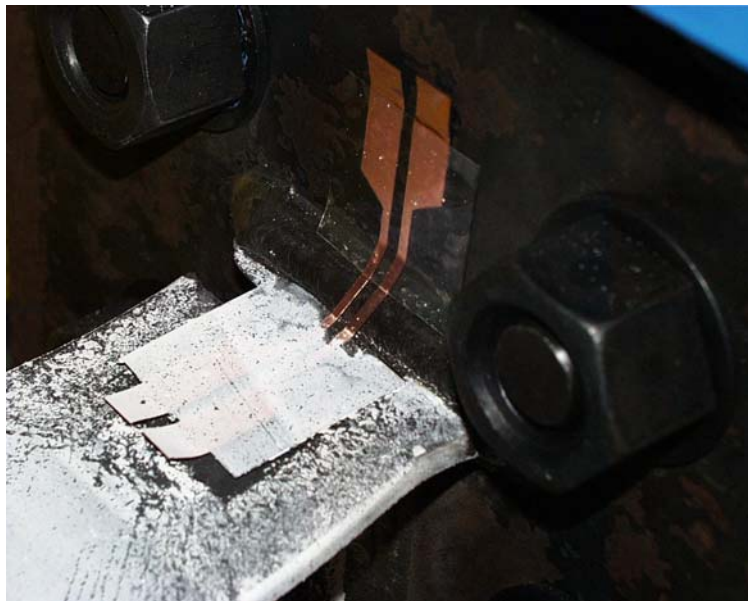
Figure 4.15 Point Switch after Beam Flange Failed Near Top Flange Weld in First Shear Link Specimen
