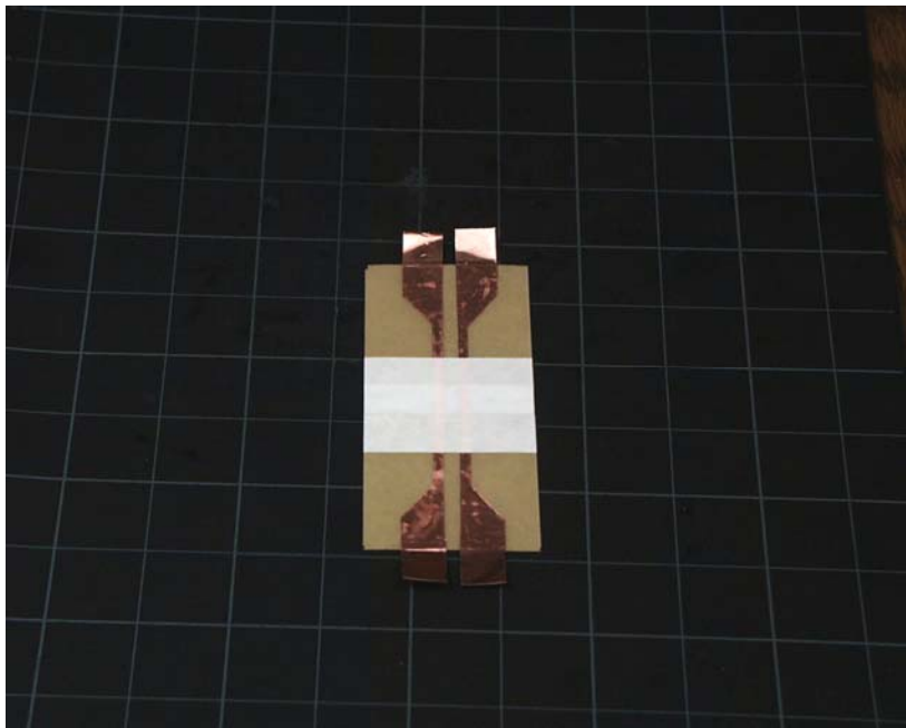
Figure A.20 Completed Point Switch
