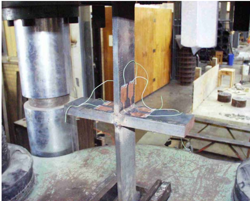
Figure 3.7 Installation of Copper Foil Shapes
