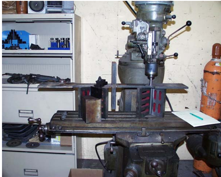
Figure 3.9 Cruciform Mounted on Milling Machine
