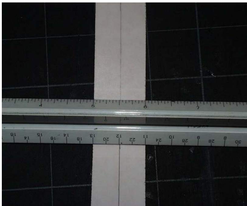
Figure A.9 Defining Midsection of Copper Tape
