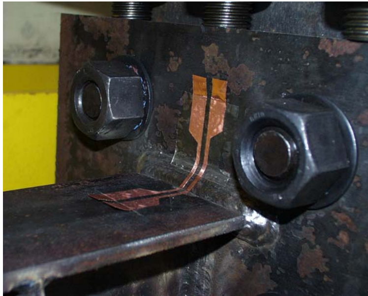
Figure 4.14 Point Switch with Minimal Surface Preparation in First Shear Link Specimen
