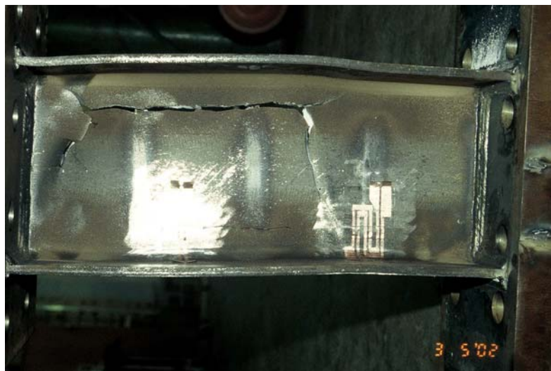
Figure 4.19 K-line Fracture on Web of Third Shear Link Specimen
