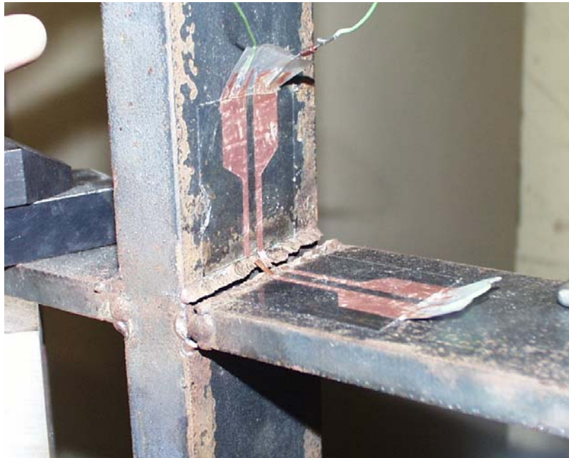
Figure 3.13 Failure of Point Switch Fabricated Using 3M Tapes
