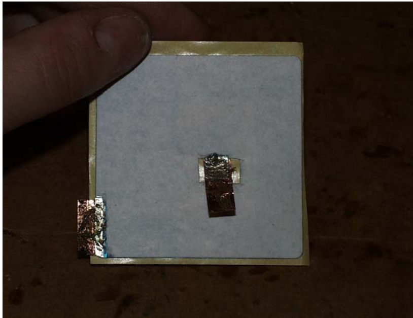
Figure A.5 Aluminum Solder Paste Applied to Copper and Aluminum
