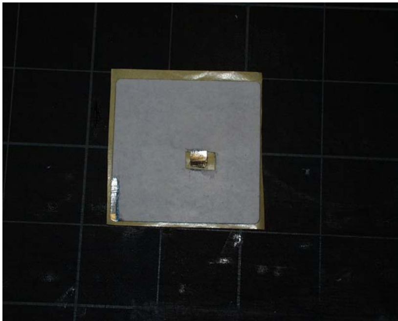
Figure A.3 EAS Tag with Aluminum Exposed
