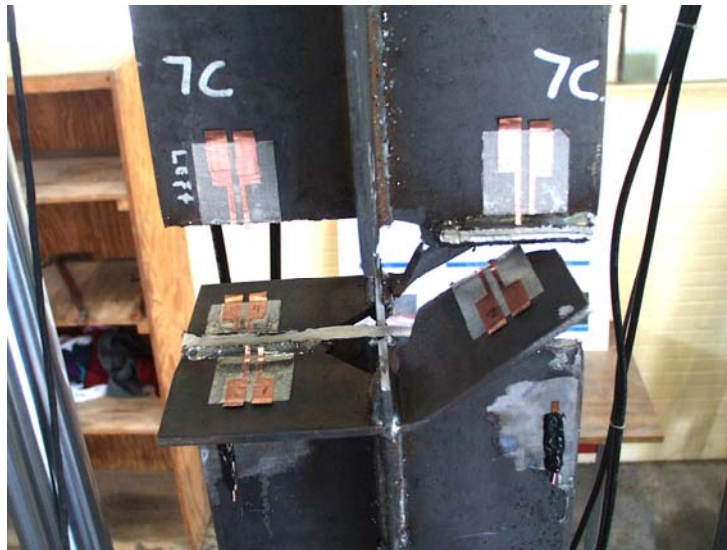
Figure 4.11 Test Specimen at Failure (Spadea, 2002)
