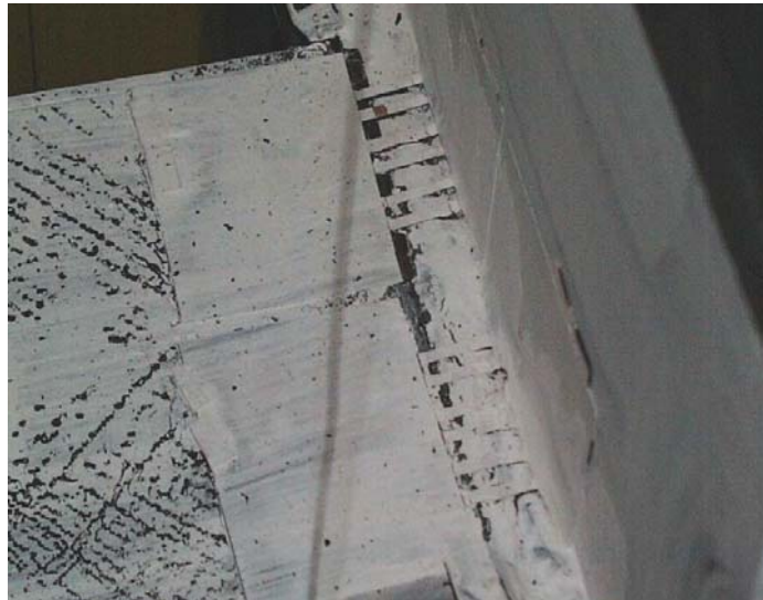
Figure 4.21 Distributed Switches Bridging a 1/10-in. Crack in Fourth Shear Link Specimen
