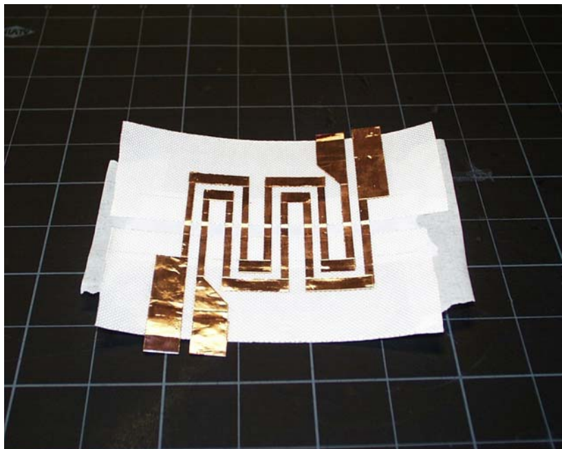
Figure A.37 Completed Transfer of Copper Strips to Carpet Tape
