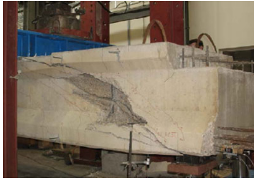
(b) Web crushing failure (Adopted from Hovell, et al. 2010)
