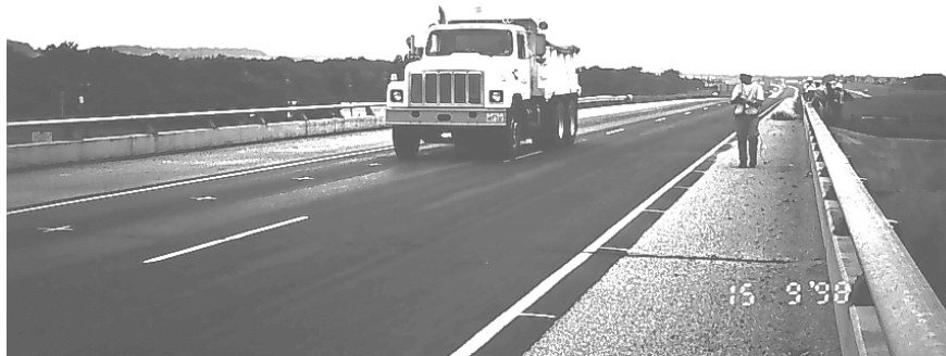
Figure 3.3 Photograph of a Ten Cubic-Yard Dump Truck Used for the Diagnostic Load Tests
