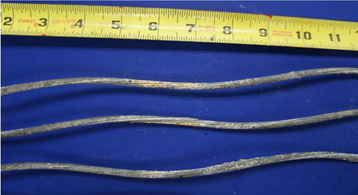
Figure 6.158: Pitting on the Outer Wires of One Strand from Specimen 7.3
