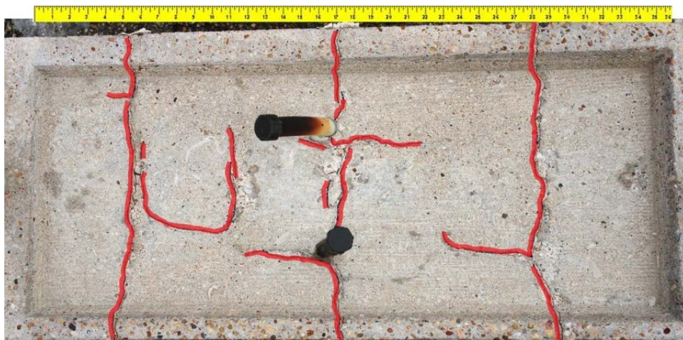
Figure 6.48: Specimen 2.3 Crack Map of Ponding Area
