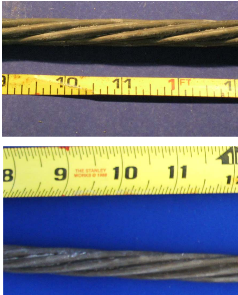
Figure 7.24: Typical Conventional Strand from 4 Year 2 (Top) and 6 Year (Bottom) Autopsy Periods
