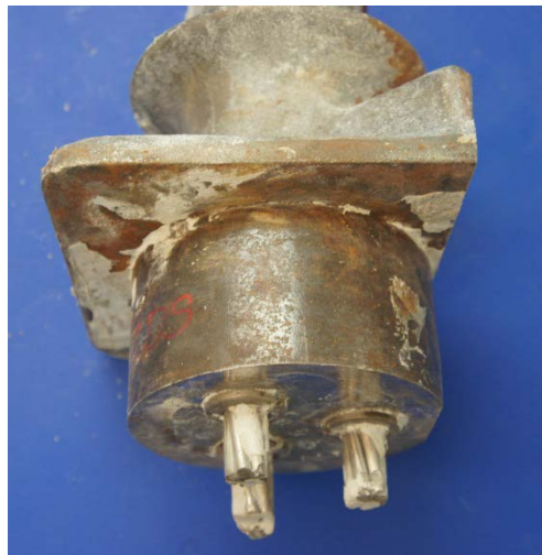
Figure 6.7: Damage from Saw of the South Dead End Anchorage of Specimen 5.2
