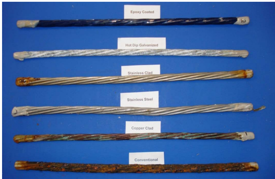
Figure 3.6: Appearance of Strands after Six Months of Exposure 13
