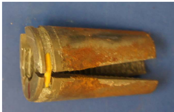
Figure 6.176: Moderate Corrosion on a Live End Wedge from Specimen 7.4
