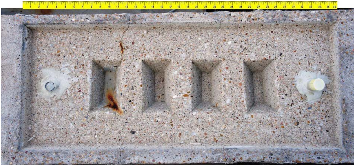
Figure 6.148: Specimen 7.3 Main Autopsy Region and Grout Vents
