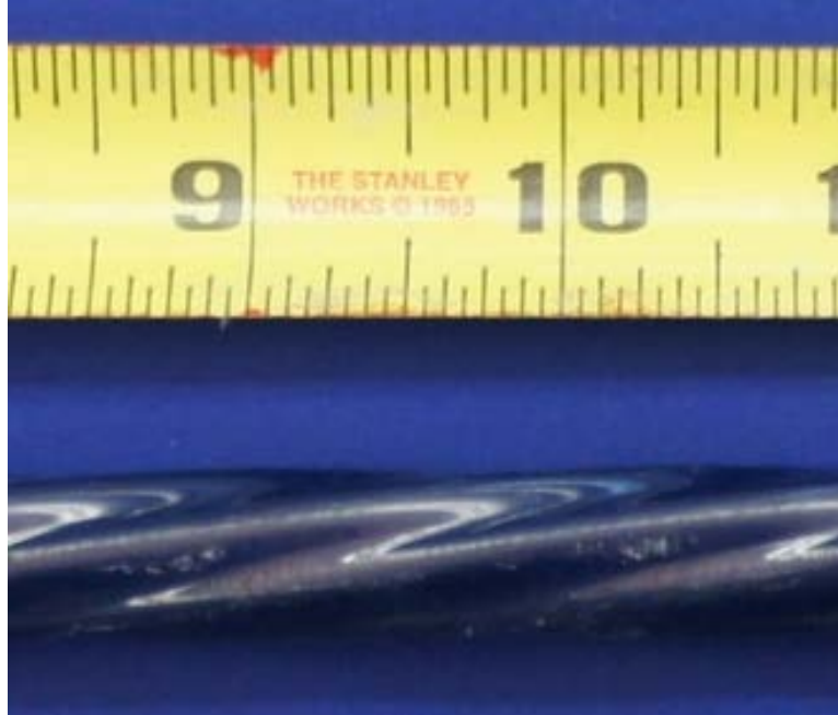
Figure 6.170: Scratches and Gouges in Epoxy Coating of a Strand from Specimen 7.4
