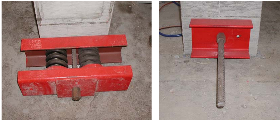
Figure 2.13: Dywidag Assembly, Dead End (Left) and Live End (Right) 1
