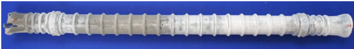
Figure 6.169: Variation of Color on the Bottom of the Grout from Specimen 7.4
