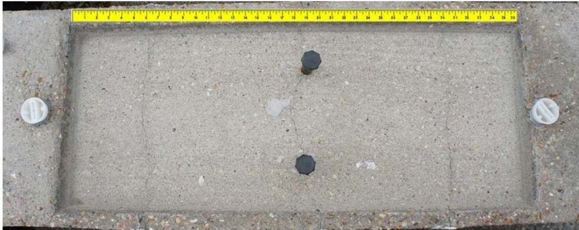
Figure 6.11: Specimen 1.1 Main Autopsy Region and Grout Vents
