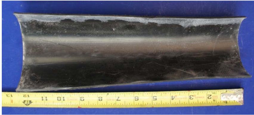
Figure 6.144: Light Scratches on the bottom of the Live End Duct Section of Specimen 7.2
