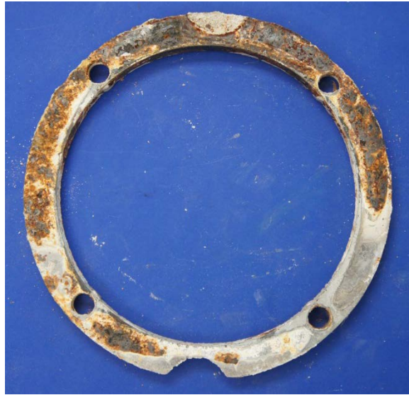
Figure 6.160: Pitting on Live End Steel Retaining Ring from Specimen 7.3
