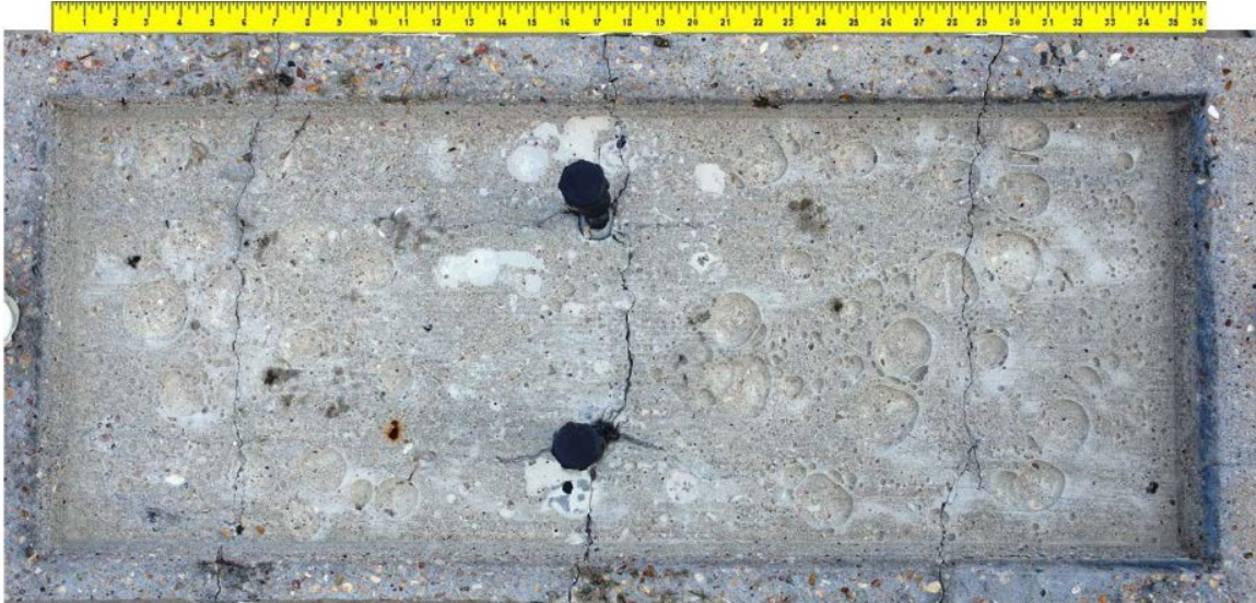
Figure 6.58: Specimen 3.3 Main Autopsy Region and Grout Vents
