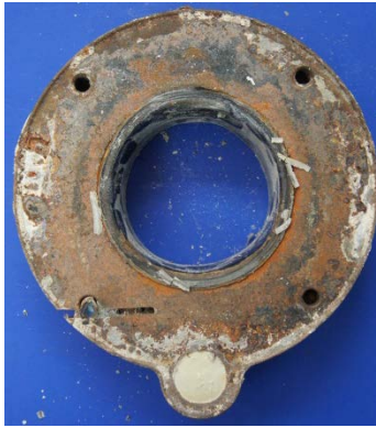
Figure 6.143: Exposed Surface of Dead End Anchorage Plate from Specimen 7.2
