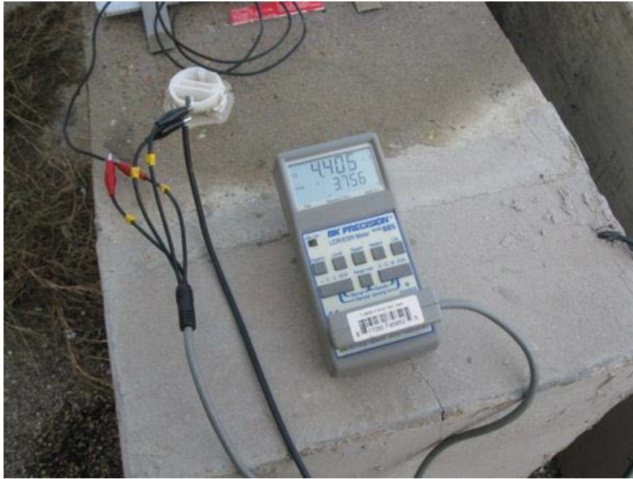
Figure 4.6: BK Model 885/886 LCR Meter Connected to Specimen 2
