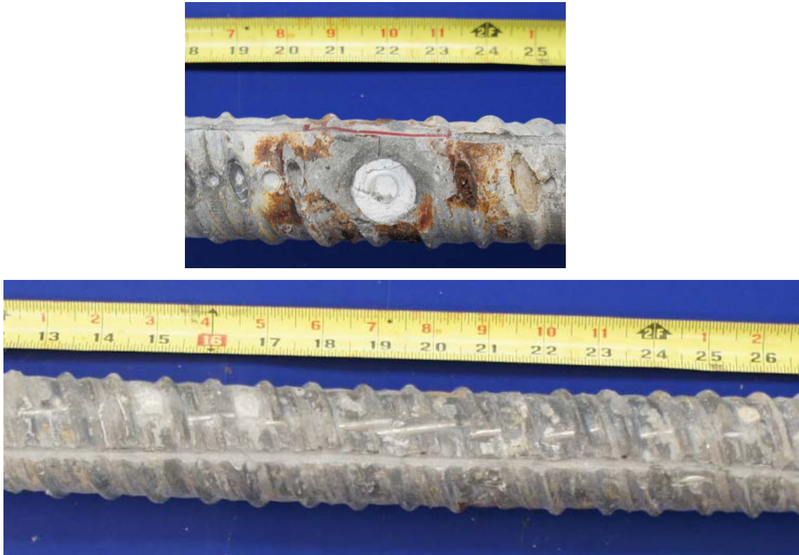
Figure 6.30: Staining on Grout from North Tendon (Top) and Exposed Strands on the Bottom of South Duct (Bottom) of Specimen 1.3
