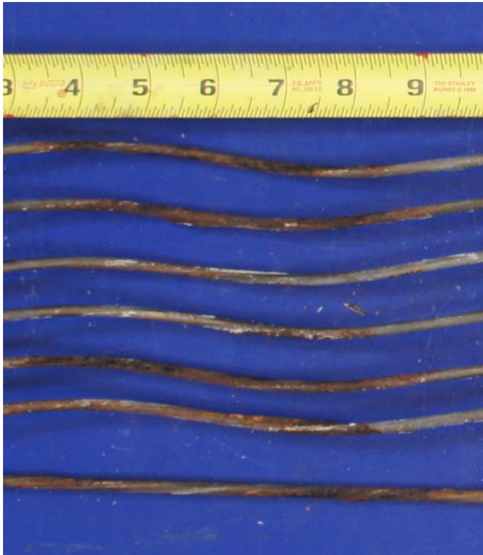
Figure 6.136: Pitting at Dead End Grout Vent of Specimen 7.2
