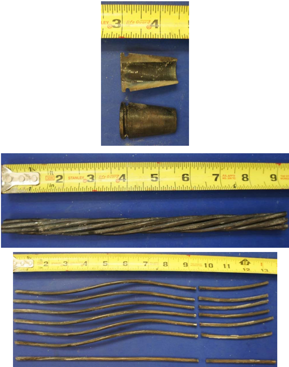
Figure 6.23: Typical Wedge (Top), Strand (Middle), and Unraveled Strand (Bottom) for the Dead End Anchorage Region of Specimen 1.1
