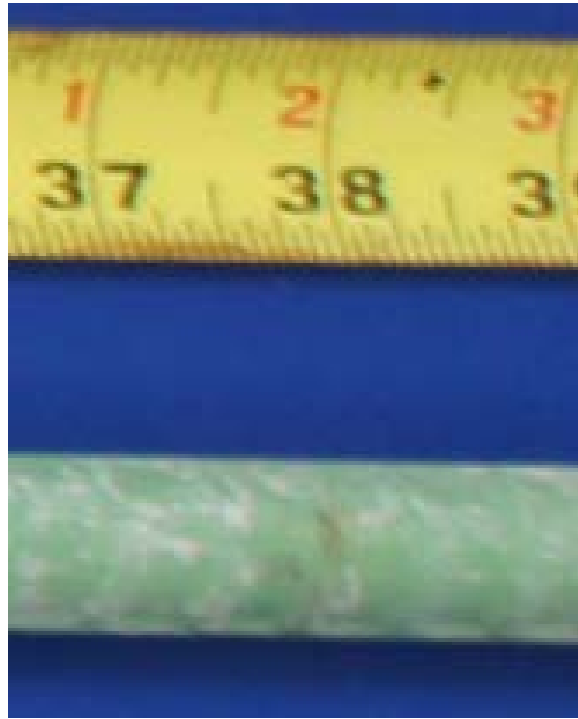
Figure 6.99: Rust Stain on North Longitudinal Bar from Specimen 5.1
