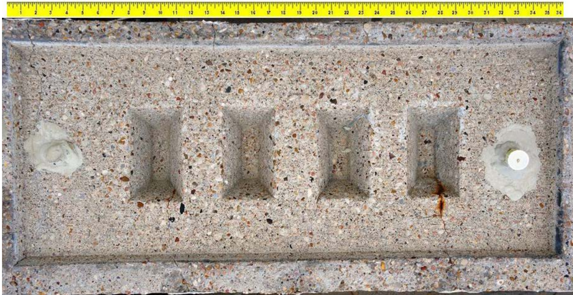
Figure 6.163: Specimen 7.4 Main Autopsy Region and Grout Vents
