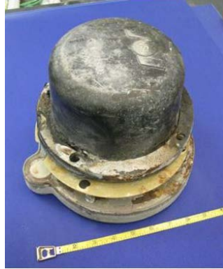
Figure 6.138: Anchorage Components, from Top: Grout Cap, Steel Retaining Ring, Insulation Plate, and Anchorage Plate 2
