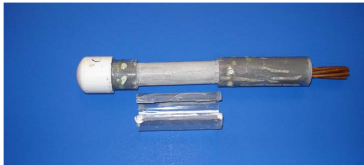
Figure 3.2: Cracked Active Corrosion Test Specimen 4
