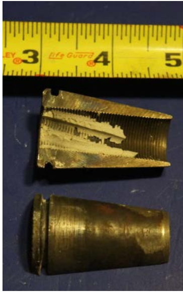
Figure 6.34: Light Surface Corrosion on Wedge from Specimen 1.3
