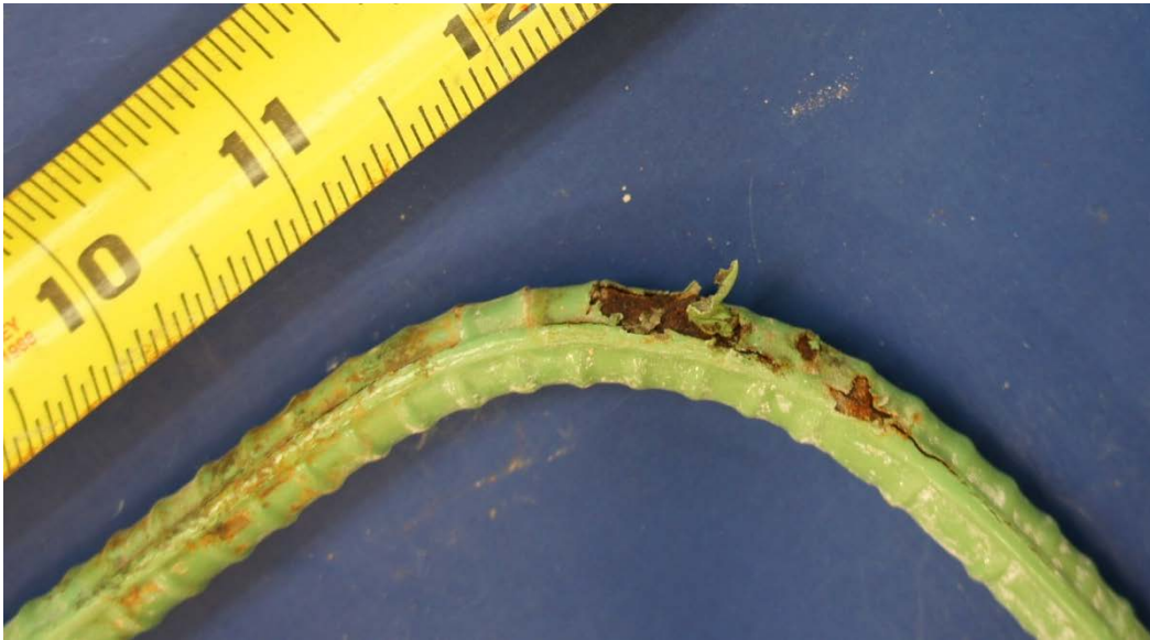
Figure 6.119: Moderate Corrosion at South Side Corner of Transverse Bar #4 from Specimen 5.3
