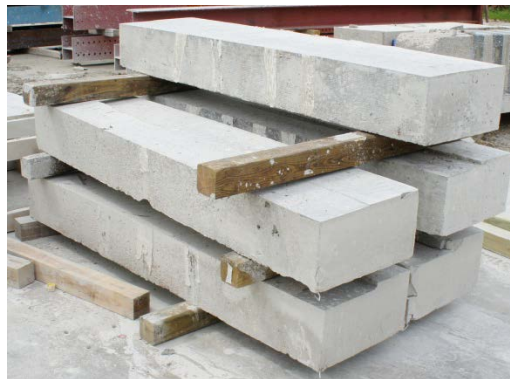
Figure 6.4: Stacked Specimen Blocks Awaiting Removal of Mild Reinforcement and Post-Tensioning Components
