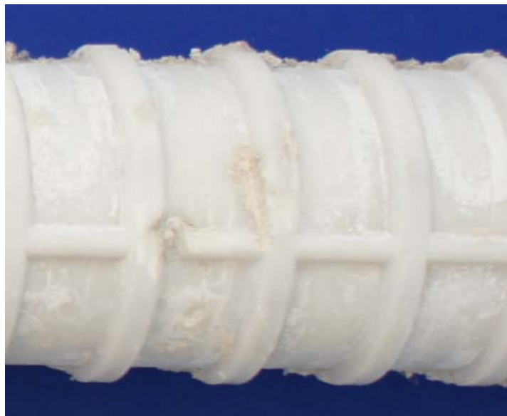
Figure 6.110: Chalky White Residue on North Duct of Specimen 5.2
