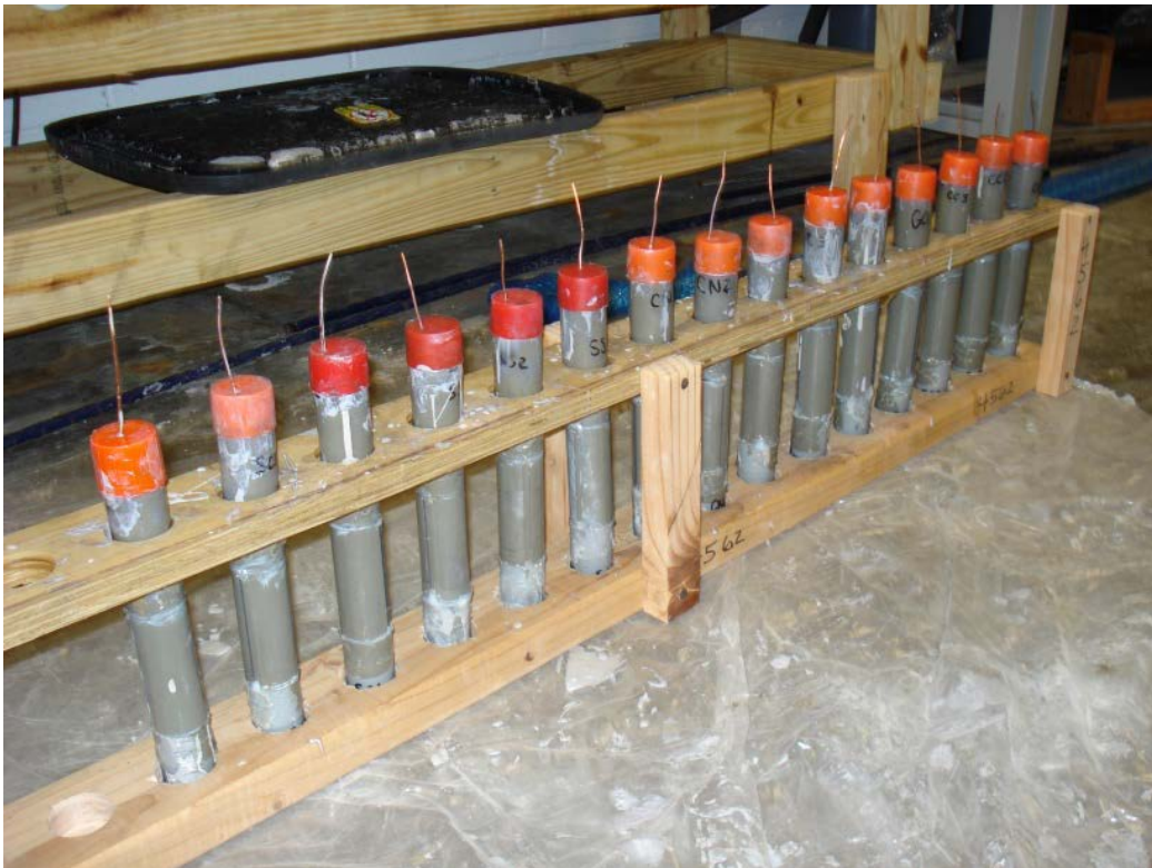
Figure 3.7: Completed Specimens for Passive Corrosion Testing 13
