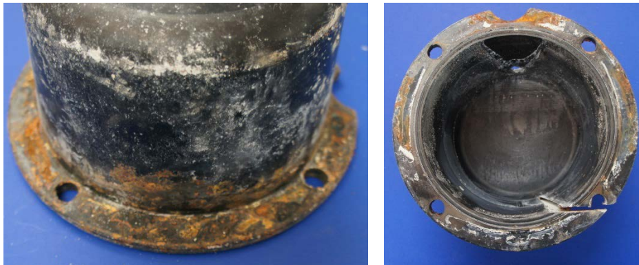
Figure 6.139: Rust Stains on Exposed (Left) and Unexposed (Right) Faces of Lip on the Dead End Rubber Cover from Specimen 7.2
