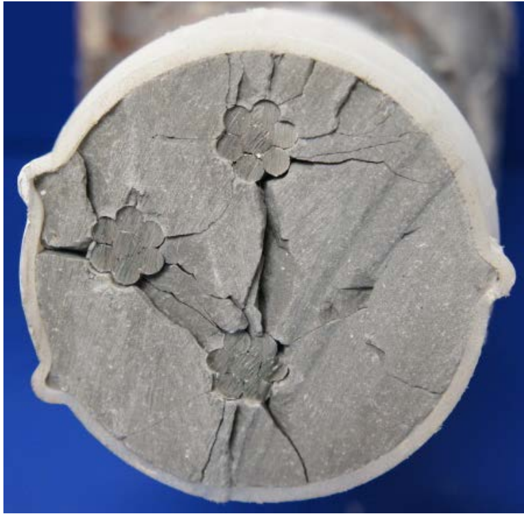
Figure 6.123: Retracted Strands from Specimen 5.3
