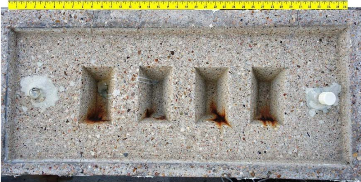
Figure 6.127: Specimen 7.2 Main Autopsy Region and Grout Vents
