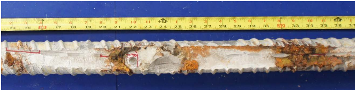
Figure 6.42: Large Void in Grout of South Tendon from Specimen 1.4
