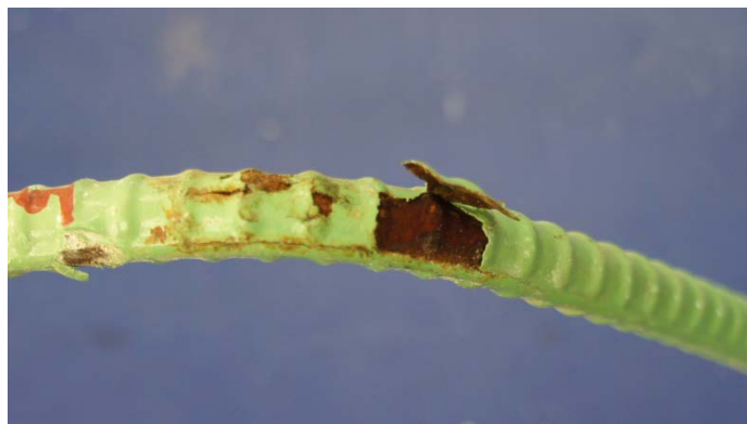
Figure 6.50: Moderate Corrosion on Transverse Bar #3 of Specimen 2.3
