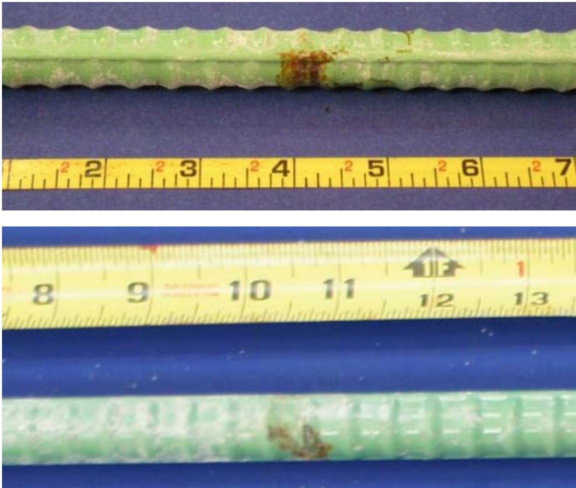
Figure 7.21: Typical Longitudinal Bar from 4 Year 2 (Top) and 6 Year (Bottom) Autopsy Period
