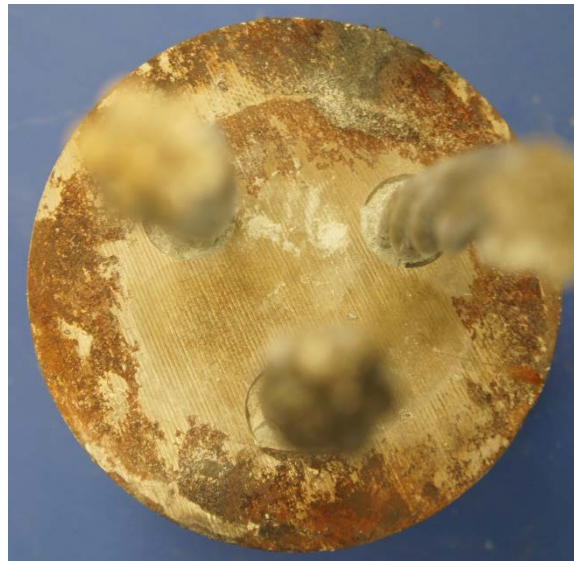
Figure 6.80: Corrosion on Unexposed Face of an Anchor Head from Specimen 4.1
