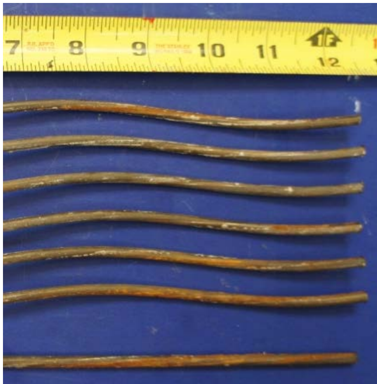
Figure 6.146: Pitting, Moderate, and Light Corrosion on Inner and Outer Wires from One Strand from the Dead End Section of the Tendon from Specimen 7.2
