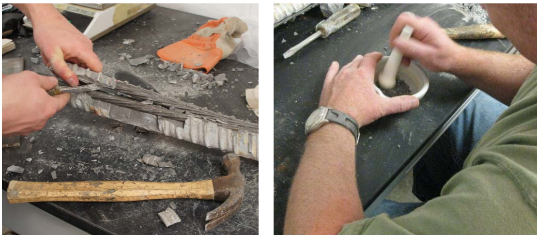
Figure 4.12: Grout Sample Extraction (Left) and Grinding Grout Sample 2 (Right)
