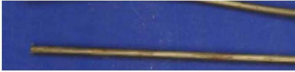
Figure 6.171: Mild Pitting and Moderate Corrosion on Inner Wire from a Specimen 7.4 Strand
