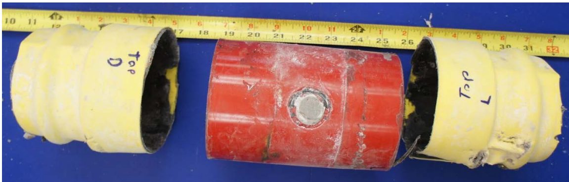
Figure 6.63: Coupler and Heat Shrink Wrap from North Duct of Specimen 3.3
