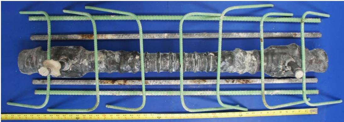
Figure 6.128: Layout of the Main Autopsy Region of 7-Series Specimens
