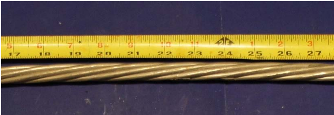
Figure 6.31: Typical Stainless Clad Strand from Specimen 1.3
