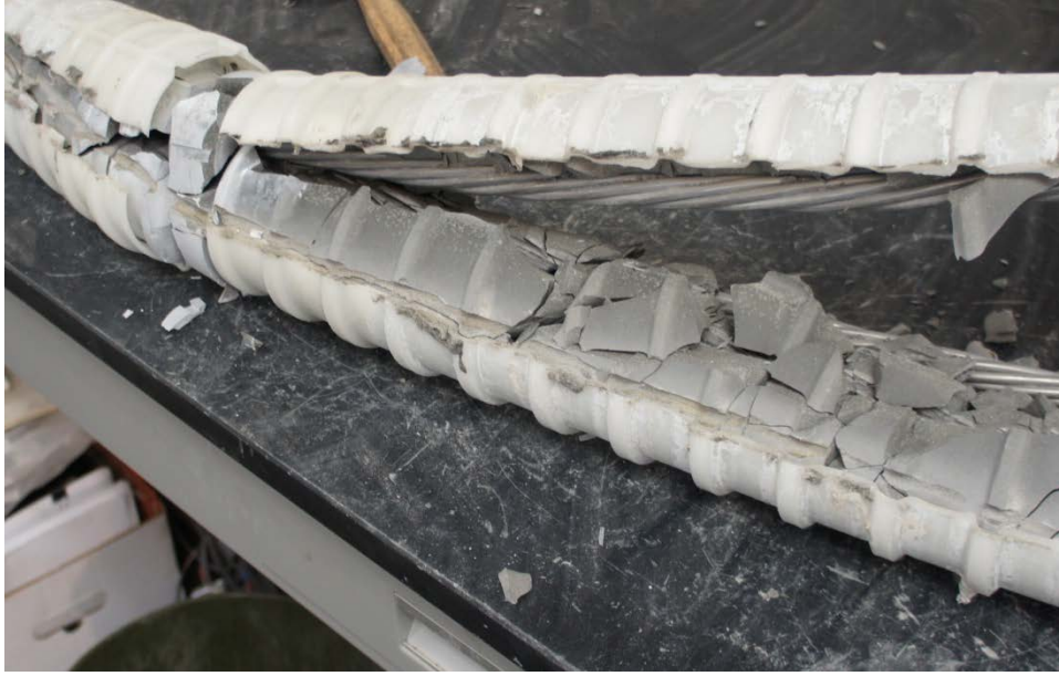
Figure 6.121: Grout Falling Apart from North Tendon of Specimen 5.3
