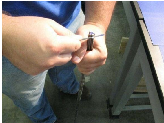
Figure 6.8: Separating Wires of the Strand Using a Screwdriver 2
