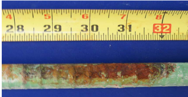
Figure 6.152: Pitting on Top of South Longitudinal Epoxy Coated Bar from Specimen 7.3
