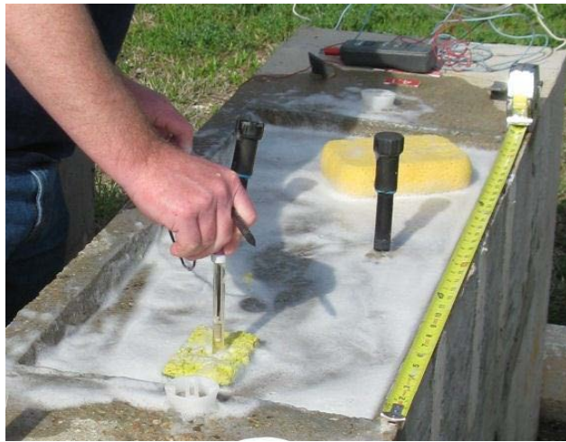
Figure 4.3: Taking Half-Cell Potential Readings 2
