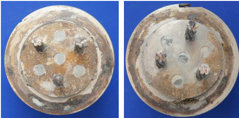
Figure 6.141: Unexposed Faces of Dead (Left) and Live (Right) End Anchor Heads from Specimen 7.2
