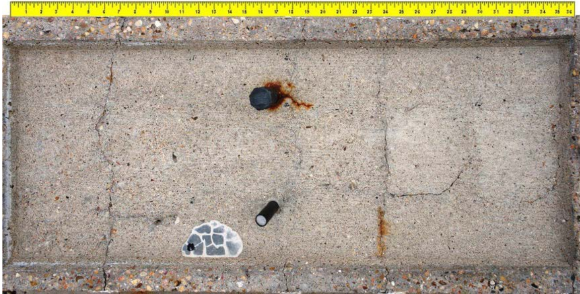
Figure 6.36: Specimen 1.4 Main Autopsy Region and Grout Vents
