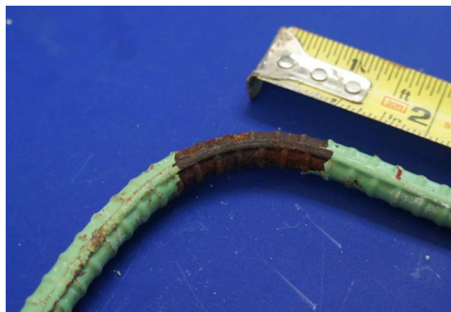
Figure 6.167: Pitting on Transvers Bar #1 from Specimen 7.4
