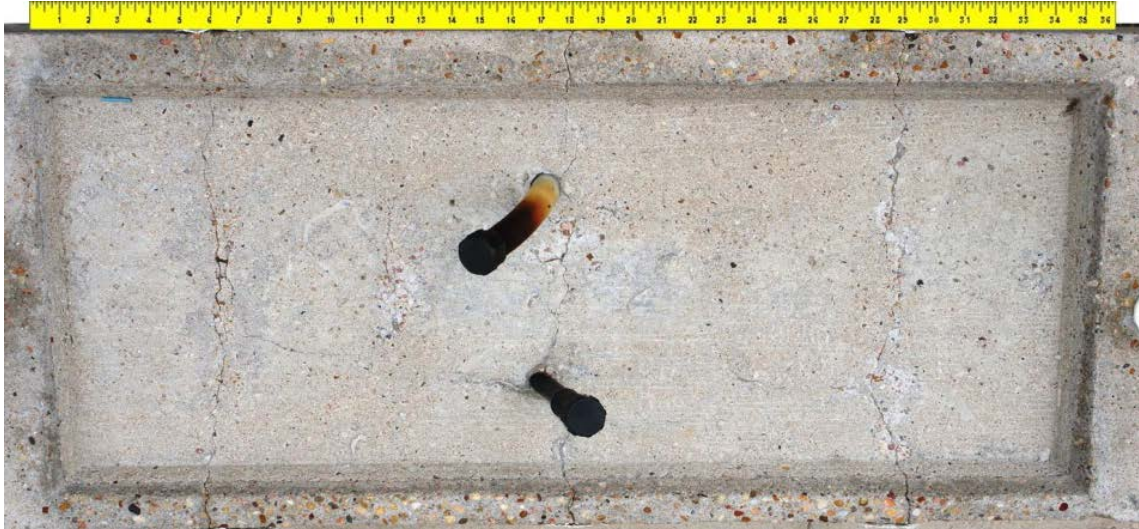
Figure 6.47: Specimen 2.3 Main Autopsy Region and Grout Vents
