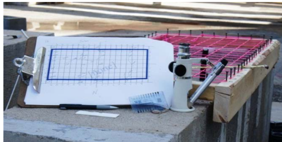
Figure 6.1: Crack Mapping and Crack Measuring Tools
