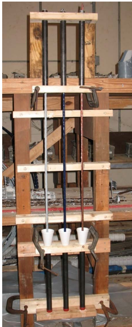
Figure 3.1: Adjustable Casting Jig 13
