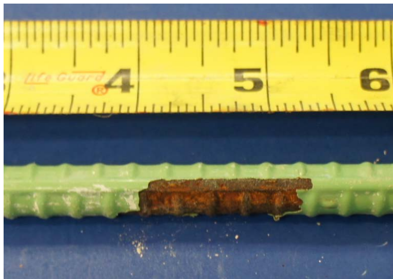
Figure 6.109: Moderate Corrosion on Transverse Bar #6 from Specimen 5.2
