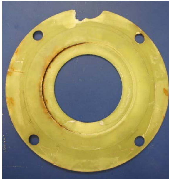
Figure 6.175: Split in Dead End Insulation Plate from Specimen 7.4
