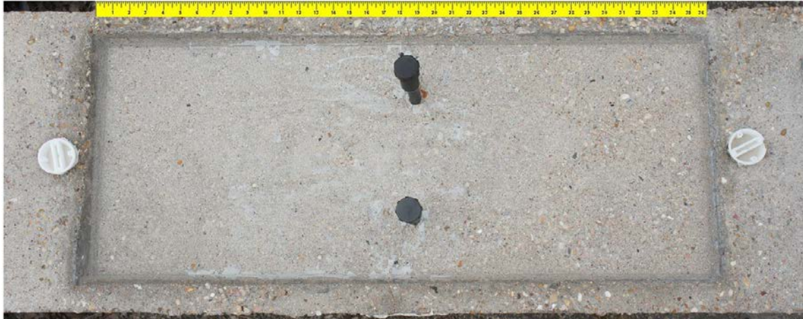
Figure 6.25: Specimen 1.3 Main Autopsy Region and Grout Vents
