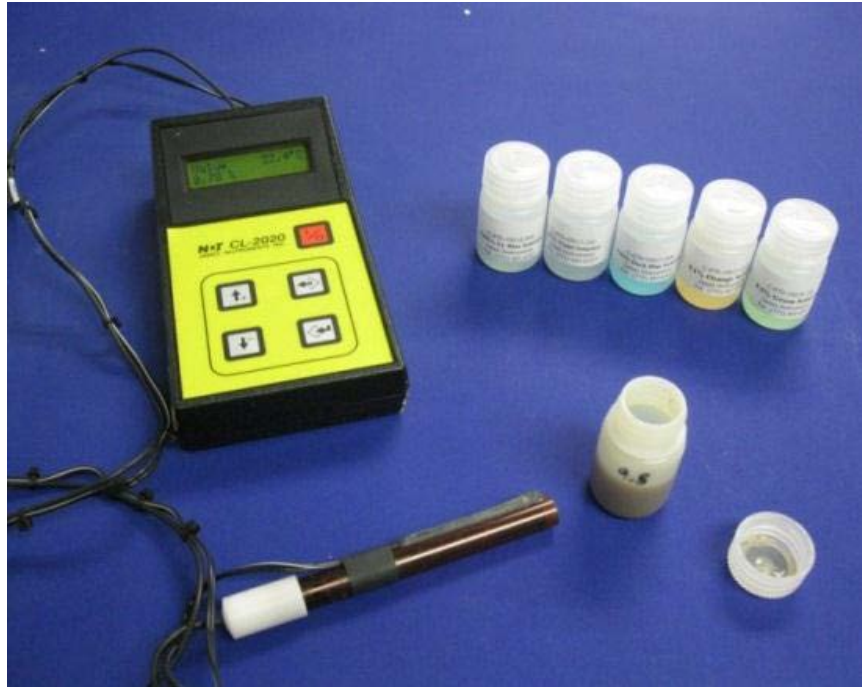
Figure 4.7: Chloride Content Measurement Setup 2
