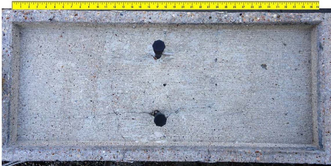
Figure 6.116: Specimen 5.3 Main Autopsy Region and Grout Vents
