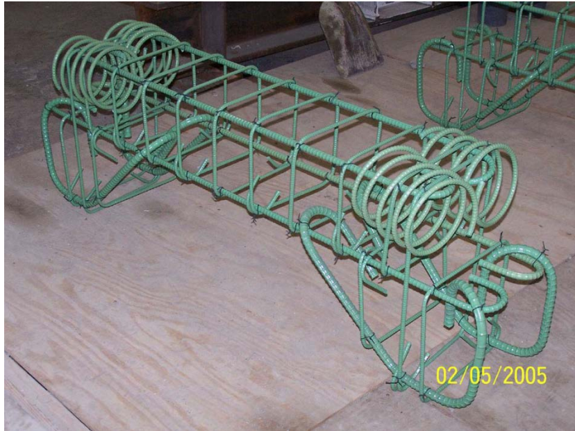
Figure 2.8: Passive Reinforcement Cage 1
