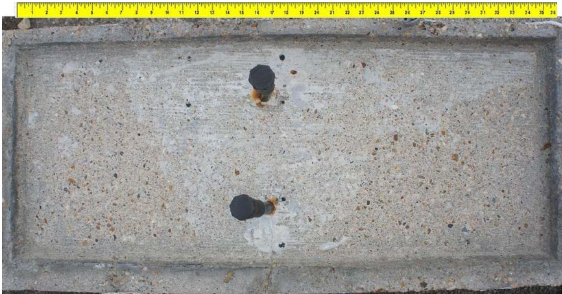
Figure 6.71: Specimen 4.1 Main Autopsy Region and Grout Vents
