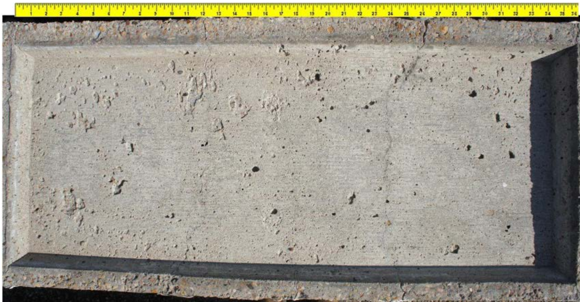
Figure 6.83: Specimen 4.3 Main Autopsy Region and Grout Vents
