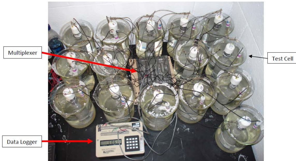
Figure 3.8: Completed Passive Corrosion Test Set-up 4
