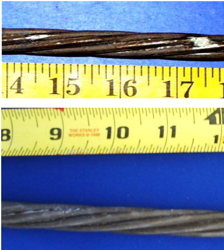
Figure 7.30: Typical Conventional Strand from Project 0-1405 5 (Top) and Project 0-4562 (Bottom)
