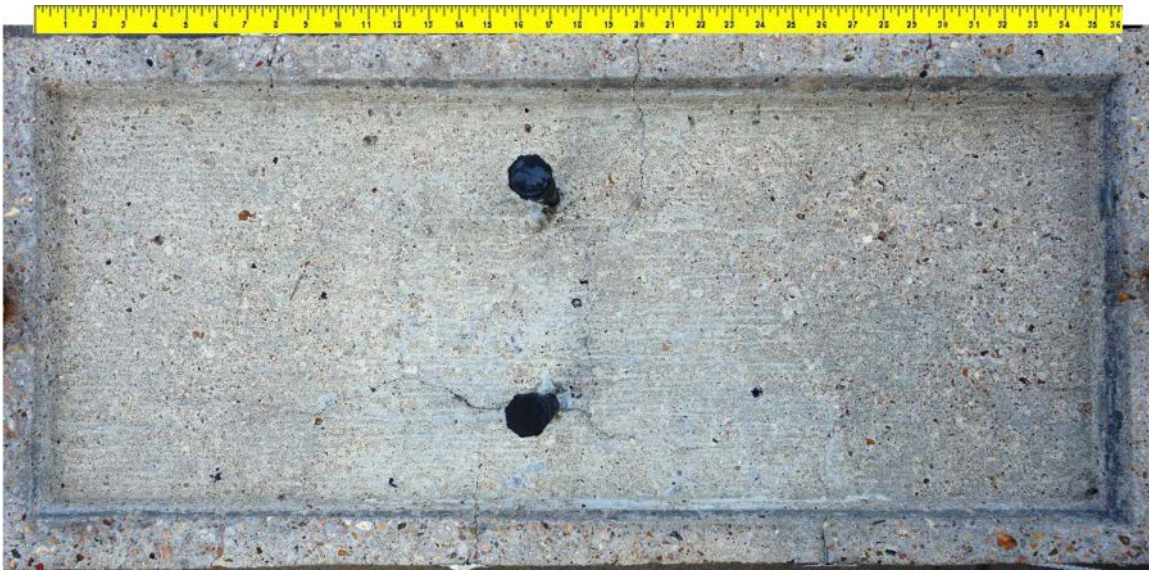
Figure 6.106: Specimen 5.2 Main Autopsy Region and Grout Vents
