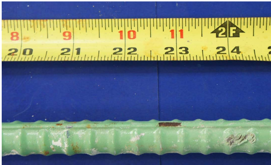
Figure 6.14: Extraction Damage, Rust Staining, and Moderate Corrosion of South Longitudinal Bar of Specimen 1.1
