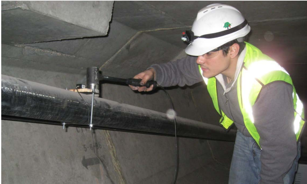
Figure 6.3: Vertical Vibration Test, US 183 Bridge
