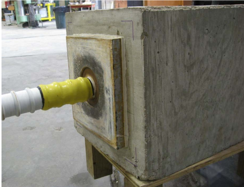
(a) Bearing Plate, Duct Exiting Anchor Block
