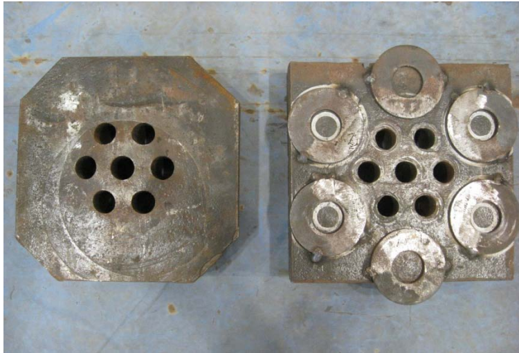
Figure 3.13: Steel Plates Used During Stressing
